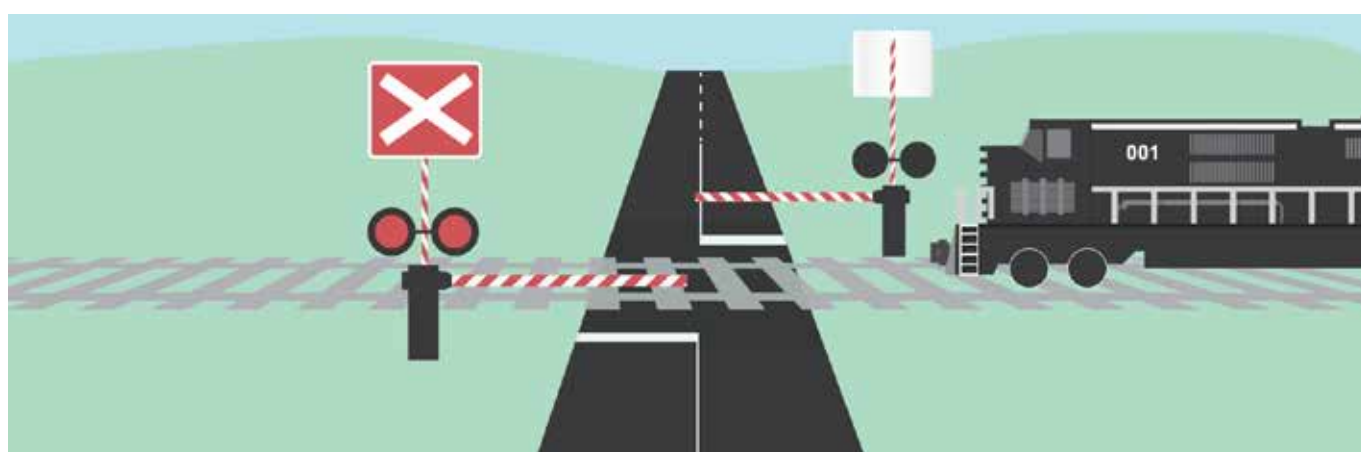
Level crossings can be either passive or active. This illustration shows an active crossing.
