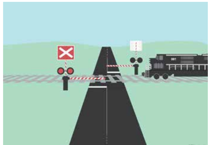
Example of level crossing. Level crossings can be either passive or active. This illustration shows an active crossing.
