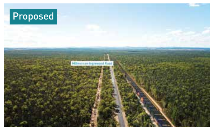
View of the project reference design, including proposed alignment and crossing loop, looking north towards Grays Road.
