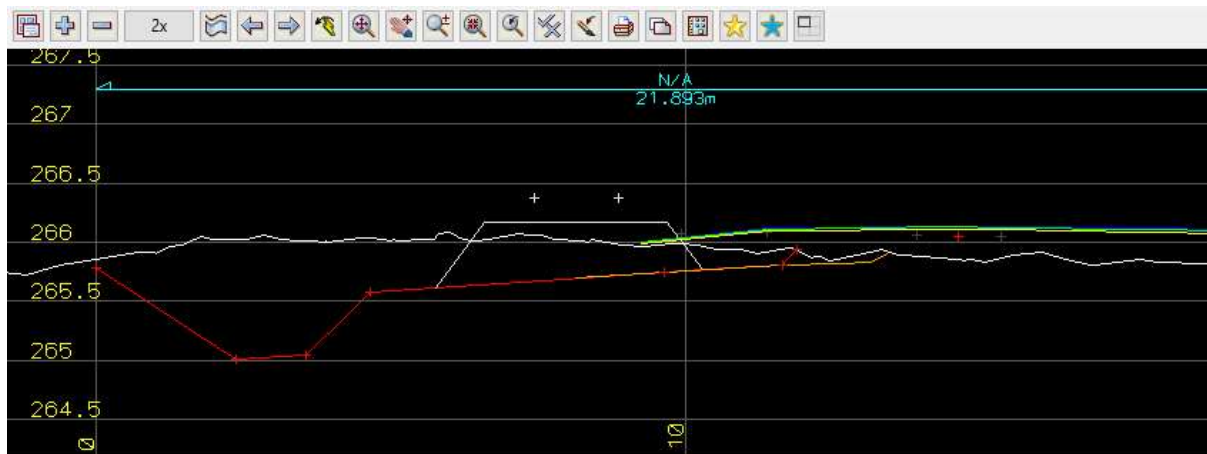
Figure 2.4 Non-conforming Cross-section at Ch498.165km
