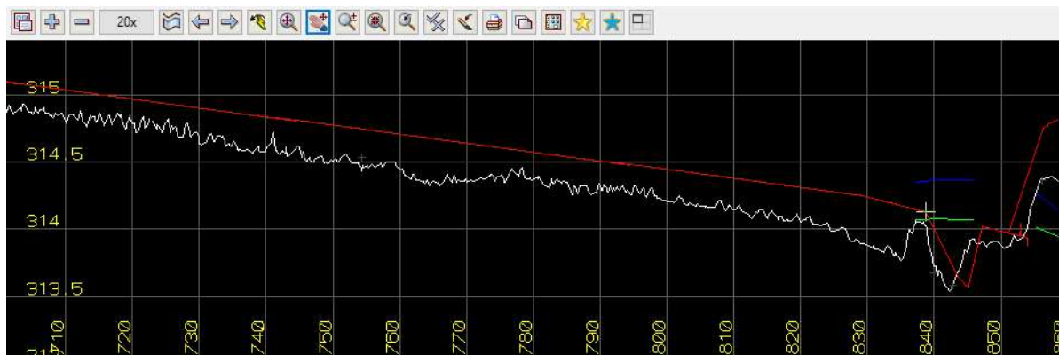
Figure 2.3 Non-conforming Long Section Profile Ch473.890km to Ch473.897km
