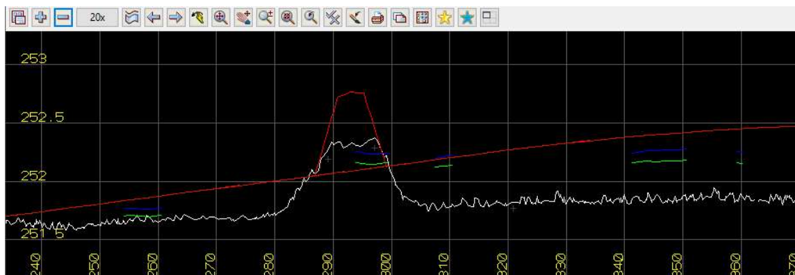
Figure 2.3 Non-conforming Long Section Profile Ch538.870km to Ch538.900km
