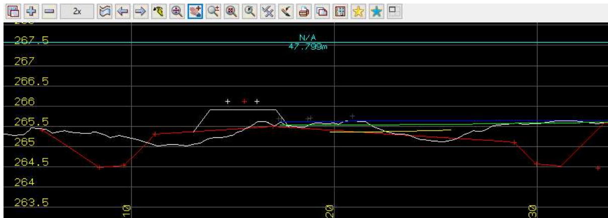
Figure 2.6 Non-conforming Cross-section at Ch498.590km
