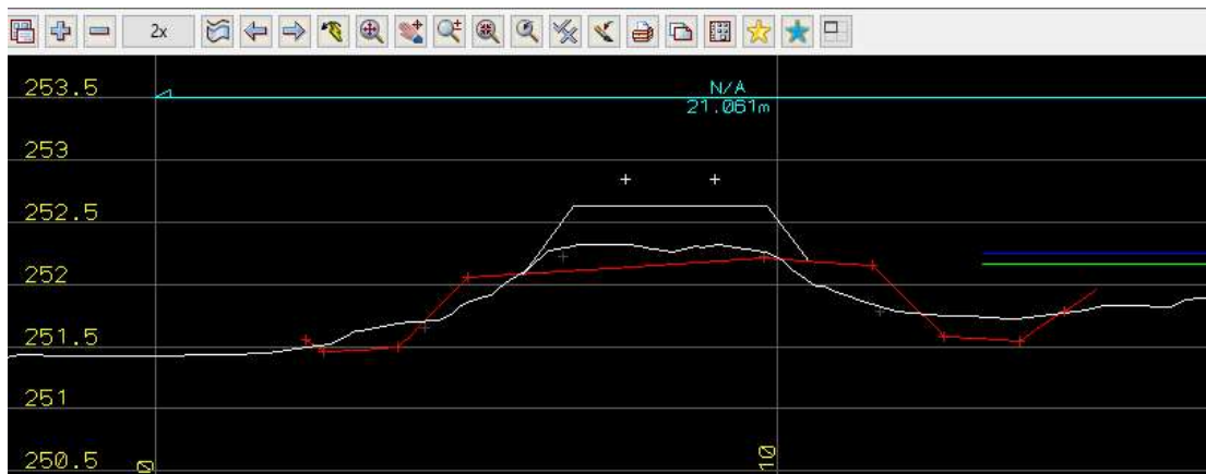
Figure 2.2 Non-conforming Cross-section at Ch538.875km
