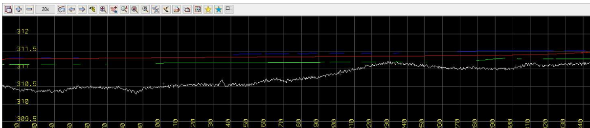
Figure 2.5 Non-conforming Long Section Profile Ch458.450km to Ch458.965km
