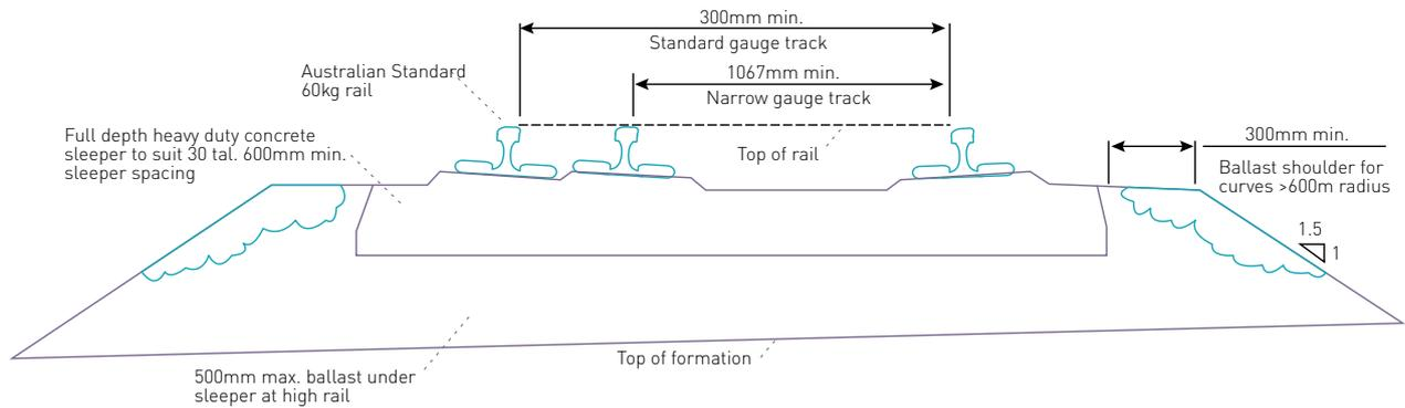
Typical dual-gauge ballasted track cross section
