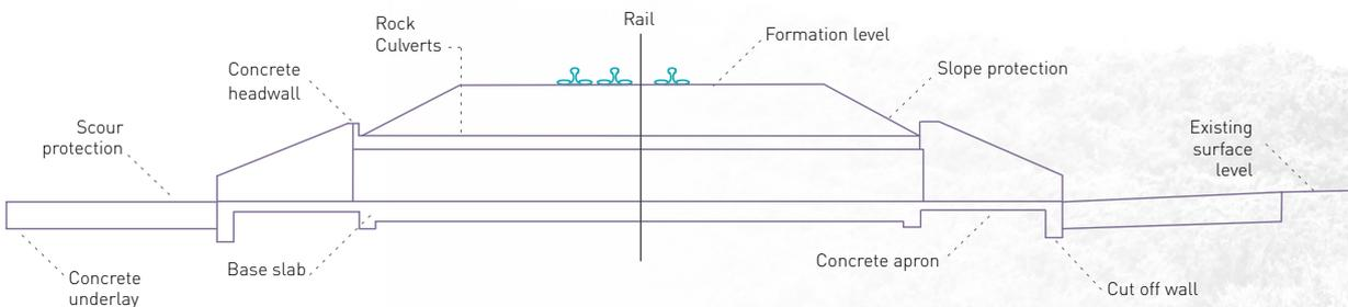
*Typical section of a cross drainage culvert*
