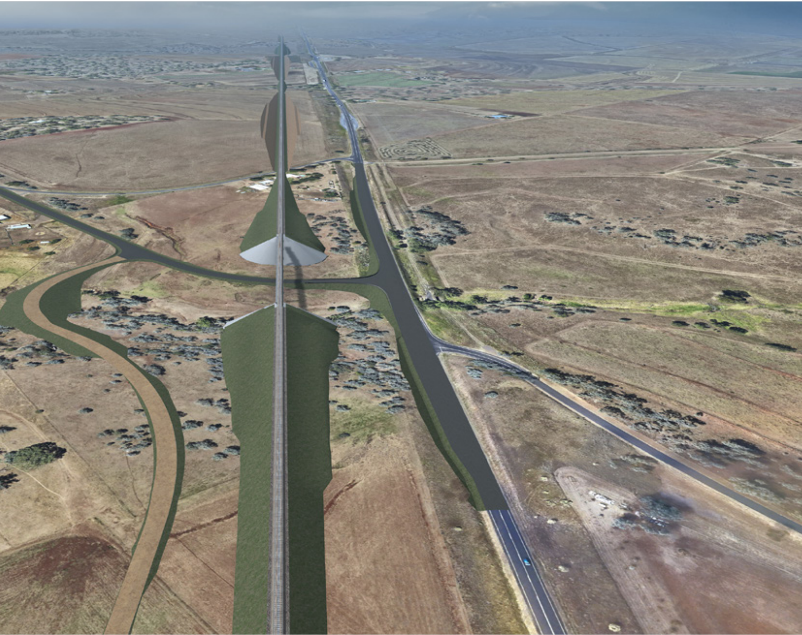
Proposed grade separation at Biddeston Southbrook Road and Bushy Lane diversion, Southbrook
