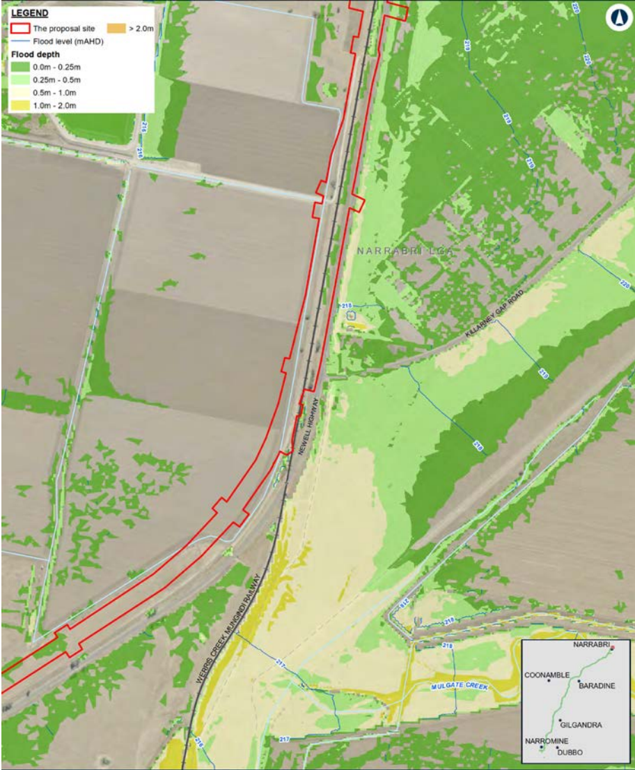
NARRABRI TO NARRABRI Existing peak depth / level (contour) - Detail - 1% AEP - Narrabri Appendix H - Figure 1.2a
