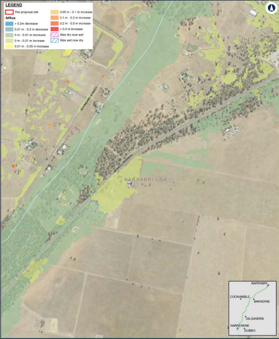
NARRABRI EXISTING FLOOD DEPTHS AND AFFLUX -1% AEP EVENT – SHEET J NARROMINE TO NARRABRI Change in peak flood level (afflux) - Detail - 1% AEP - Narrabri Appendix H - Figure 2.2)
