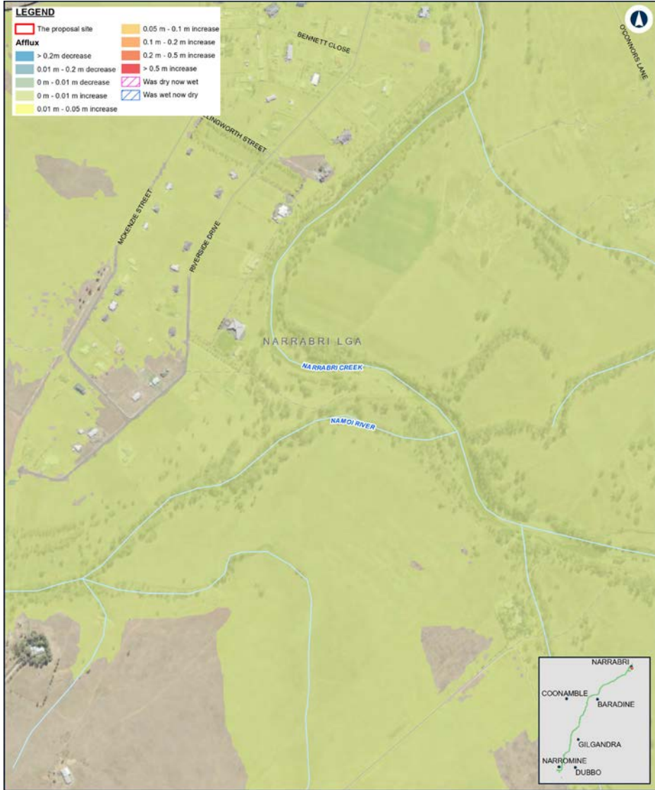
NARRABRI LGA Change in peak flood level (afflux) - Detail - 1% AEP - Narrabri Appendix H - Figure 2.21
