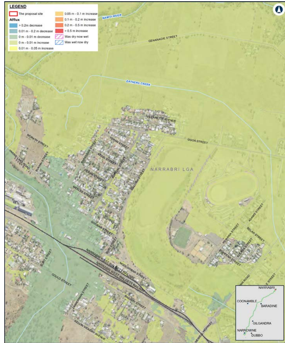
NARRABRI TO NARRABRI Change in peak flood level (afflux) - Detail - 1% AEP - Narrabri Appendix H - Figure 2.2g
