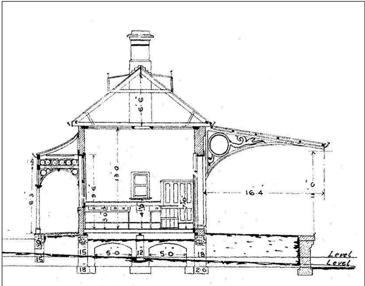
Figure 3-2: Original station plan: detail of the awning.
