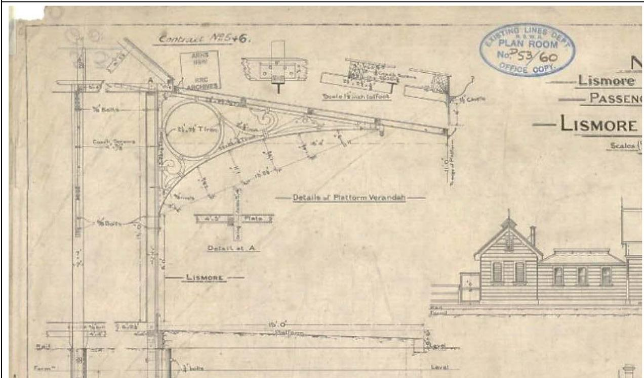
11. Plan of Lismore Station showing the awning overhanging the platform exactly as it does at Forbes Station. Lismore Station also appears to demonstrate the awning having been trimmed, as per the recent image in Photo 7 above.
