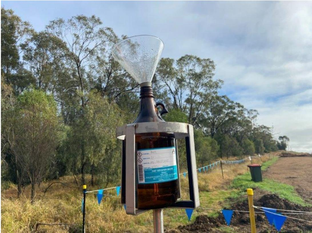
Plate 5 – PAD 6 Dust Deposition Gauge
