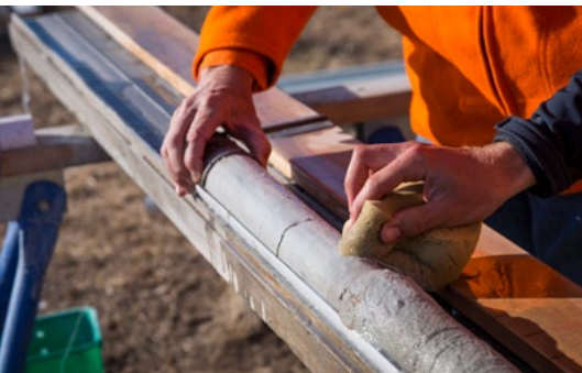
Cleaning a rock sample from a borehole to assess how fractured, weathered, and strong it is
