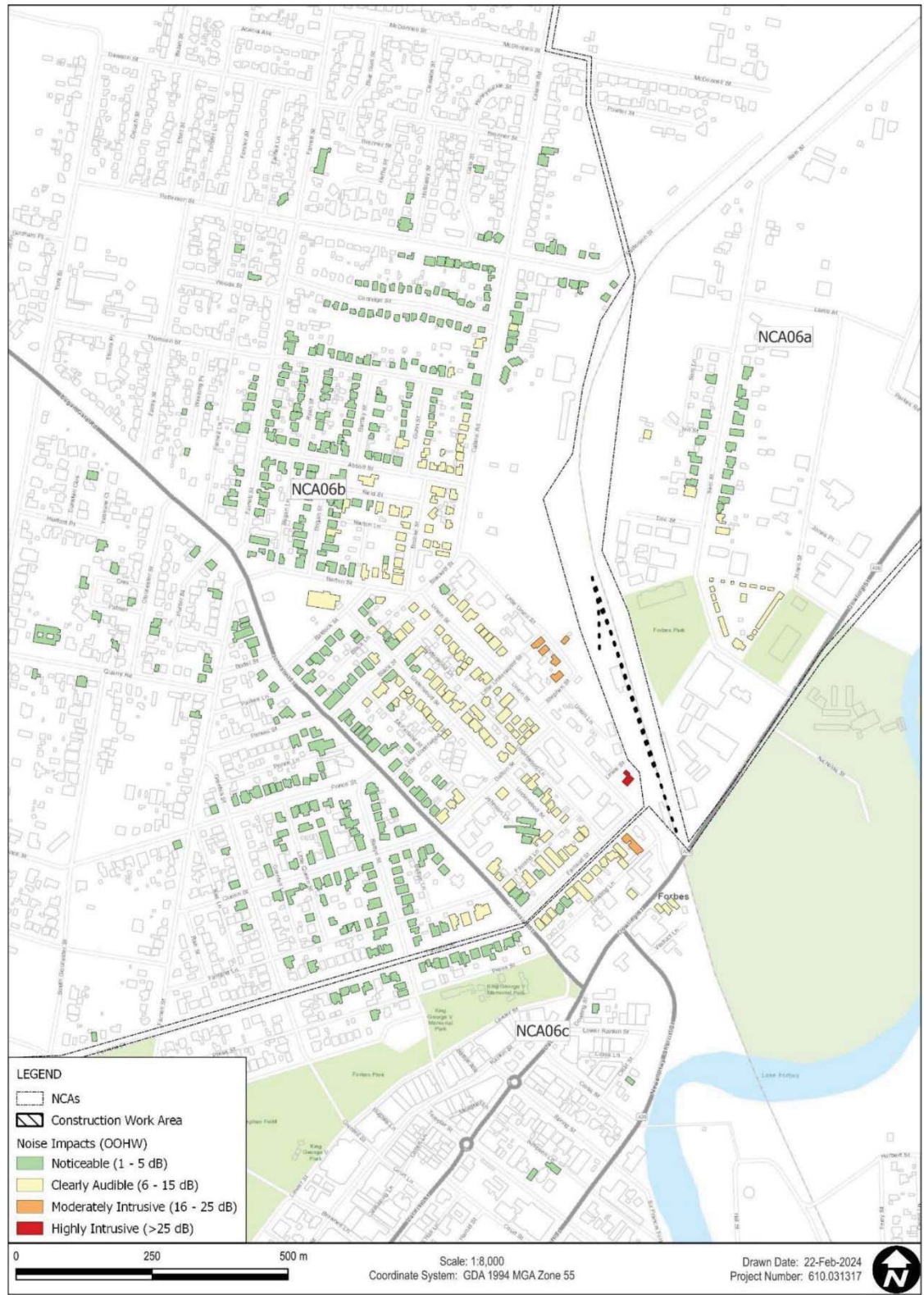
Figure C-11 W.003b: Trackwork w/o Rail saw – Daytime (OOHW)
