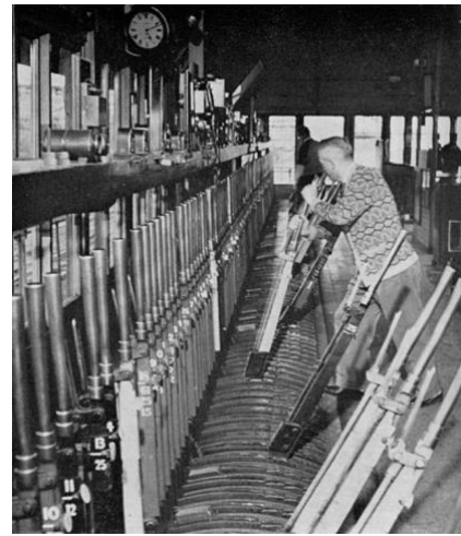
Figure 6: Staff manually operating signals by pulling the lever, as published in a 1958 Victorian Railways Newsletter . Source: Victorian Railways.
