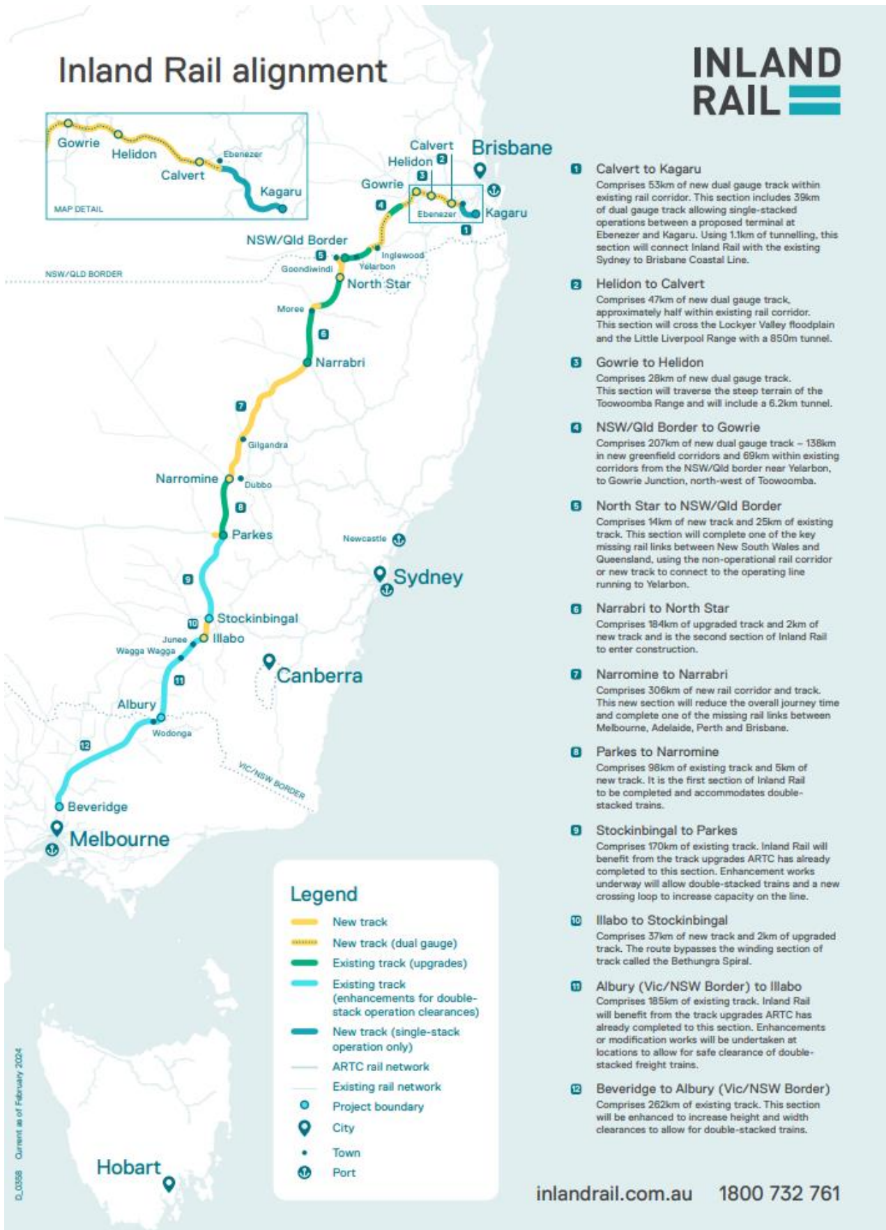
Figure 1: Beveridge to Kagaru projects
