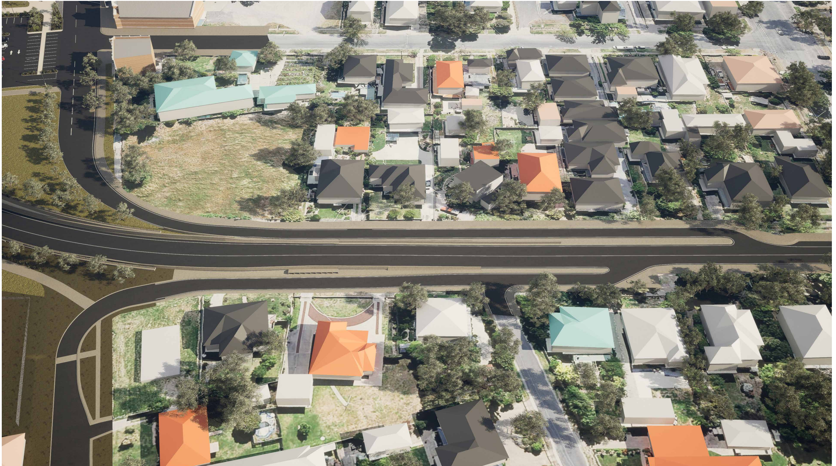
Figure 12 : Indicative artistic impression of slip lane extensions on both sides of Anderson Street.
