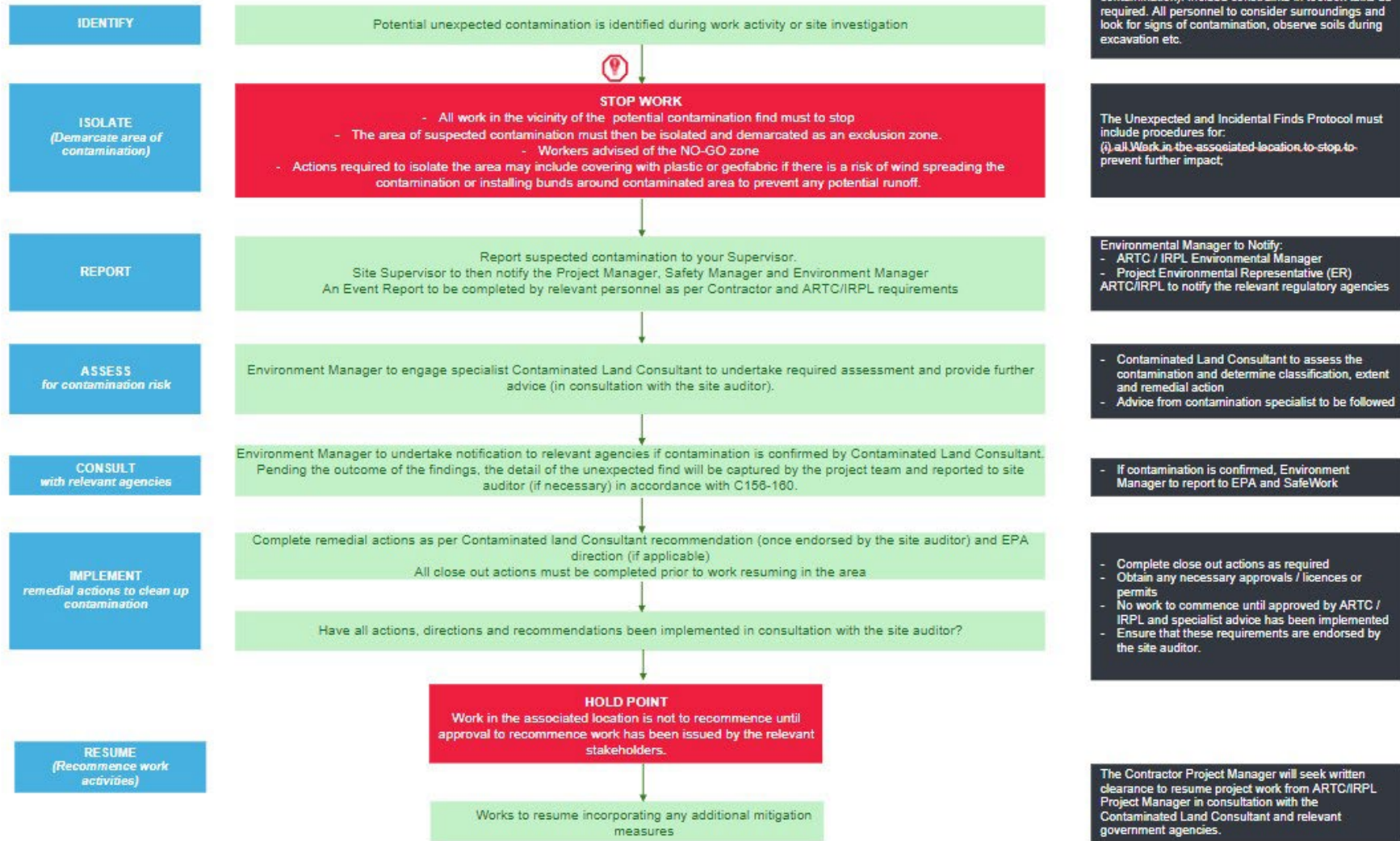
Figure C1: Unexpected Finds Procedure, Contaminated Land
