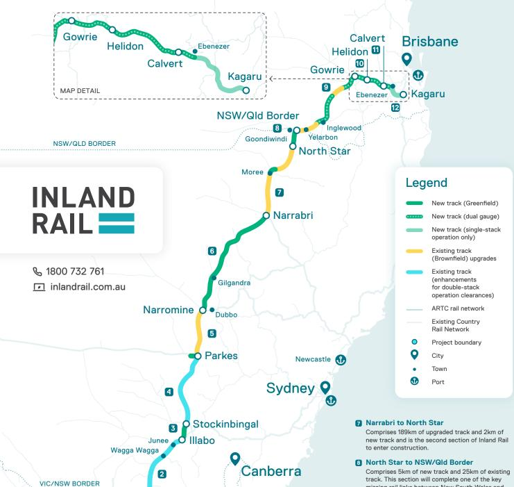
Comprises 5km of new track and 25km of existing track. This section will complete one of the key missing rail links between New South Wales and Queensland, using the non-operational rail corridor and new track to connect to the NSW/Qld Border to Gowrie section and the operating line running to Yelarbon.
