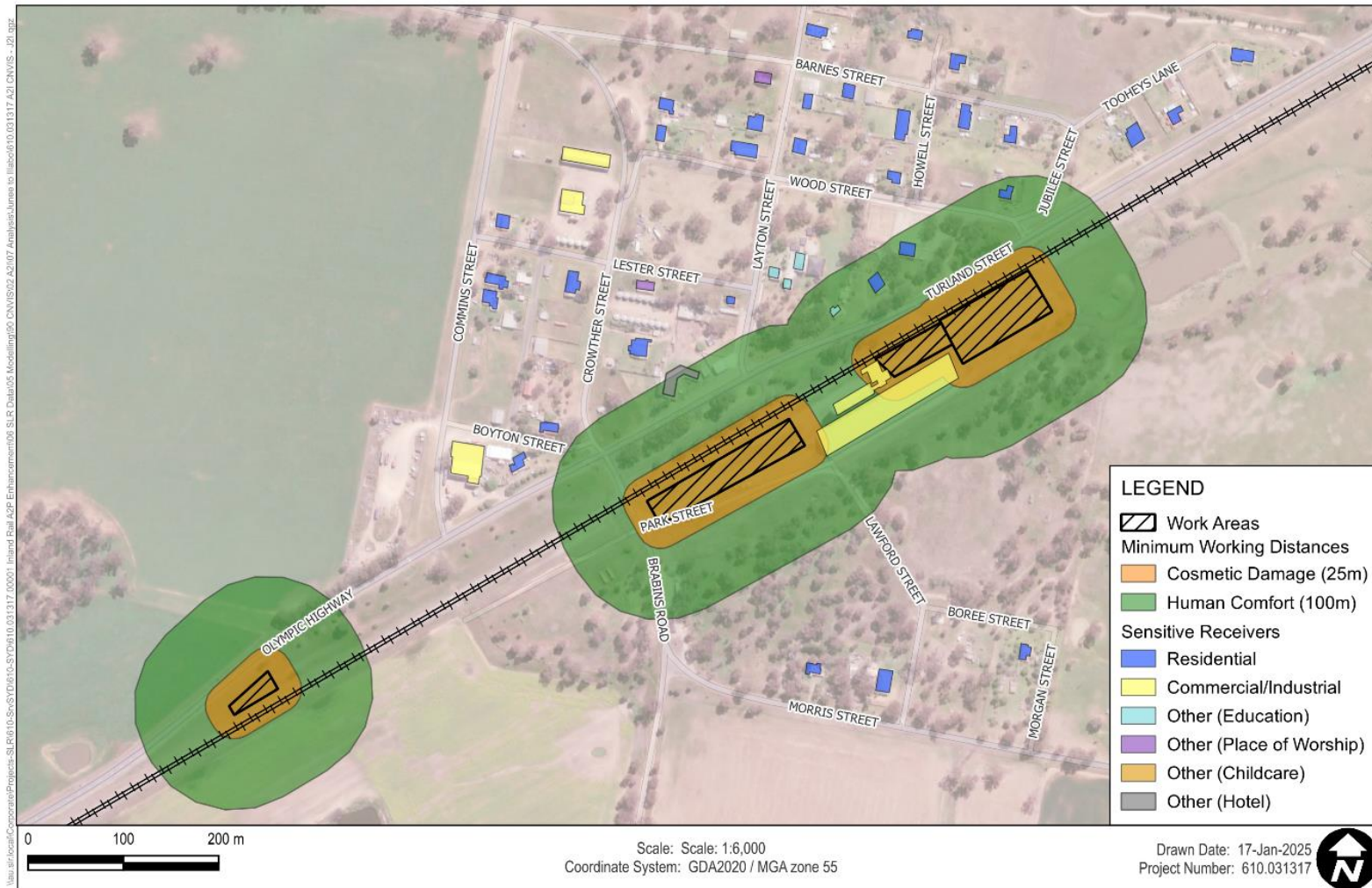
Figure 9 Vibratory Roller >300 kN -Minimum Working Distances (W.001 East)
