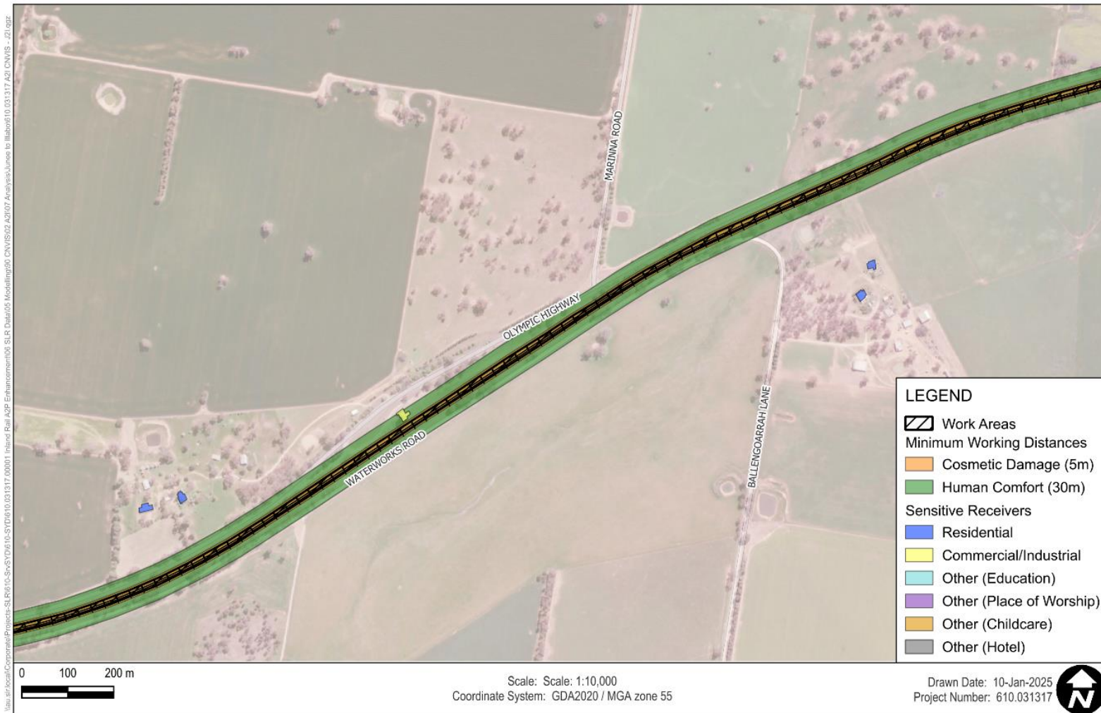
Figure 10 Ballast tamping - Minimum Working Distances W.005 (West)
