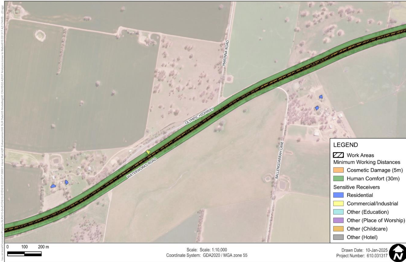
Figure 10 Ballast tamping - Minimum Working Distances W.005 (West)
