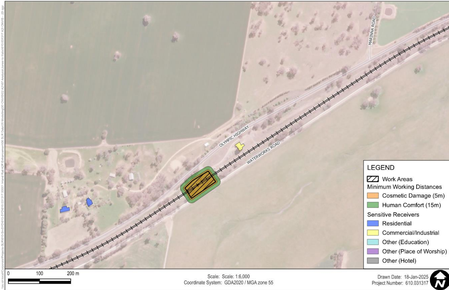
Figure 12 Vibratory Roller <50 kN -Minimum Working Distances (W.009 West)
