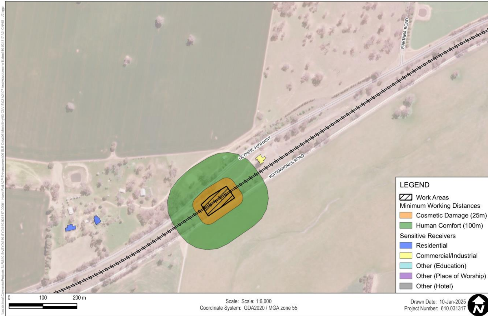
Figure 13 Vibratory Roller >300 kN -Minimum Working Distances (W.009 West)
