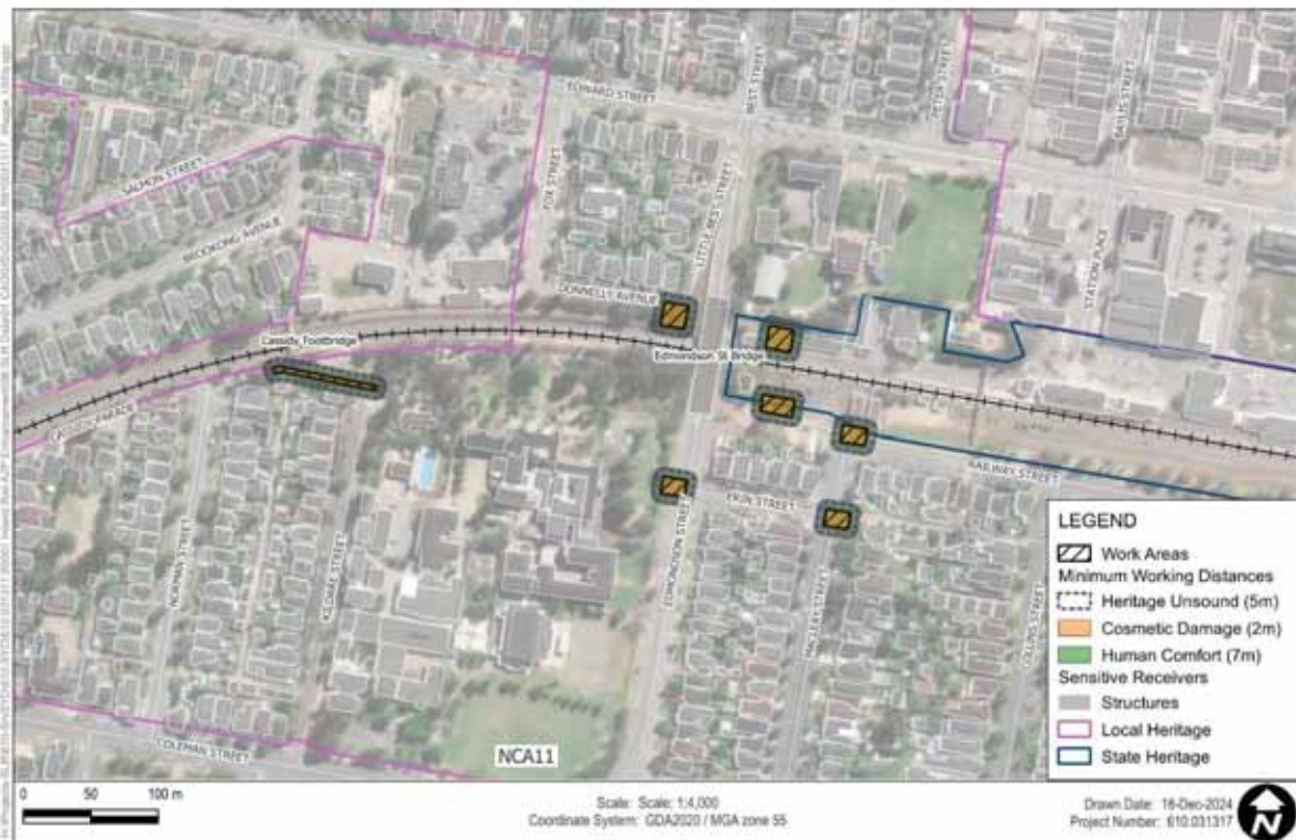
Figure 8 Small Hydraulic Hammer - Minimum Working Distances (Pearson Street)
