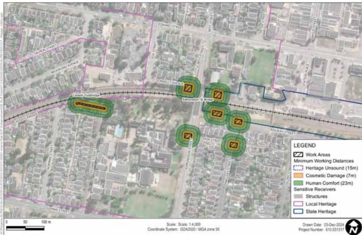
Figure 6 Medium Hydraulic Hammer - Minimum Working Distances (Pearson Street)
