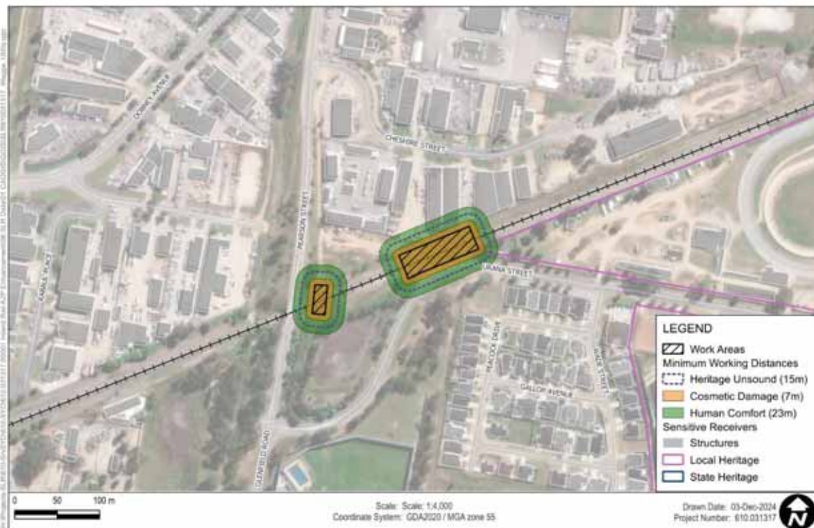
Figure 6 Medium Hydraulic Hammer - Minimum Working Distances (Pearson Street)
