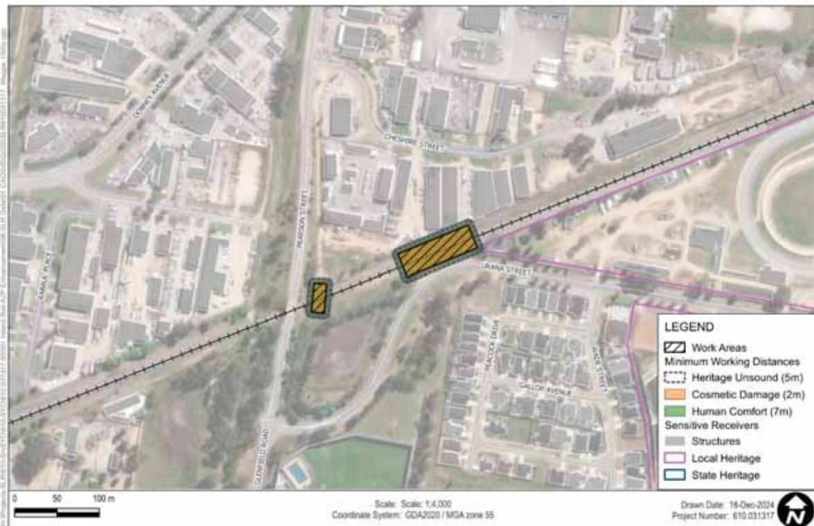
Figure 8 Small Hydraulic Hammer - Minimum Working Distances (Pearson Street)
