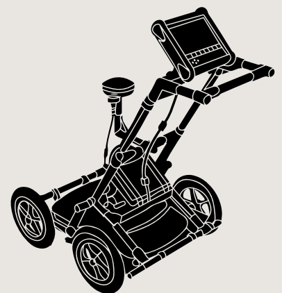
Illustration of a Ground Penetrating Radar.
