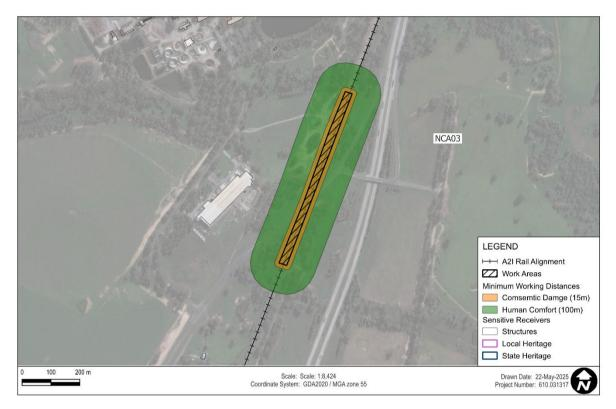
Figure 4 Construction Vibration Minium Working Distances – Vibratory Roller <300kN (7-13 tonne) (W.004)
