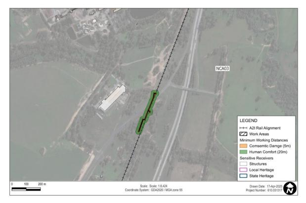
Figure 8 Construction Vibration Minium Working Distances – Large Hydraulic Hammer (W.010)
