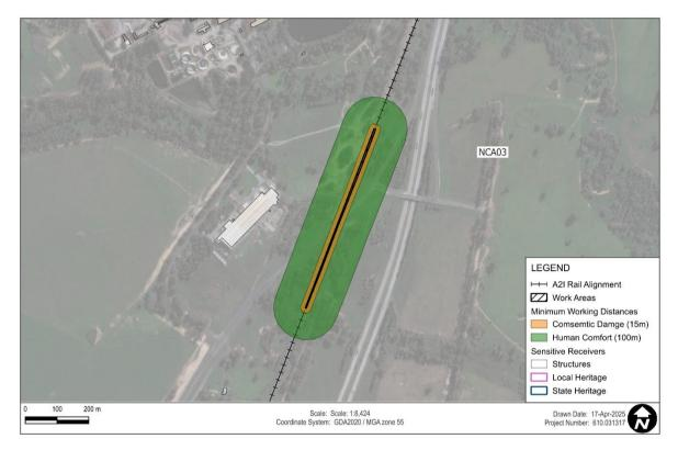
Figure 6 Construction Vibration Minium Working Distances – Ballast tamper (W.007)
