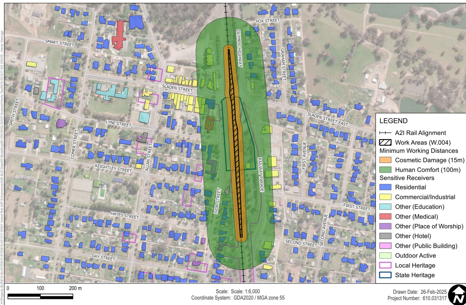
Figure 3 Vibratory Roller <300 kN – Minimum Working Distances (7-13 tonne) (W.004)
