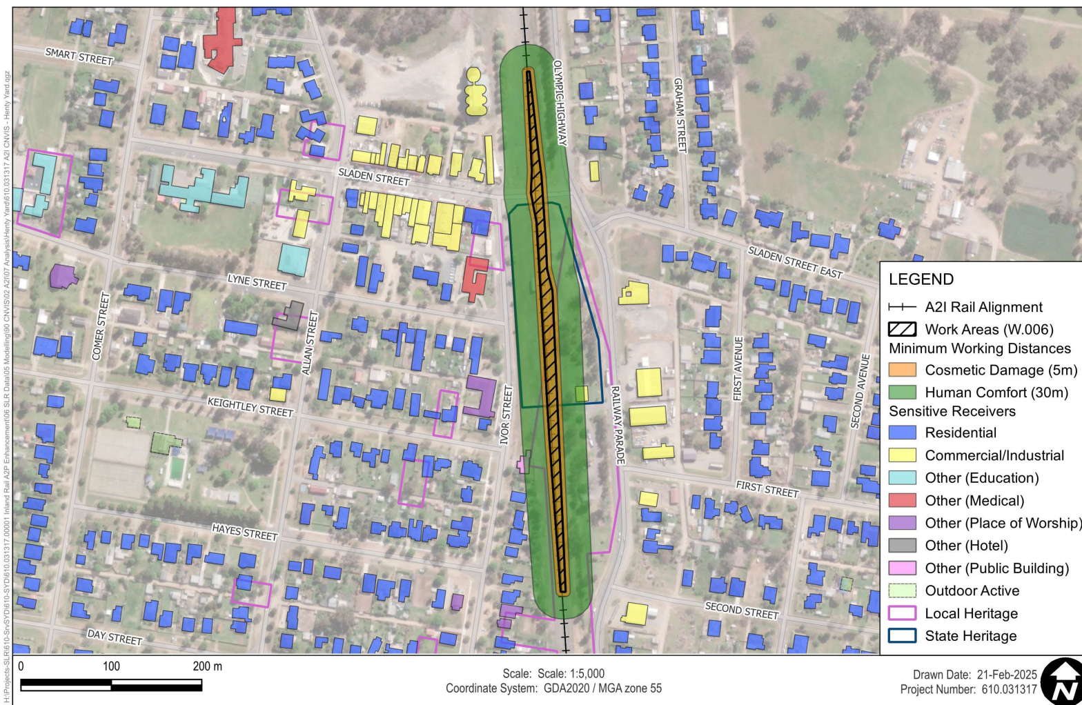
Figure 5 Track Tamping – Minimum Working Distances (W.006)
