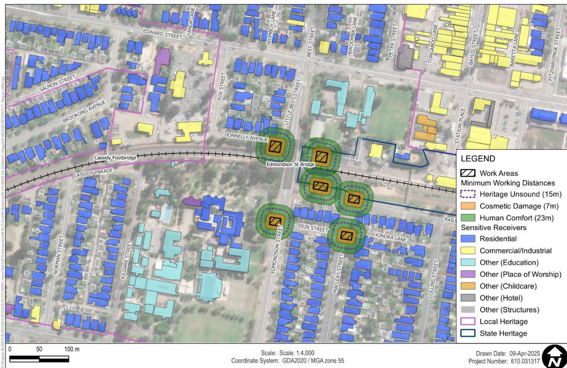
Figure 5 Medium Hydraulic Hammer - Minimum Working Distances (Edmondson Street)
