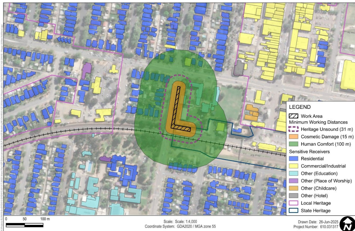
Figure 9 Vibratory Roller (7-13 T) - Minimum Working Distances (Edmondson Street)
