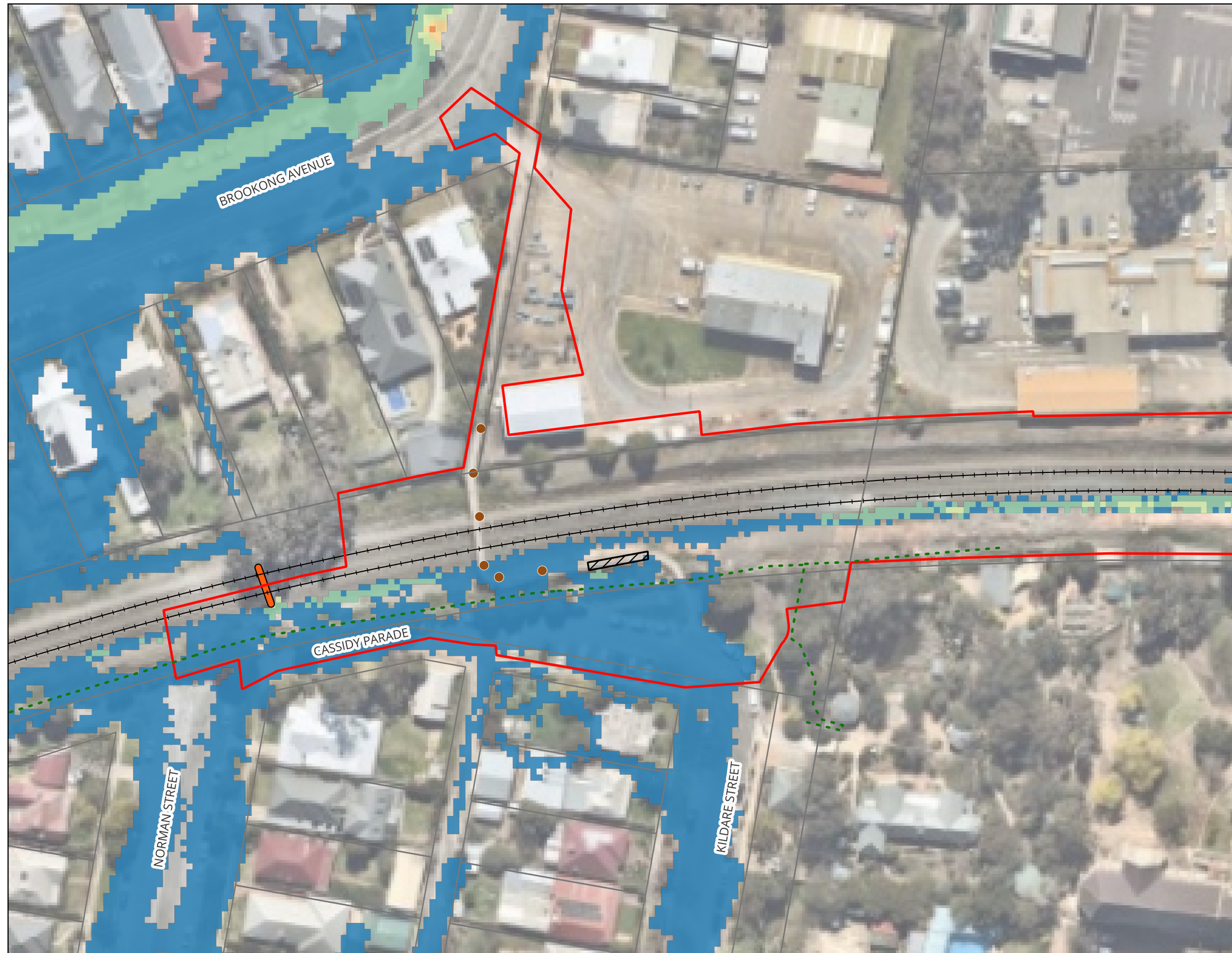
Cassidy Parade Footbridge - Inland Rail (A2P) - IFC Stage Figure A17 : 2% AEP Peak Flood Hazard - Existing Condition
