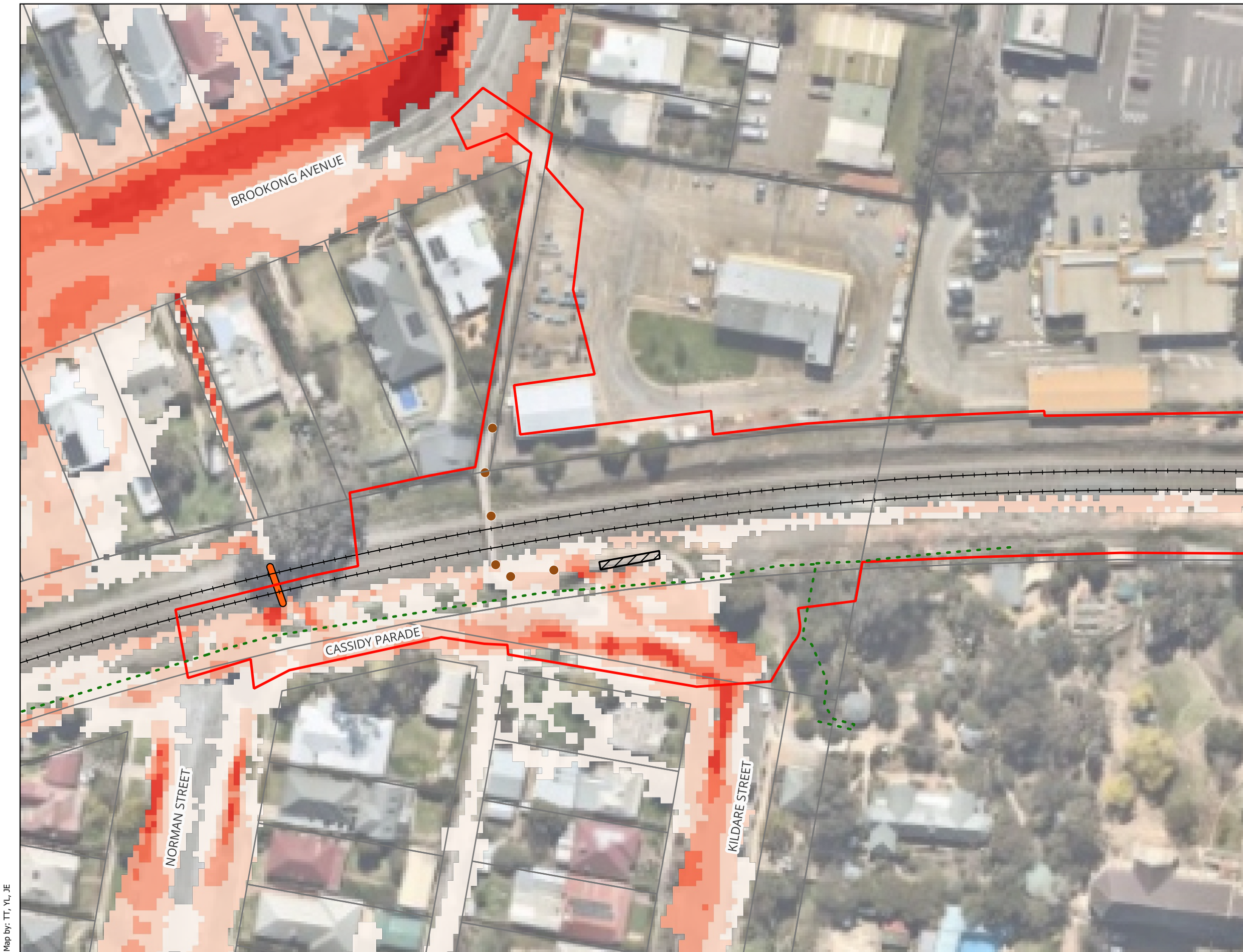
Cassidy Parade Footbridge - Inland Rail (A2P) - IFC Stage Figure A11 : 1% AEP Peak Flood Velocity - Existing Condition
