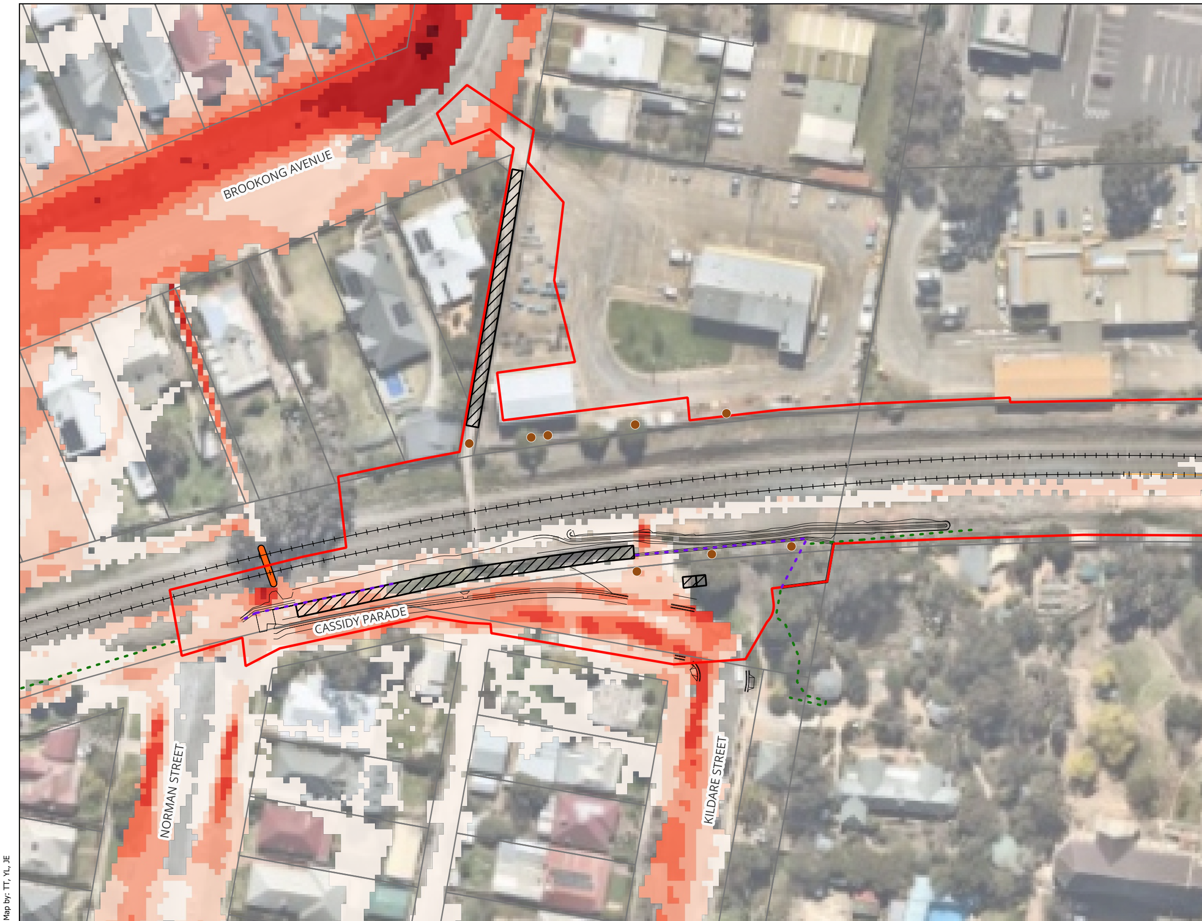
Figure A33 : 1% AEP Climate Changes Peak Flood Velocity - Master Design Condition
