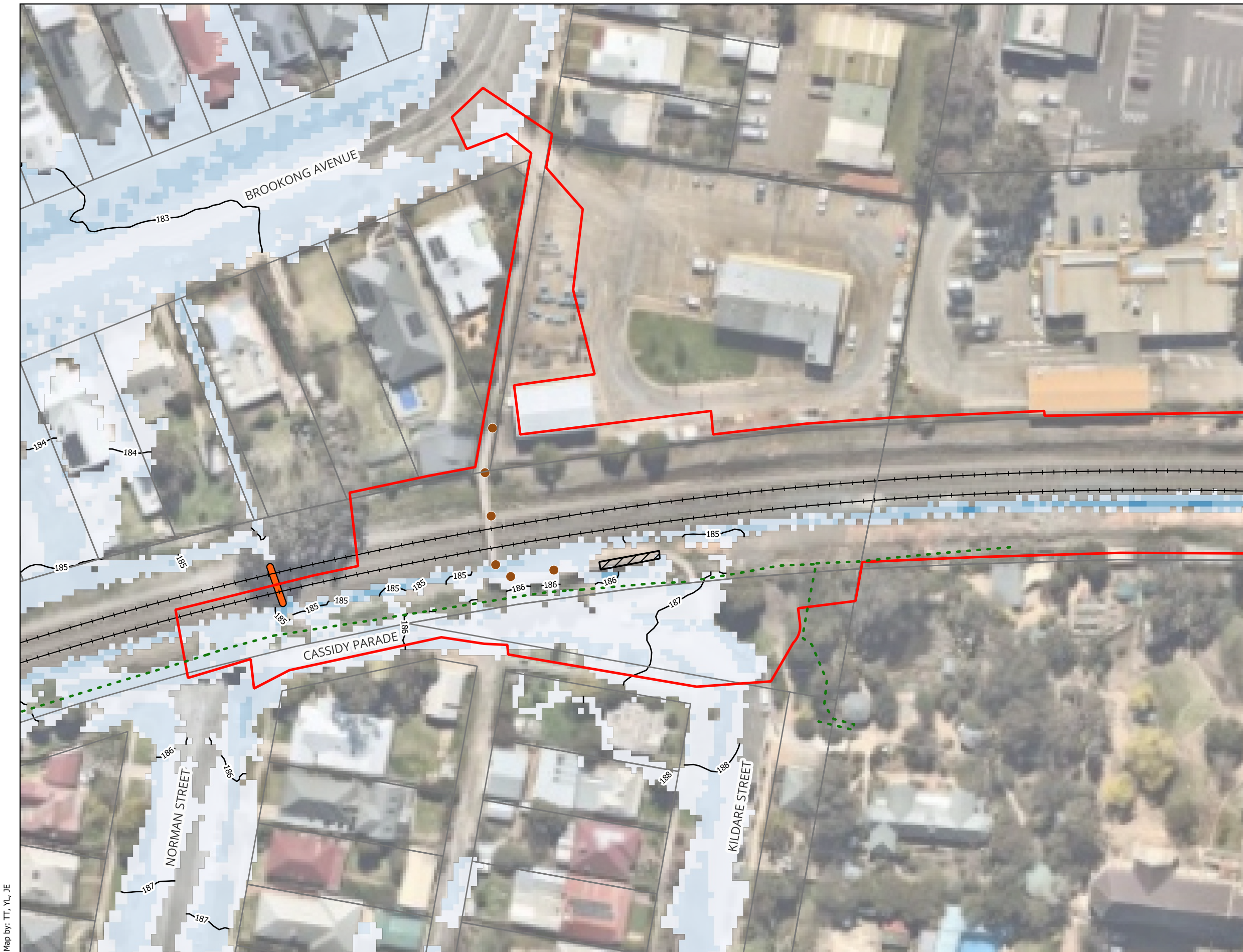
Figure A02 : 5% AEP Peak Flood Depth and Levels - Existing Condition
