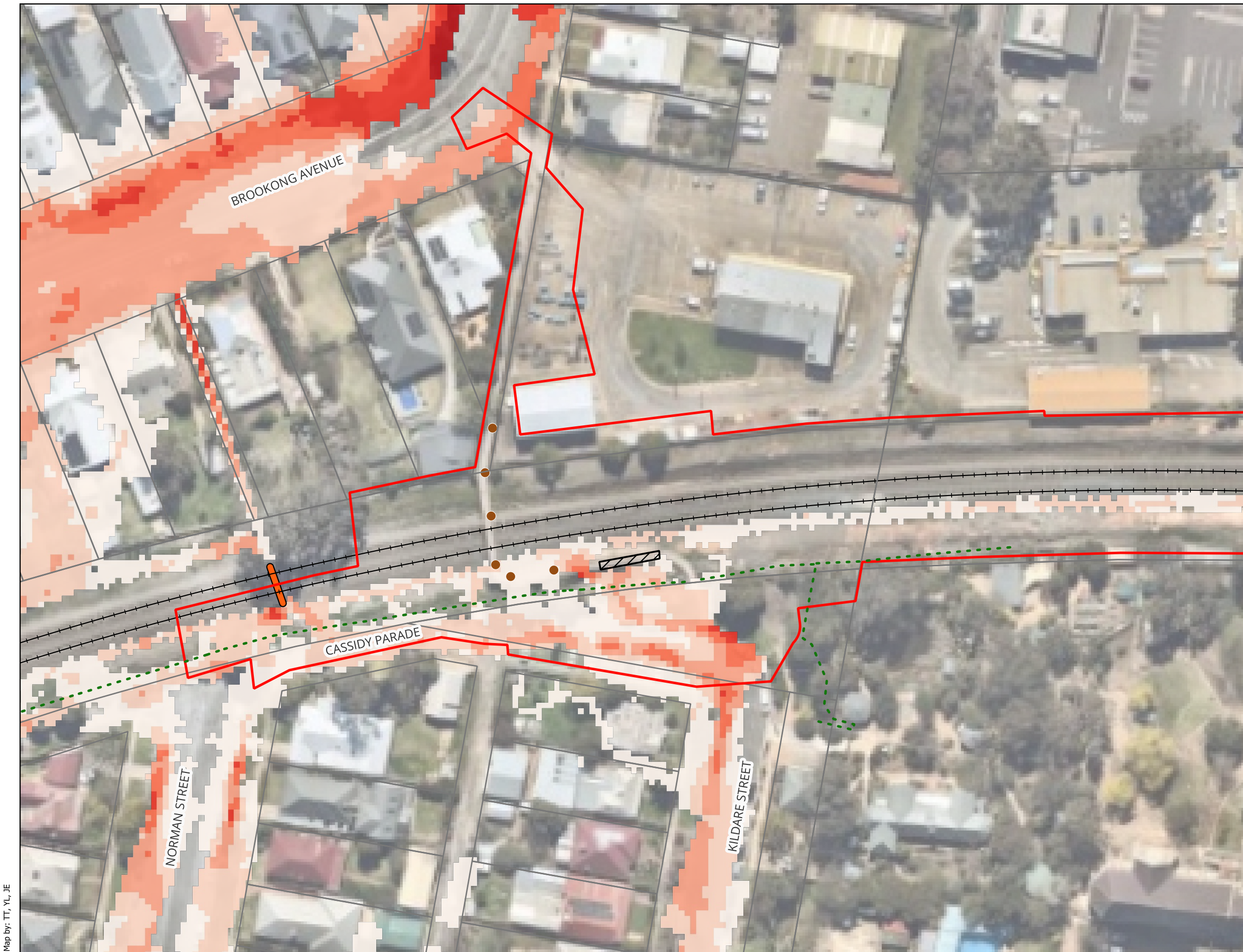
Cassidy Parade Footbridge - Inland Rail (A2P) - IFC Stage Figure A09 : 5% AEP Peak Flood Velocity - Existing Condition
