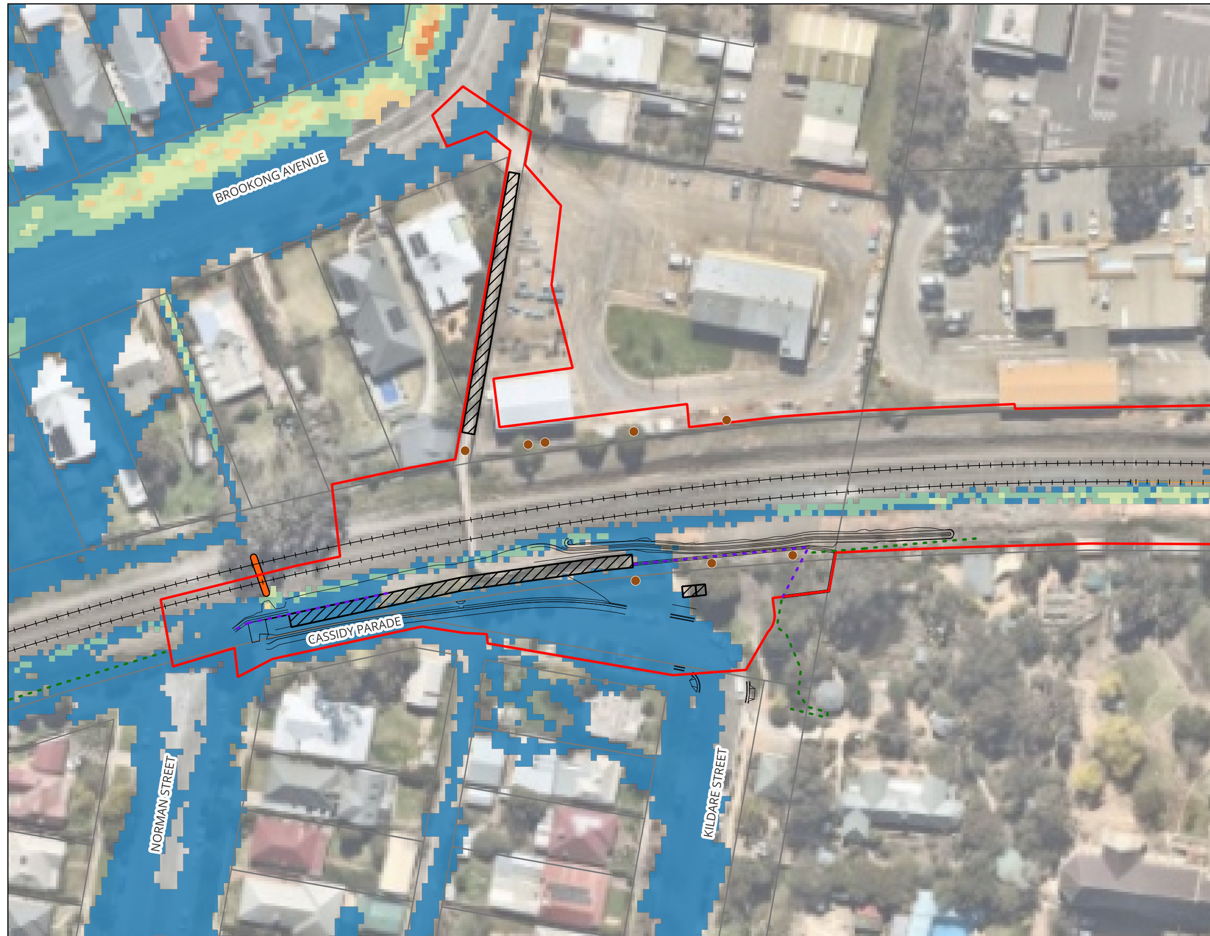
Figure A60 : 1% AEP Peak Flood Hazard - Master Design Blockage Condition
