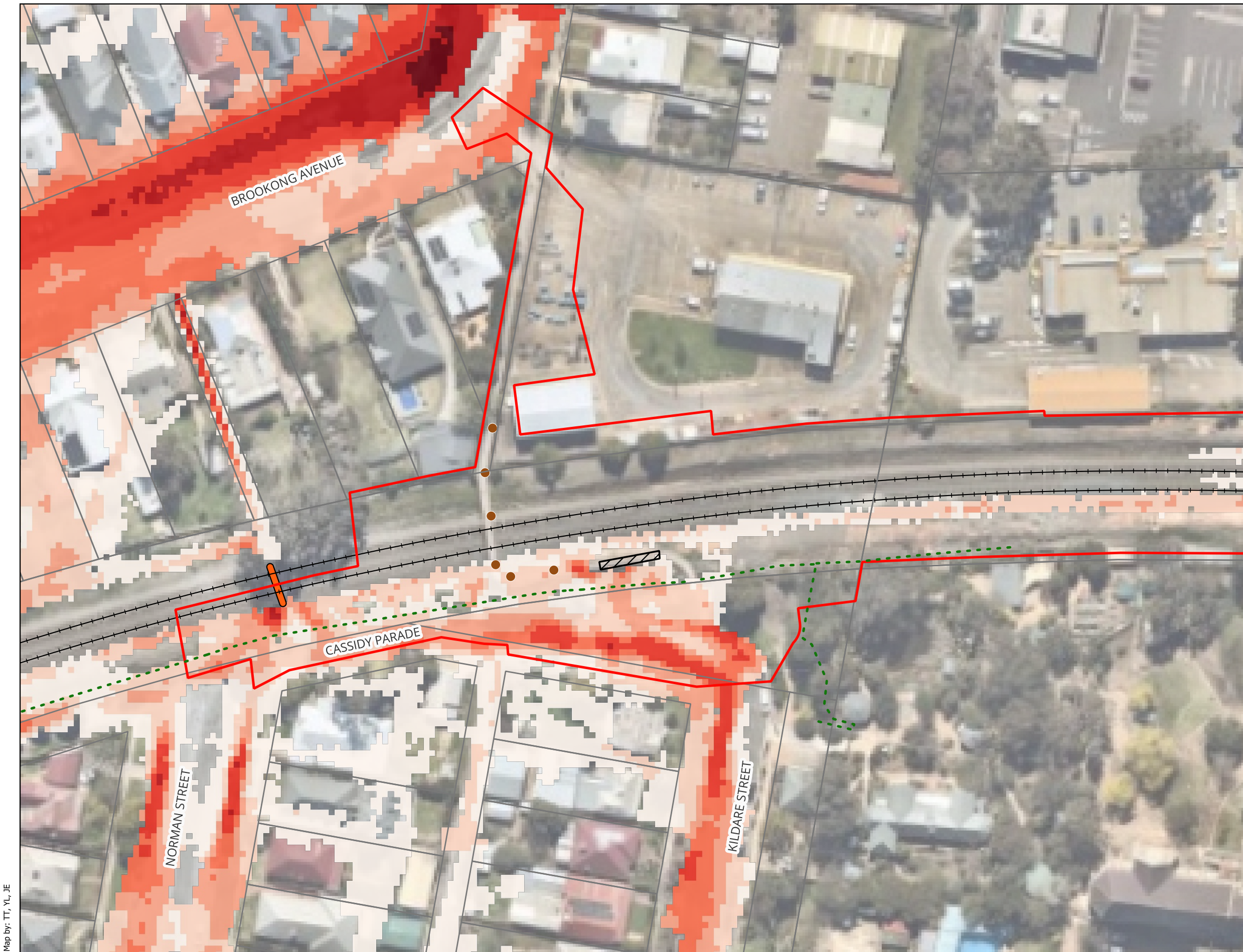
Cassidy Parade Footbridge - Inland Rail (A2P) - IFC Stage Figure A13 : 0.05% AEP Peak Flood Velocity - Existing Condition
