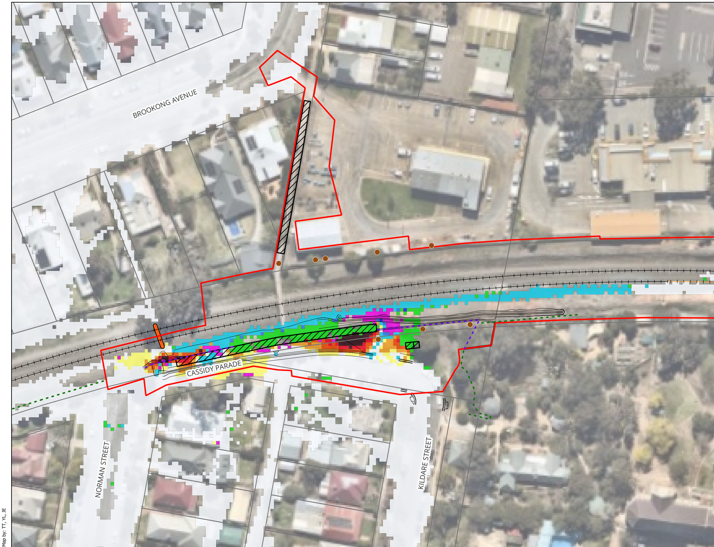
Figure A47 : Changes in Peak Flood Levels for 1% AEP Climate Changes - Master Design Condition vs Existing Condition
