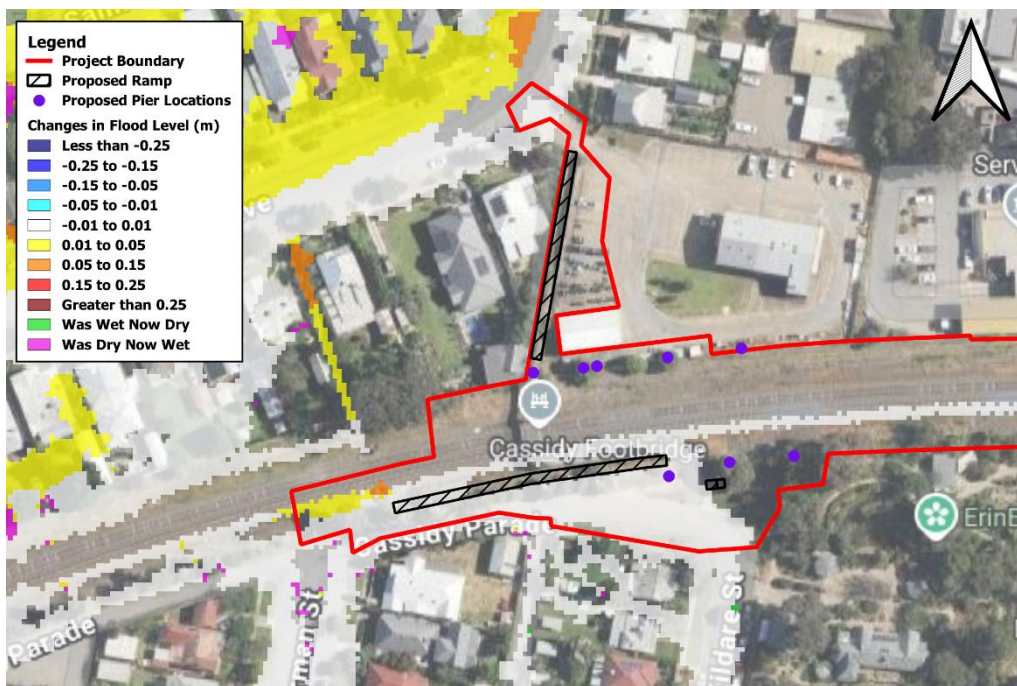
FIGURE 6:9: FLOOD LEVEL COMPARISON FOR 1% AEP DESIGN CONDITION – BLOCKAGE VS DESIGN
