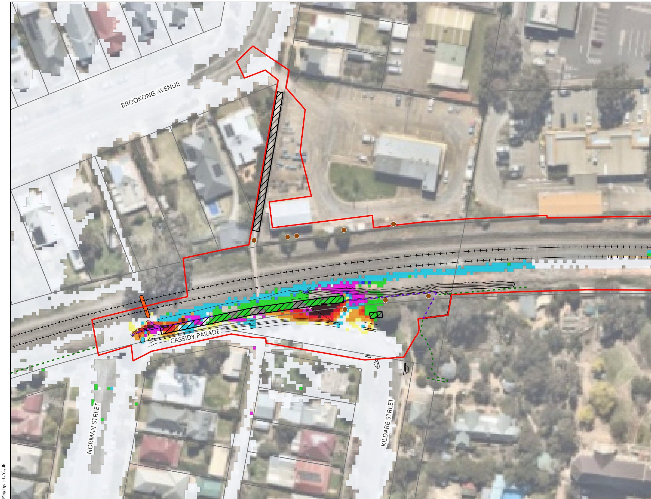
Figure A46 : Changes in Peak Flood Levels for 1% AEP - Master Design Condition vs Existing Condition
