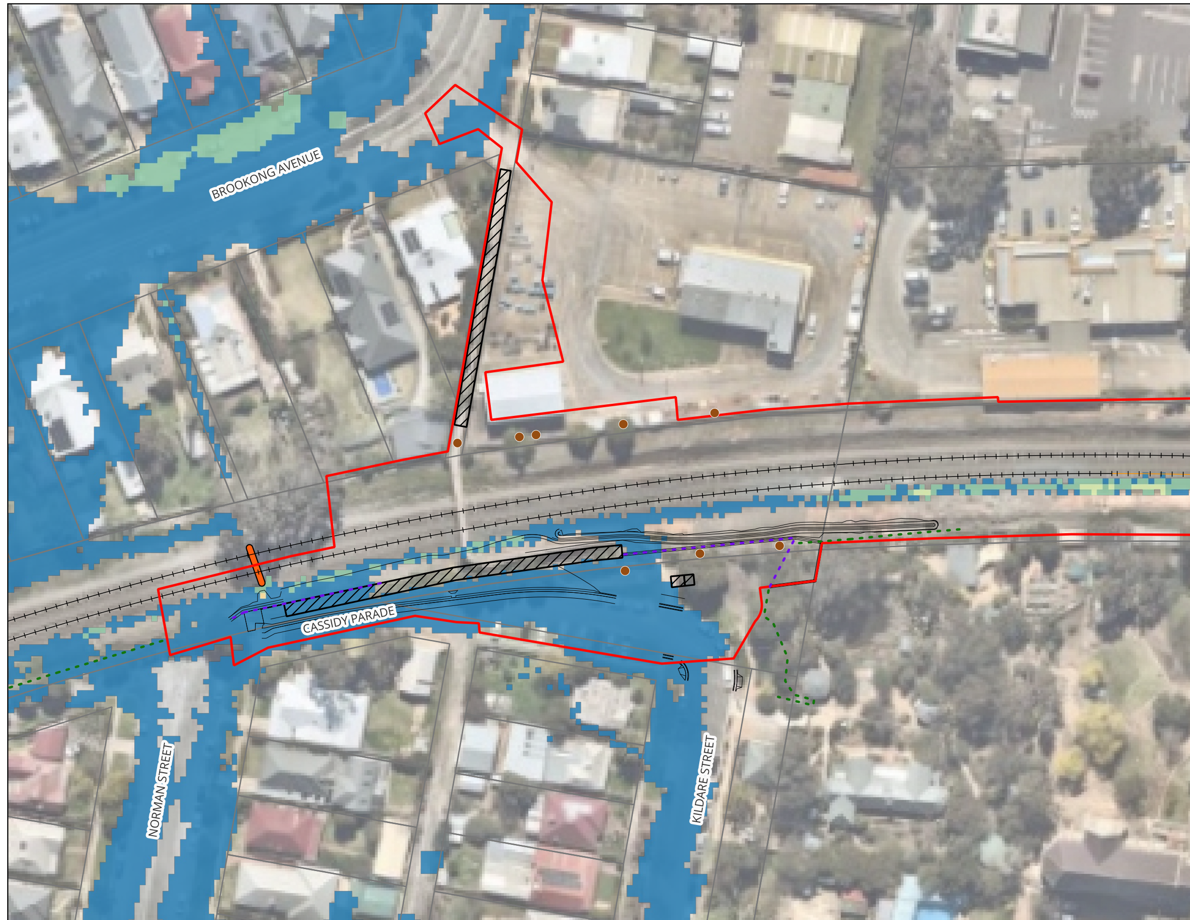
Cassidy Parade Footbridge - Inland Rail (A2P) - IFC Stage Figure A36 : 10% AEP Peak Flood Hazard - Master Design Condition
