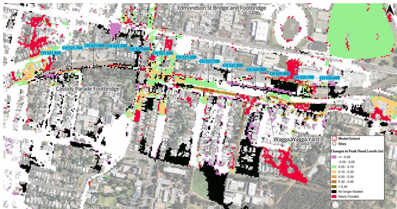
FIGURE 5:2: COMPARISON - CHANGES IN PEAK FLOOD LEVELS ZOOMED IN (UPDATED TUFLOW MODEL VS MOFFS 2021 TUFLOW MODEL)
