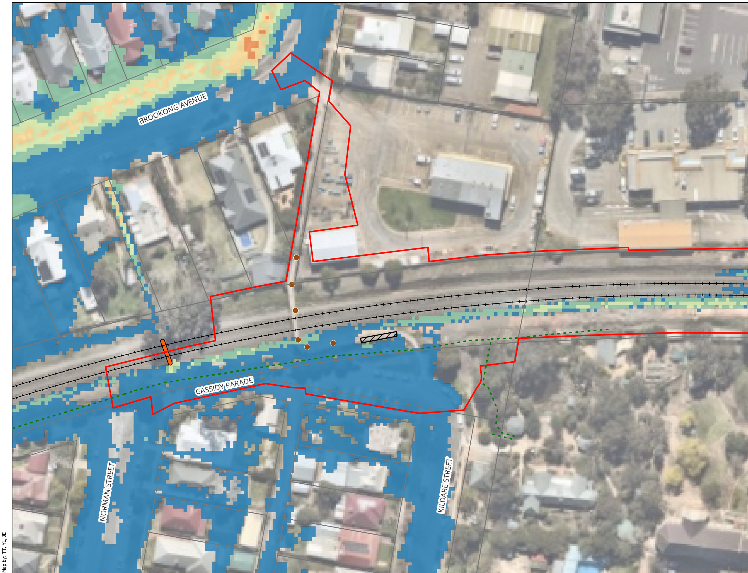
Cassidy Parade Footbridge - Inland Rail (A2P) - IFC Stage Figure A20 : 0.05% AEP Peak Flood Hazard - Existing Condition
