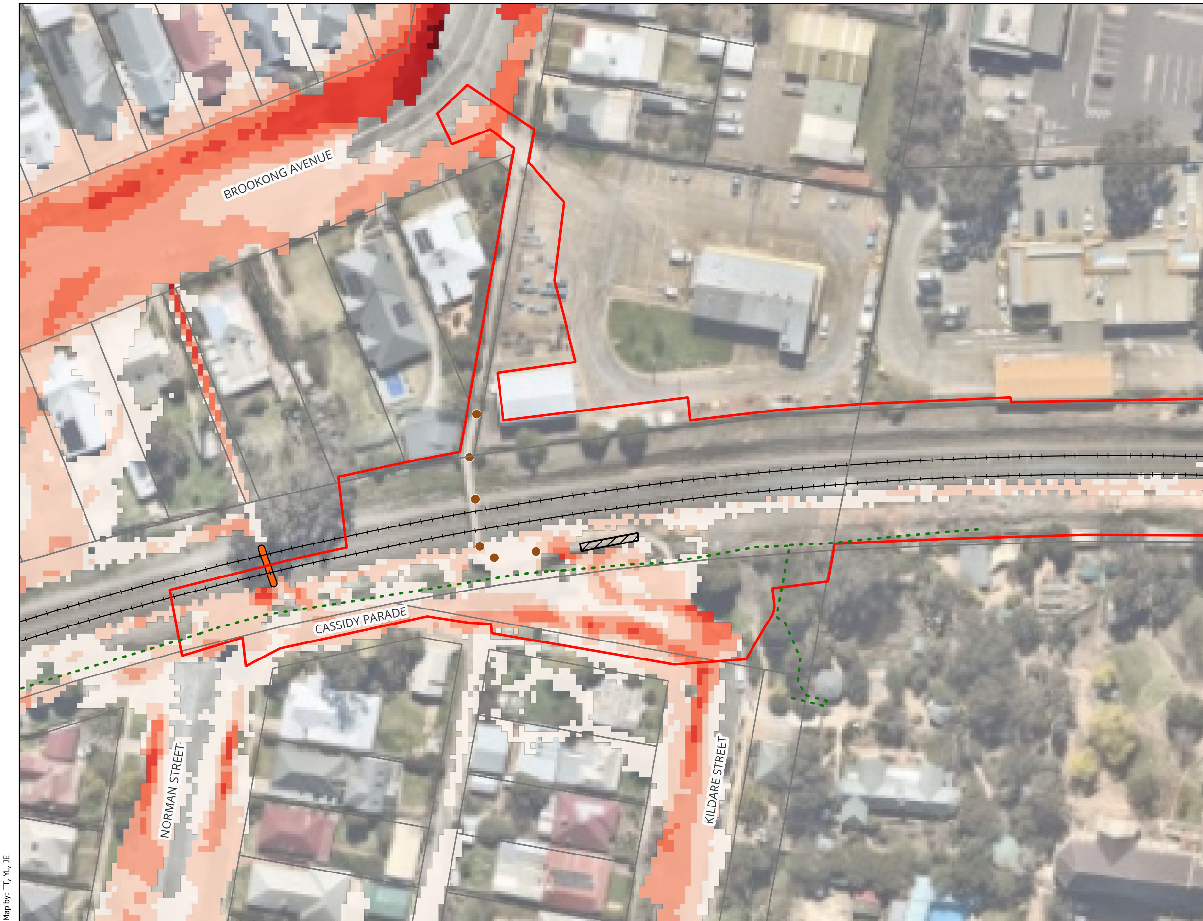
Cassidy Parade Footbridge - Inland Rail (A2P) - IFC Stage Figure A10 : 2% AEP Peak Flood Velocity - Existing Condition
