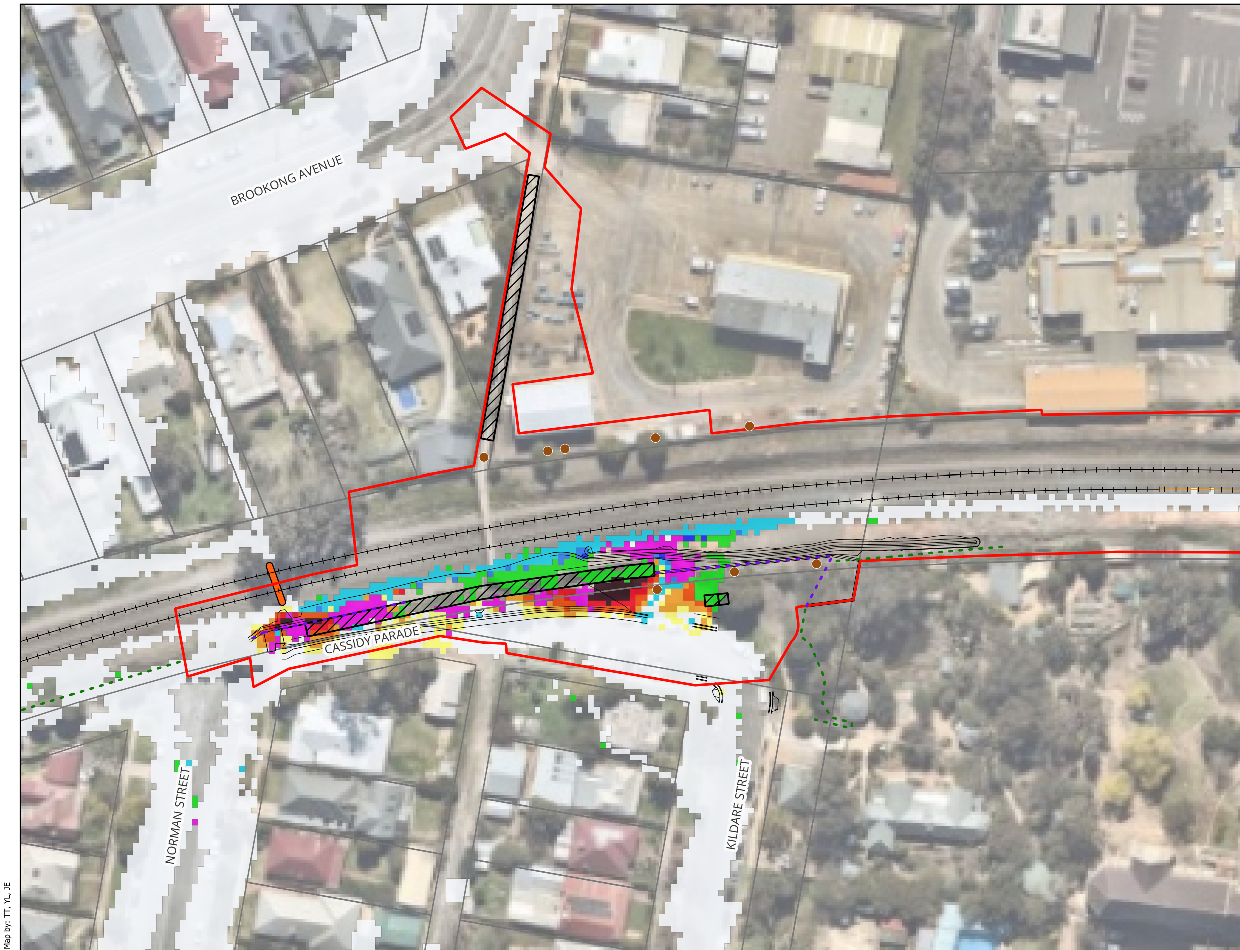
Figure A43 : Changes in Peak Flood Levels for 10% AEP - Master Design Condition vs Existing Condition
