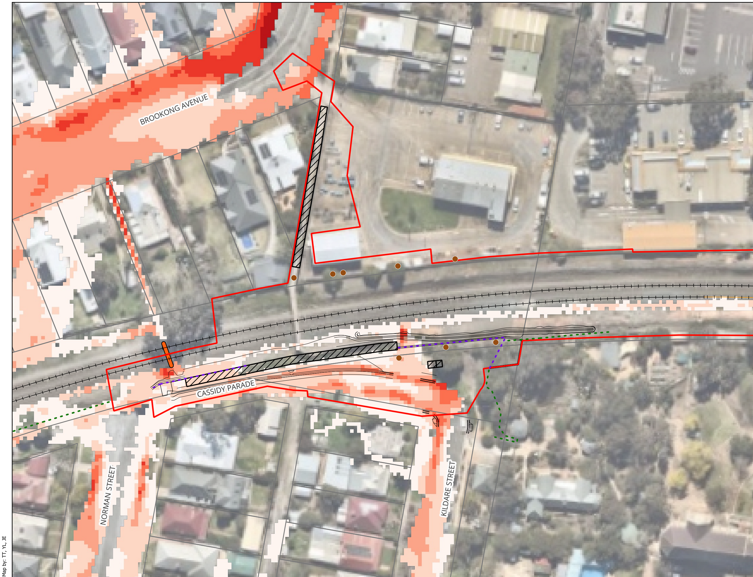
Cassidy Parade Footbridge - Inland Rail (A2P) - IFC Stage Figure A30 : 5% AEP Peak Flood Velocity - Master Design Condition
