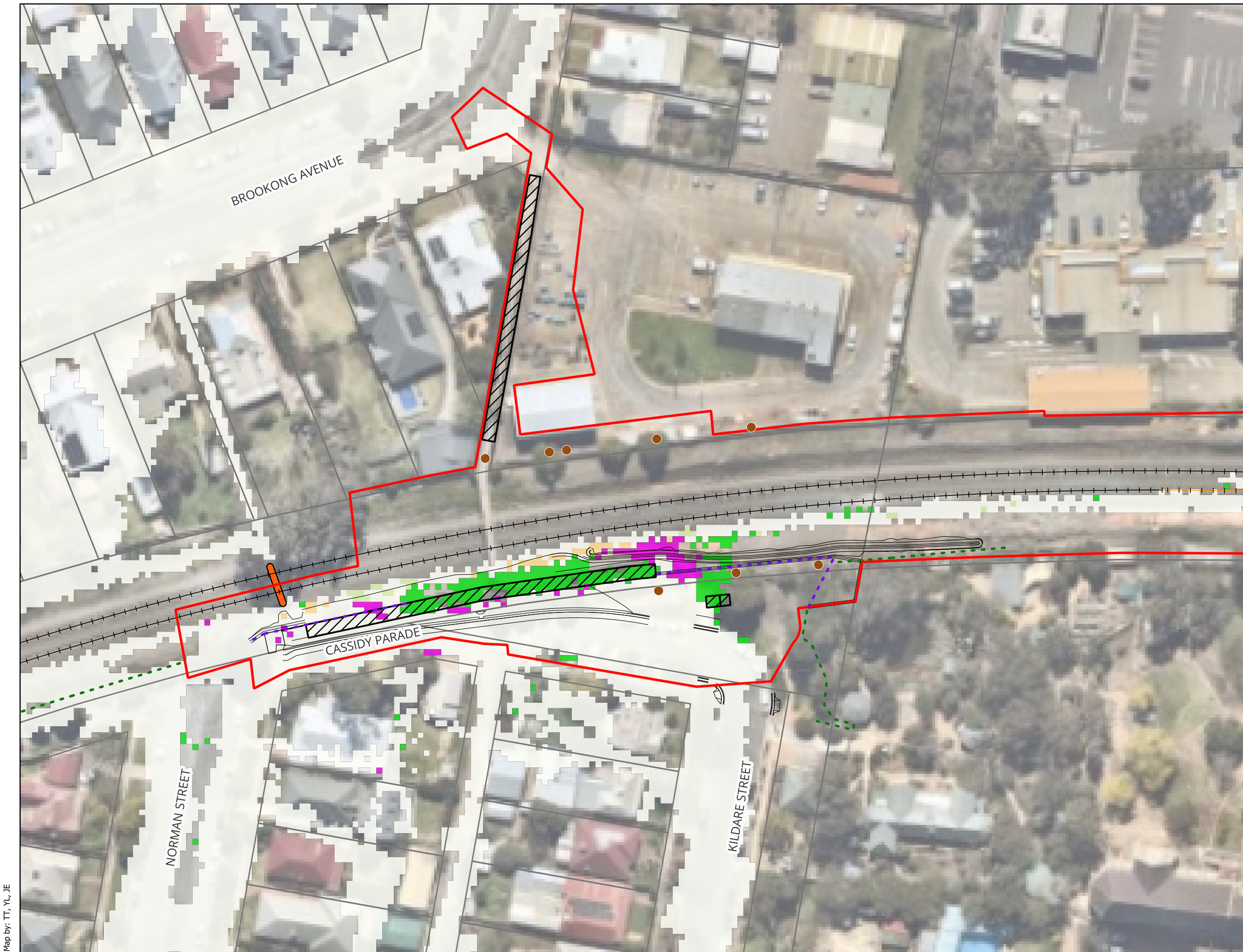
Figure A57 : Changes in Peak Flood Hazard for 1% AEP Climate Changes - Master Design Condition vs Existing Condition
