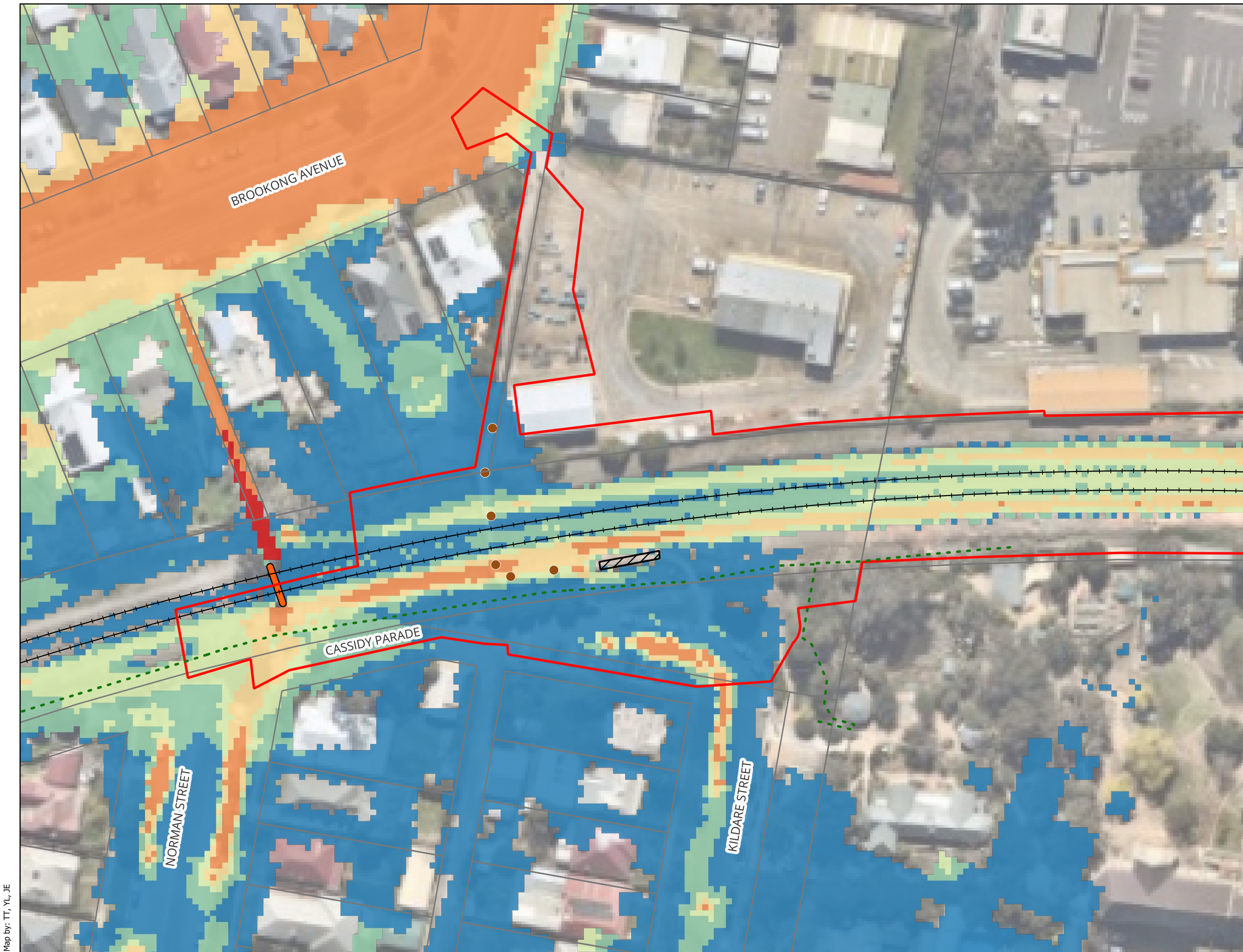
Cassidy Parade Footbridge - Inland Rail (A2P) - IFC Stage Figure A21 : PMF AEP Peak Flood Hazard - Existing Condition
