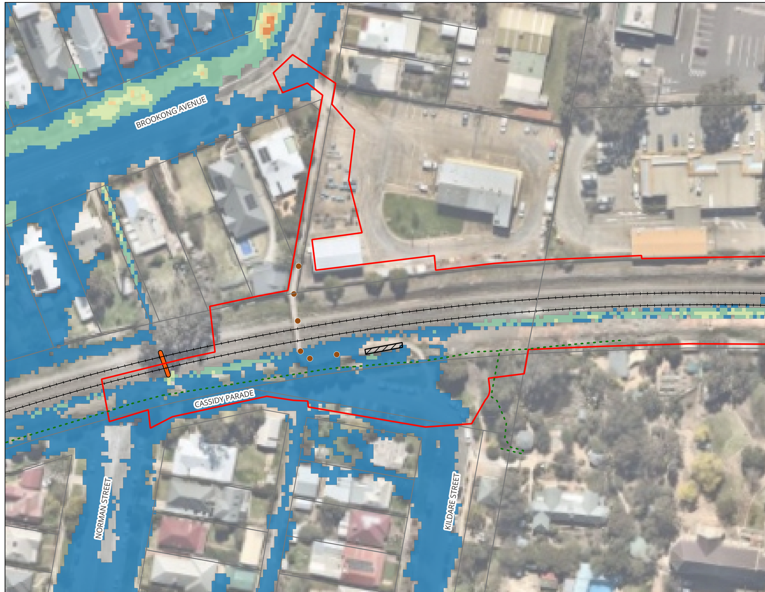
Cassidy Parade Footbridge - Inland Rail (A2P) - IFC Stage Figure A18 : 1% AEP Peak Flood Hazard - Existing Condition
