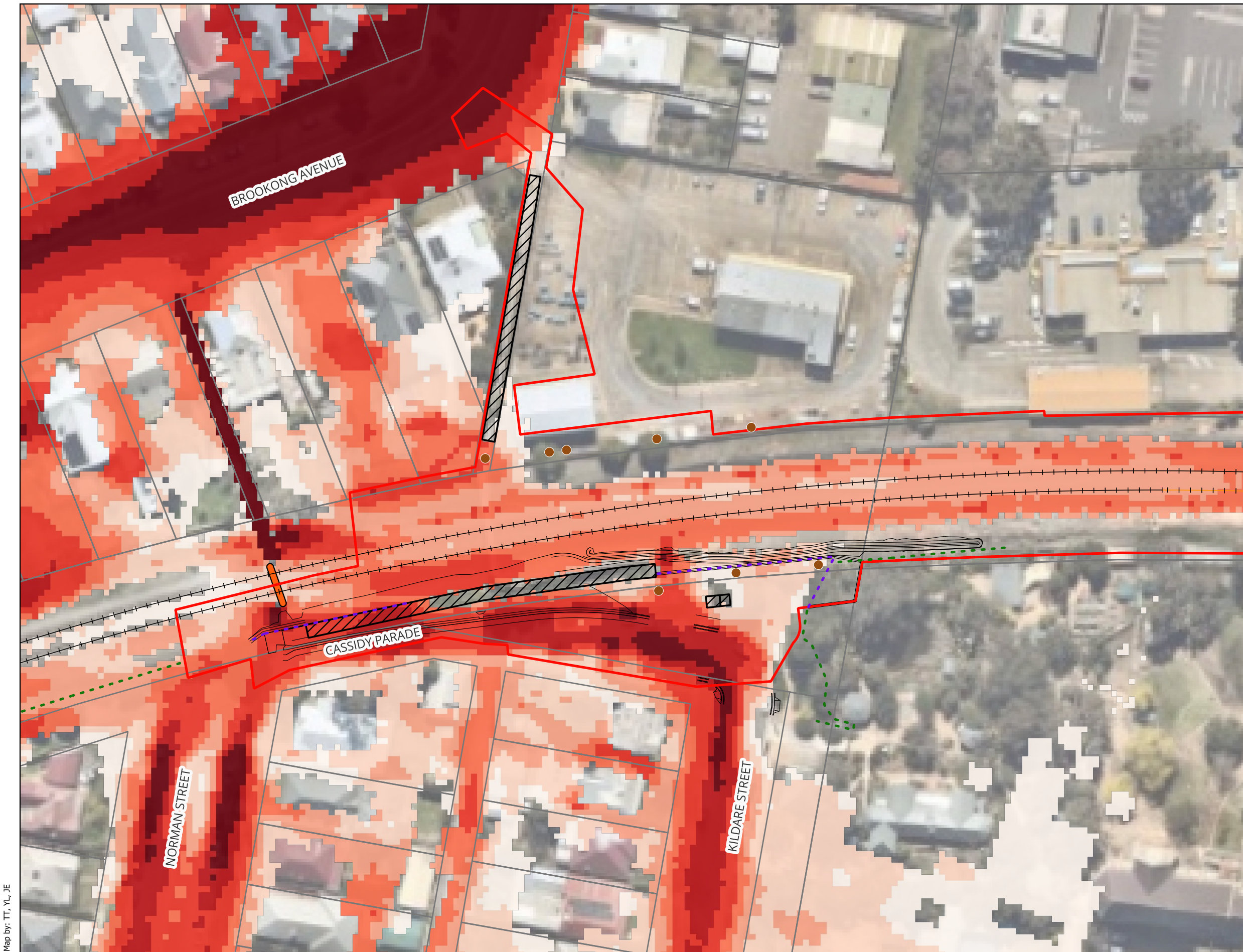
Cassidy Parade Footbridge - Inland Rail (A2P) - IFC Stage Figure A35 : PMF Peak Flood Velocity - Master Design Condition
