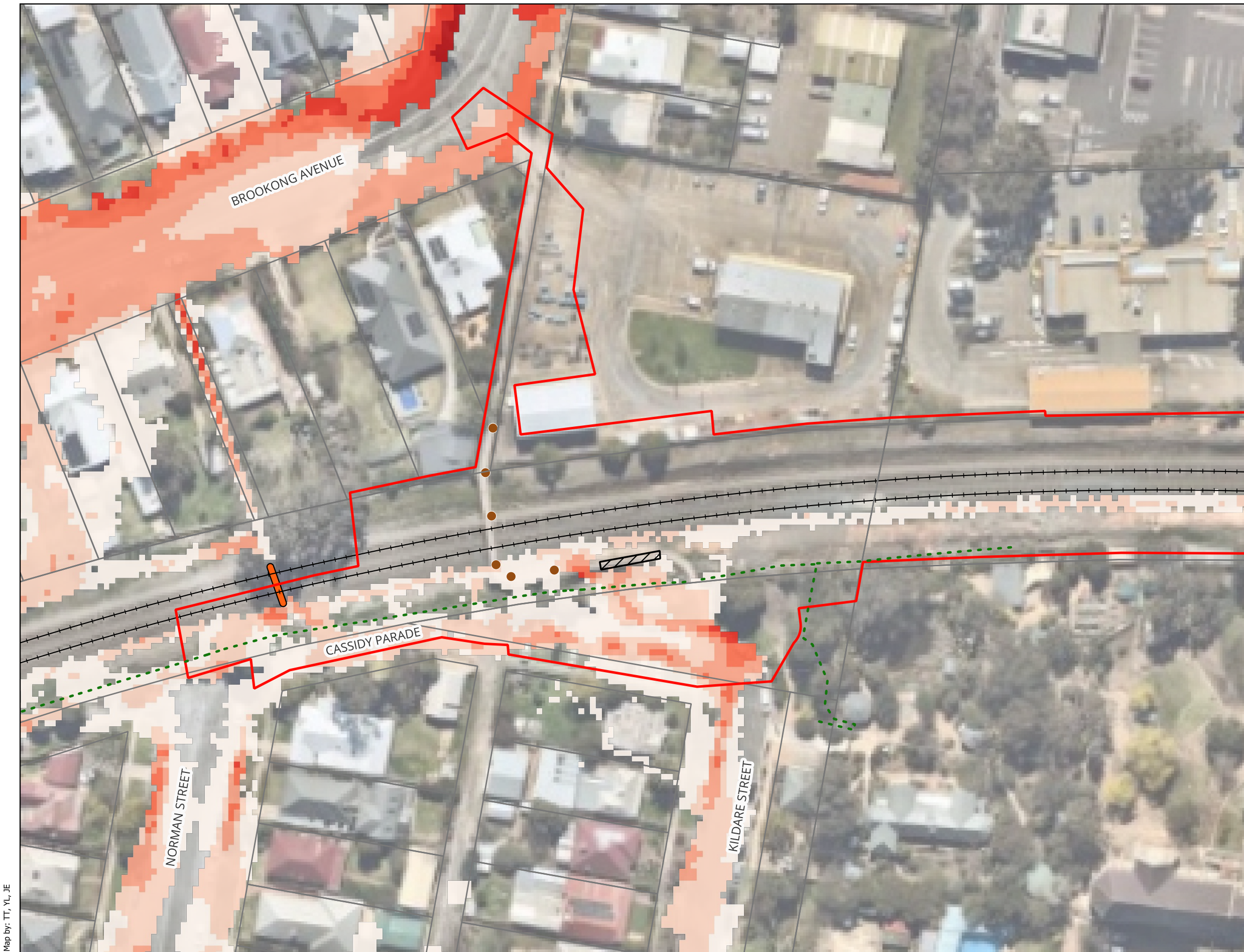
Cassidy Parade Footbridge - Inland Rail (A2P) - IFC Stage Figure A08 : 10% AEP Peak Flood Velocity - Existing Condition
