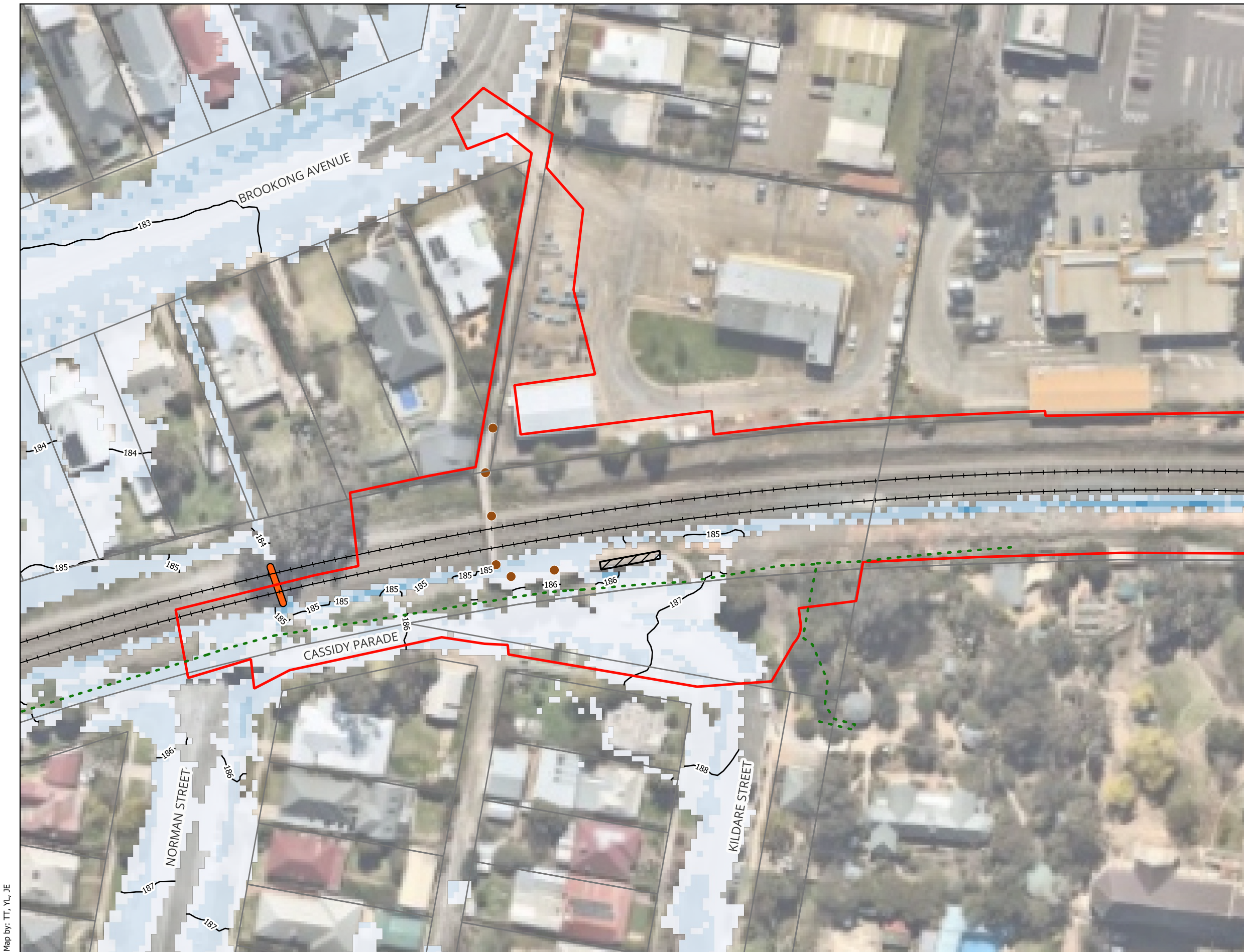
Figure A01 : 10% AEP Peak Flood Depth and Levels - Existing Condition
