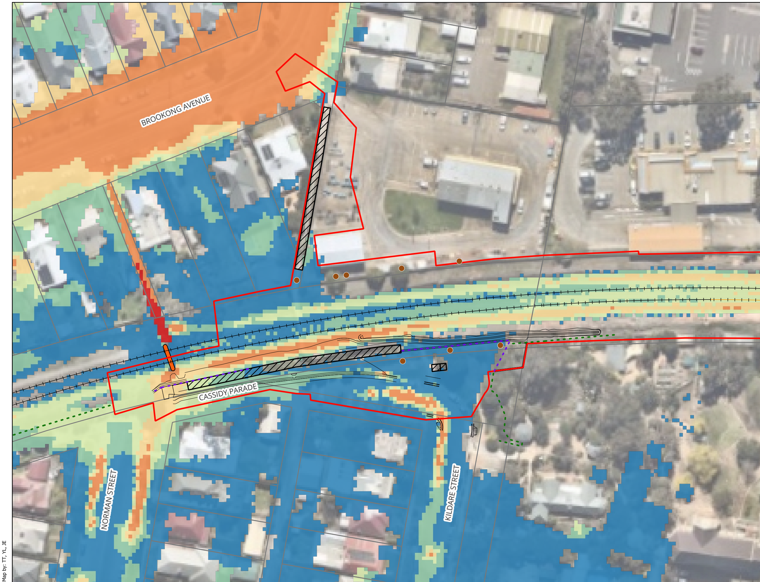
Cassidy Parade Footbridge - Inland Rail (A2P) - IFC Stage Figure A42 : PMF Peak Flood Hazard - Master Design Condition
