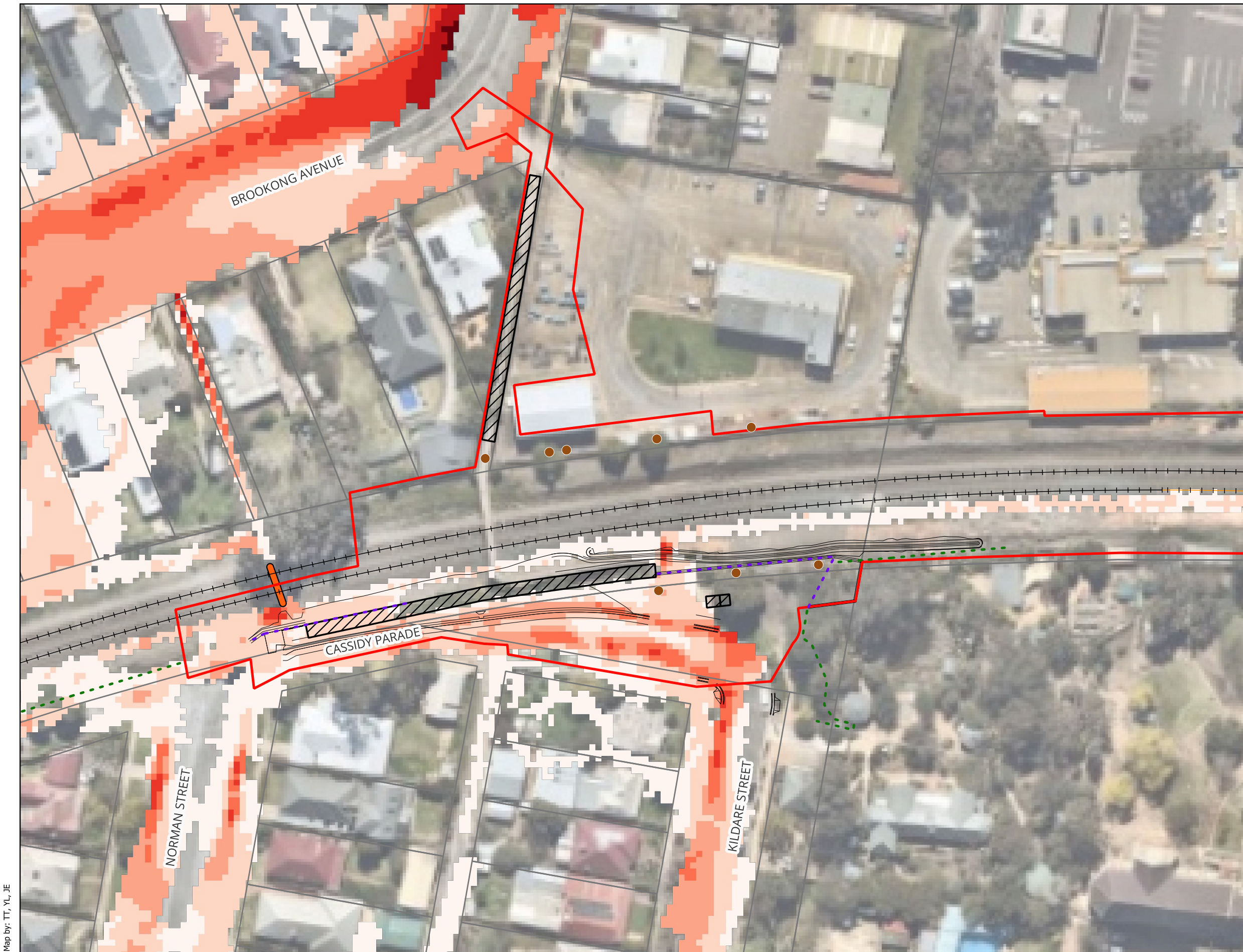
Cassidy Parade Footbridge - Inland Rail (A2P) - IFC Stage Figure A31 : 2% AEP Peak Flood Velocity - Master Design Condition
