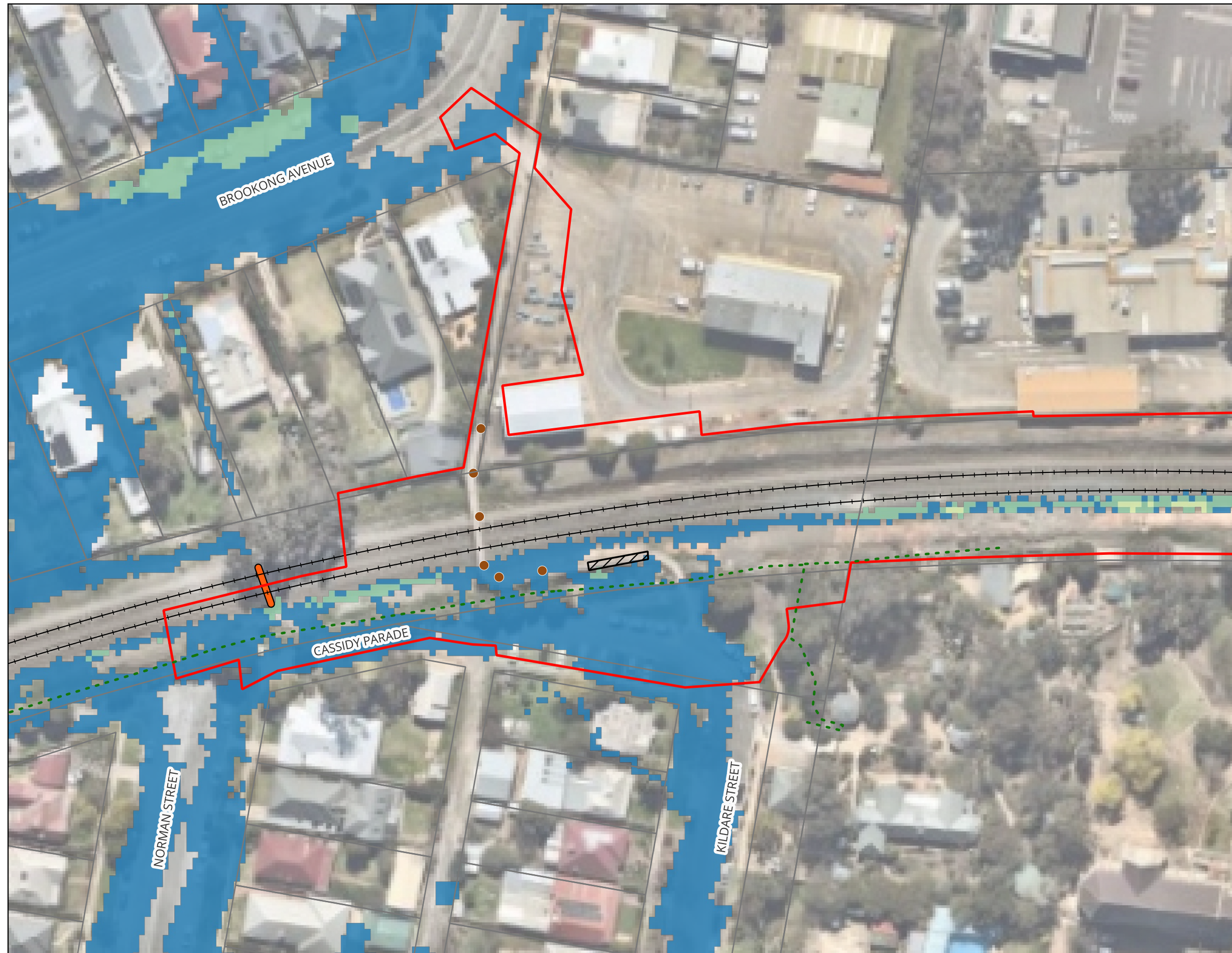
Cassidy Parade Footbridge - Inland Rail (A2P) - IFC Stage Figure A15 : 10% AEP Peak Flood Hazard - Existing Condition
