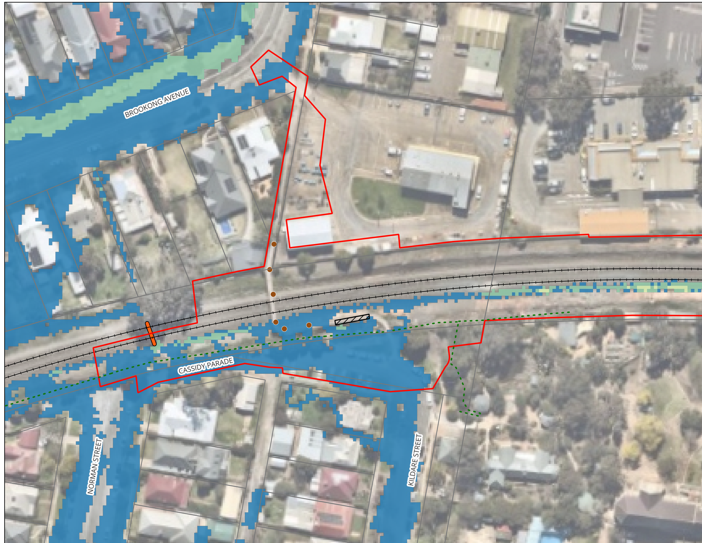
Cassidy Parade Footbridge - Inland Rail (A2P) - IFC Stage Figure A16 : 5% AEP Peak Flood Hazard - Existing Condition
