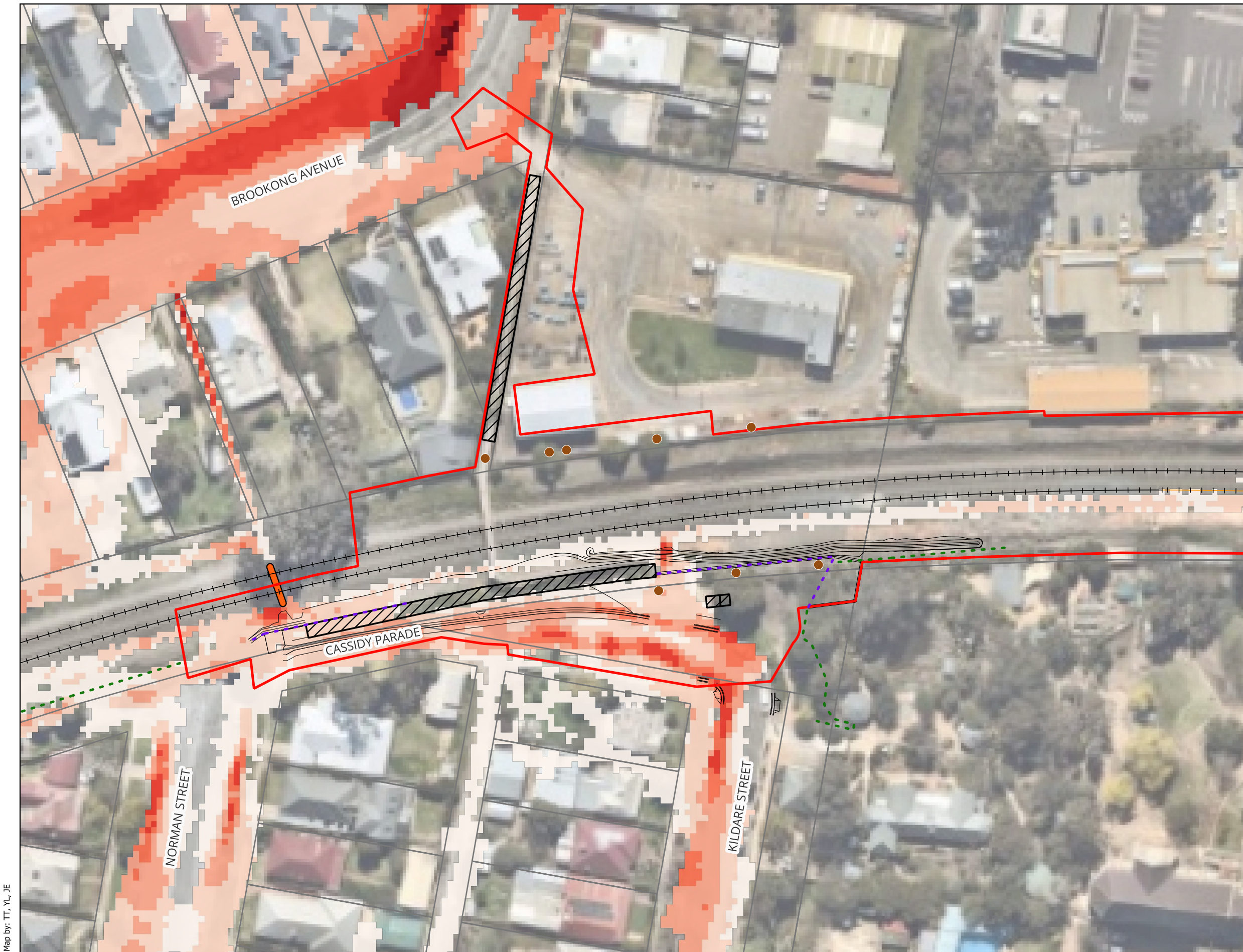
Cassidy Parade Footbridge - Inland Rail (A2P) - IFC Stage Figure A32 : 1% AEP Peak Flood Velocity - Master Design Condition
