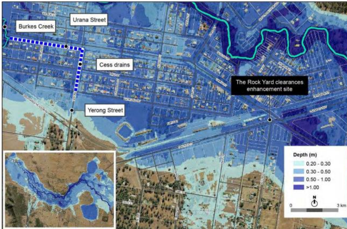
Figure 1-3: PMF flooding extent at The Rock Yard clearances enhancement site (Image source: Albury to Illabo EIS Technical Paper 11 Figure 4.24 (July 2022))
