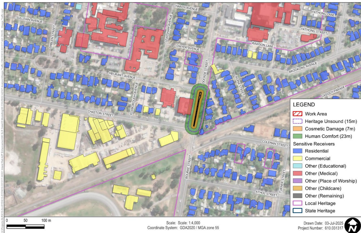
Figure 9 Vibratory Roller (2-4t) - Minimum Working Distances
