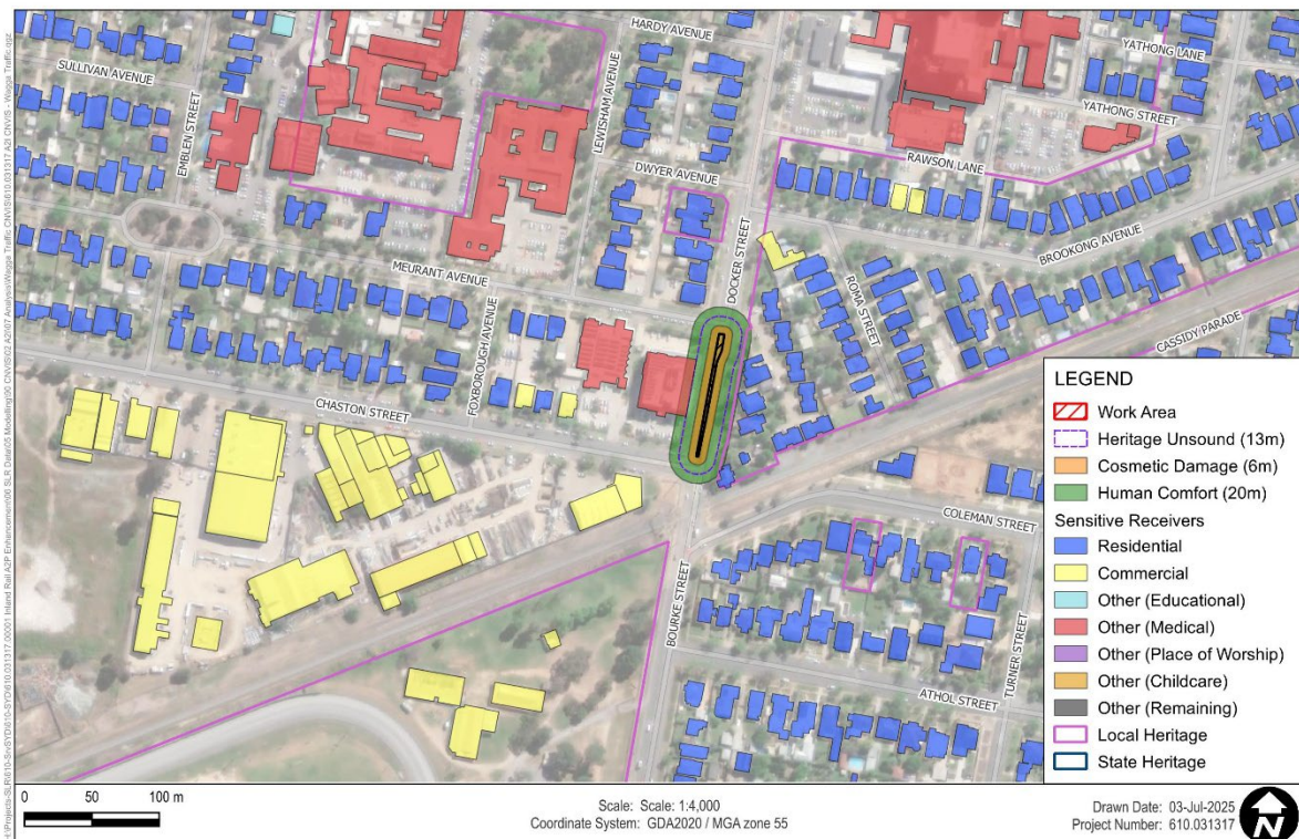
Figure 9 Vibratory Roller (2-4t) - Minimum Working Distances
