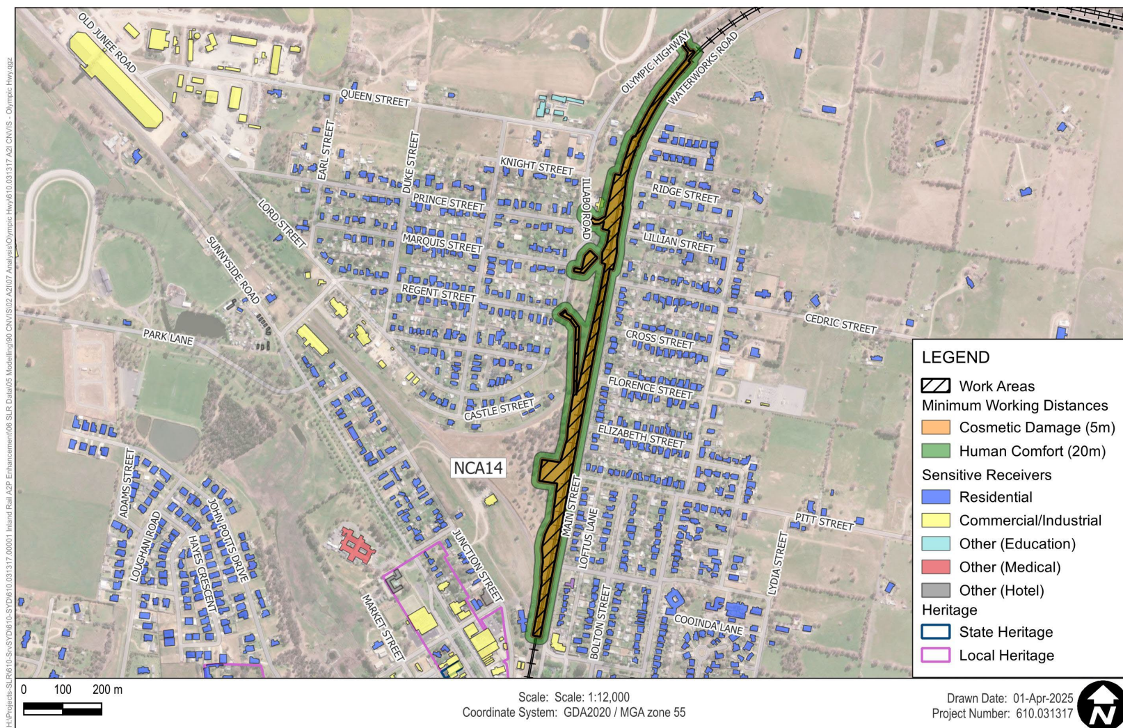
Figure 3 Construction Vibration Minimum Working Distances – Small Vibratory Roller <50 kN (1–2 tonne) (W.003)
