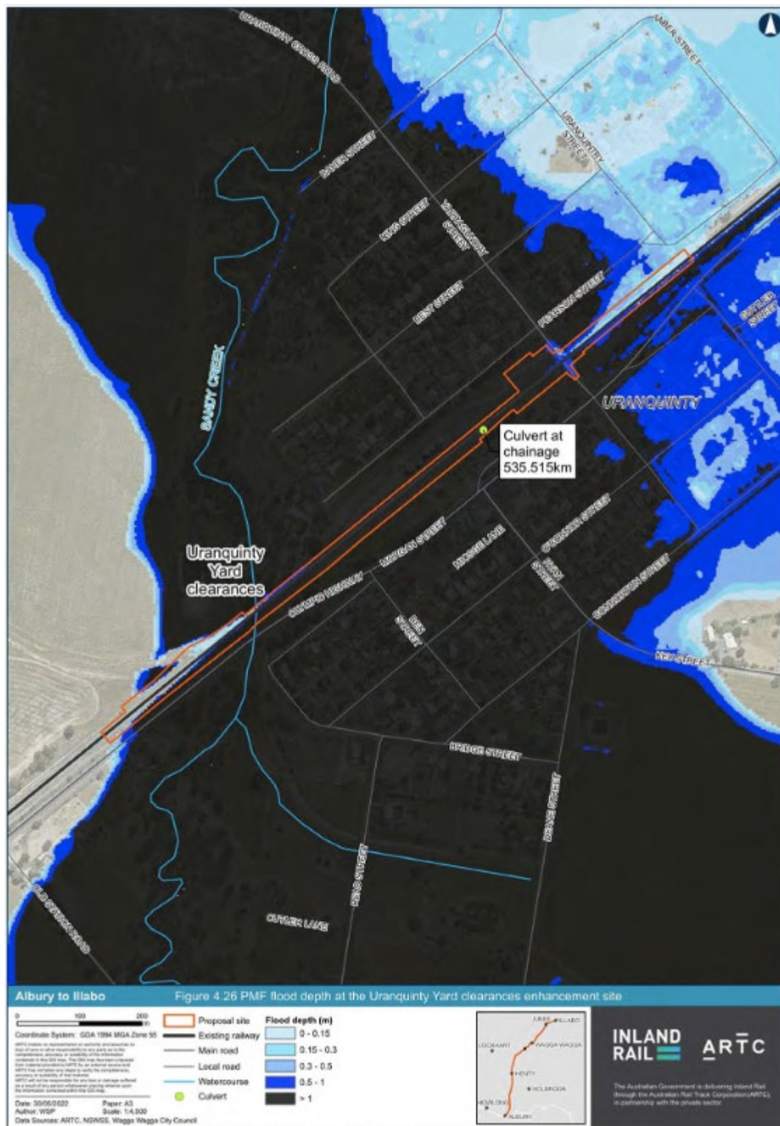
FIGURE 21: PMF FLOOD EXTENT AT URANQUINTY YARD
