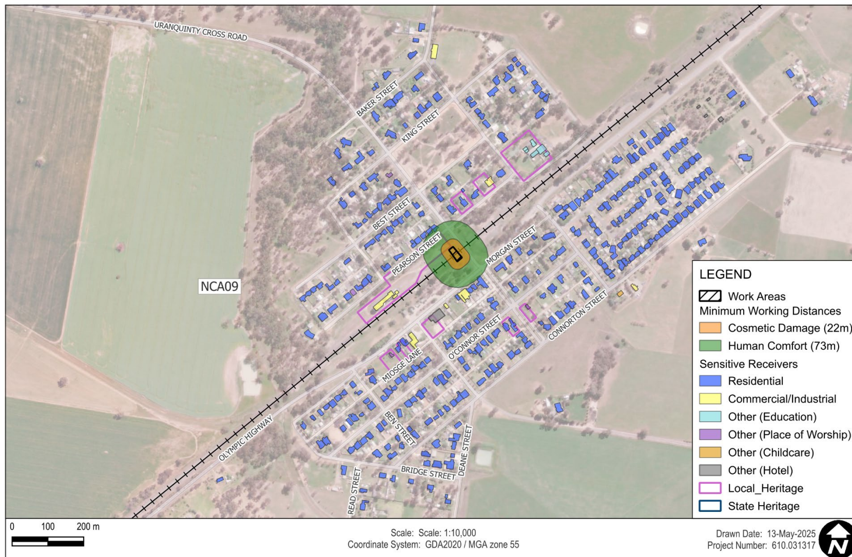
Figure 7 Minimum Working Distances – Large Hydraulic Hammer (W.014)
