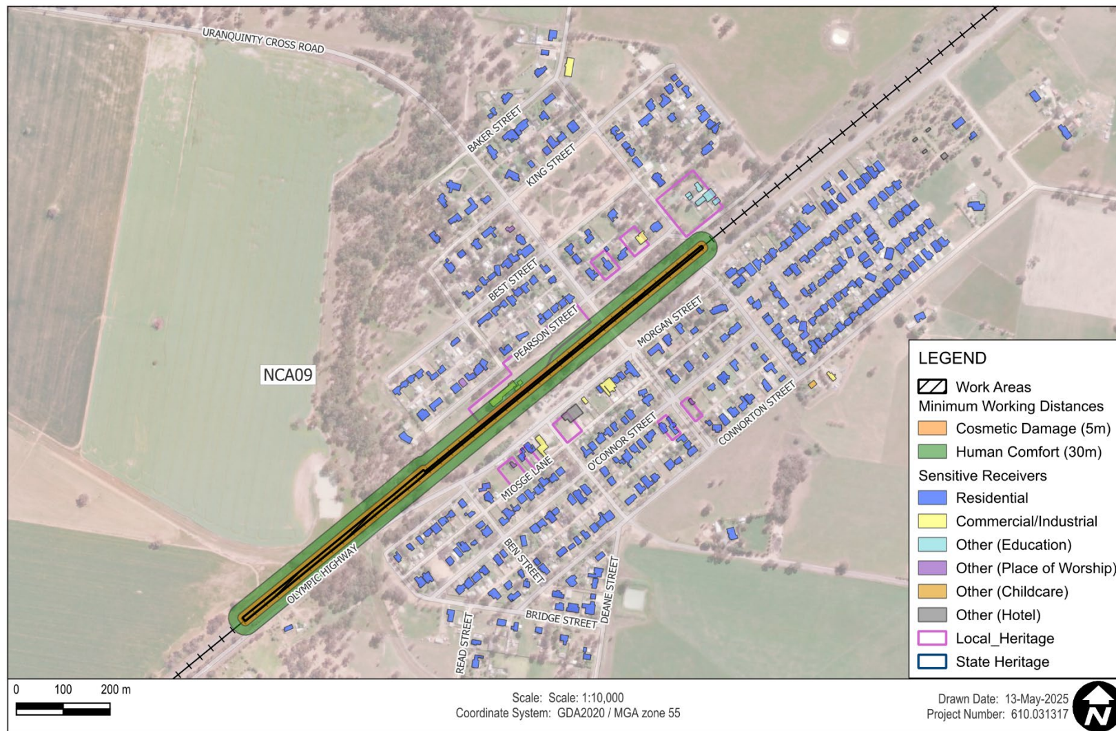
Figure 4 Minimum Working Distances – Ballast Tamping (W.007, W.012)
