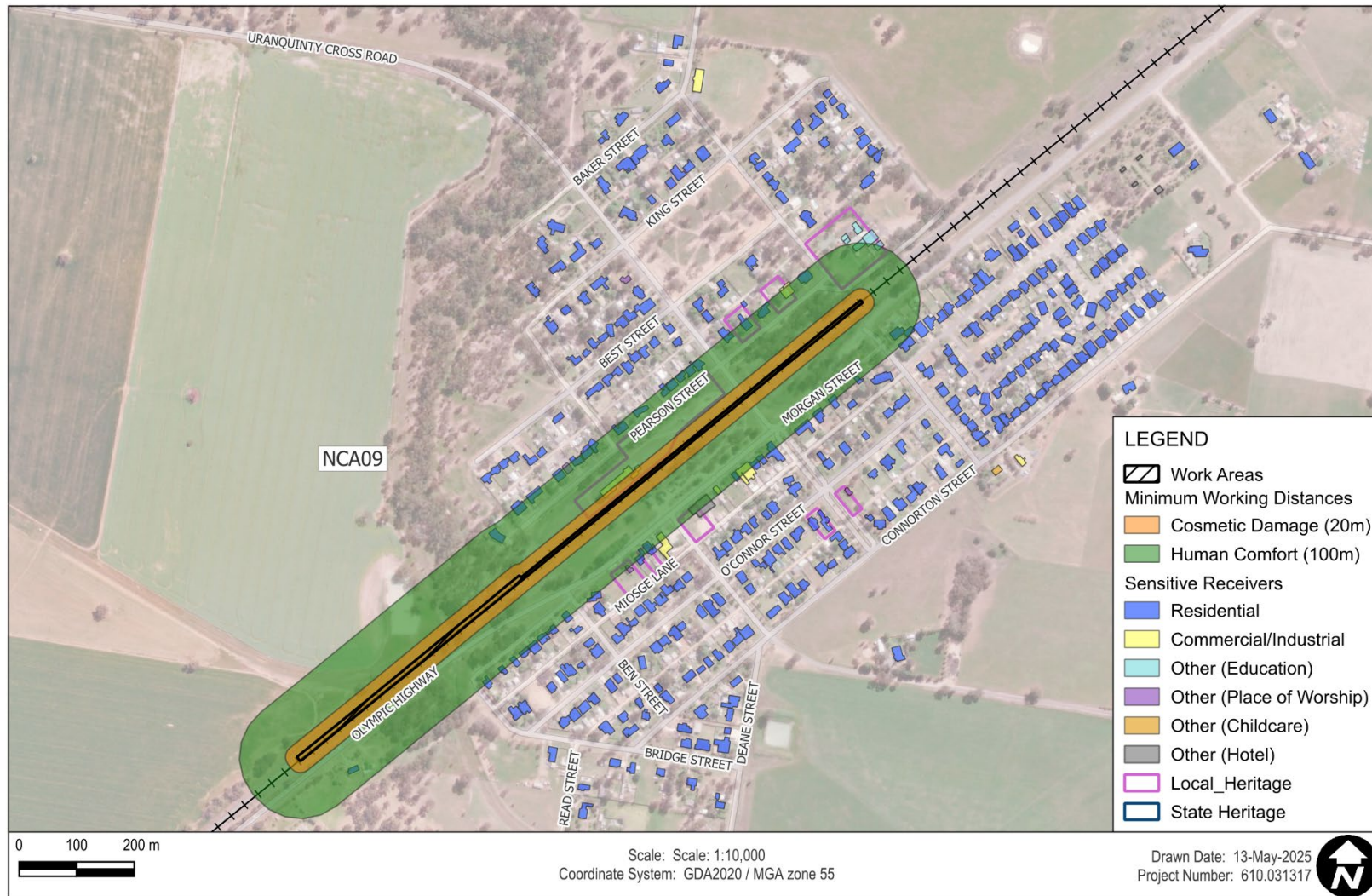
Figure 3 Minimum Working Distances – Vibratory Roller <300 kN (13-18 tonne) (W.005)
