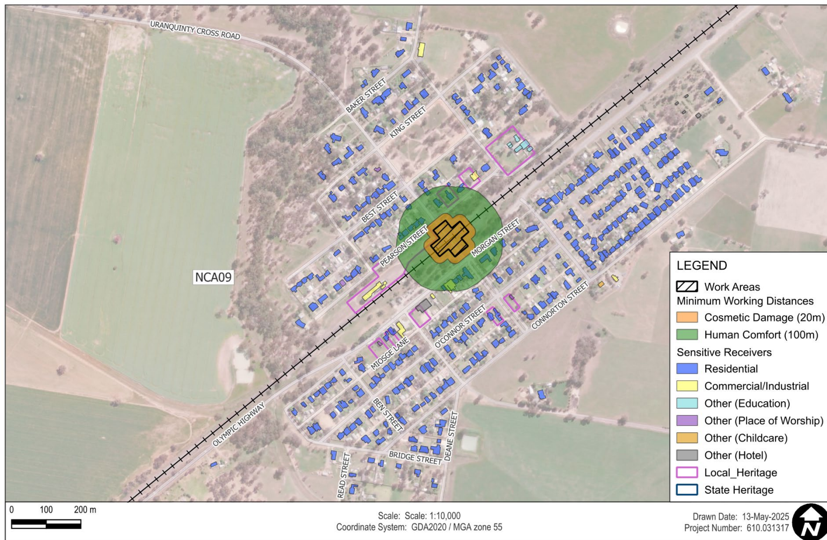
Figure 6 Minimum Working Distances – Vibratory Roller <300 kN (13-18 tonne) (W.012)
