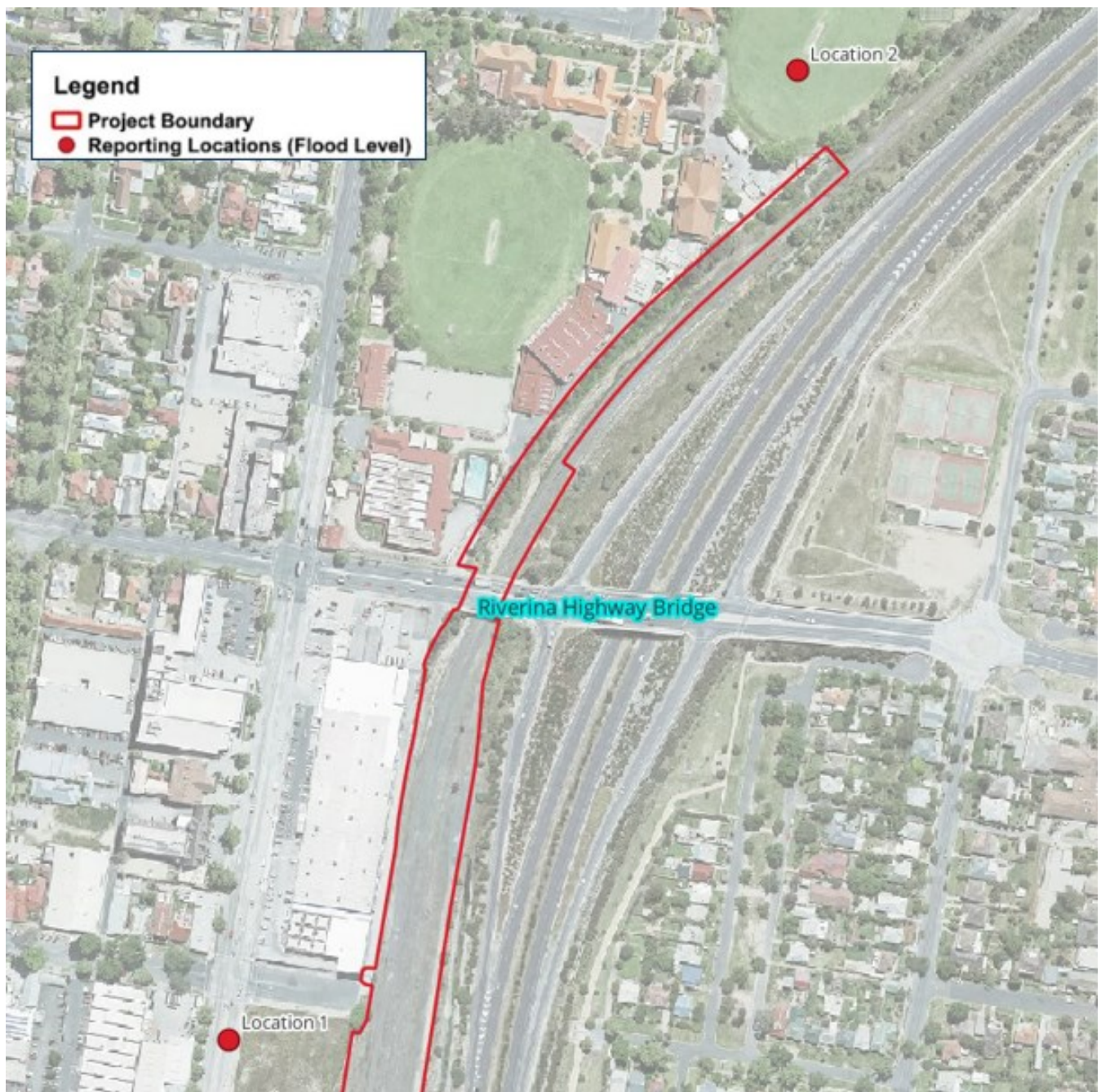
Figure 5-5: Reporting Location 1 and 2 for the Changes in Duration of Inundation, noting that the flood water flow direction is perpendicular to Location 1
