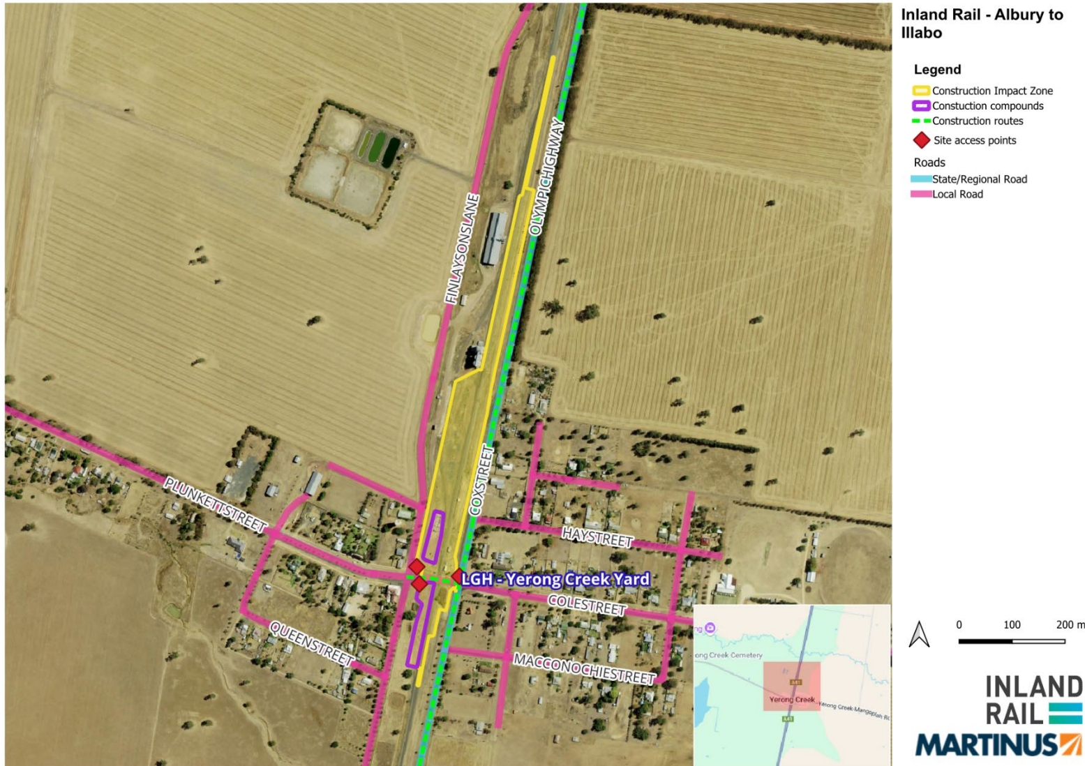
FIGURE 26 YERONG CREEK CONSTRUCTION ROUTES
