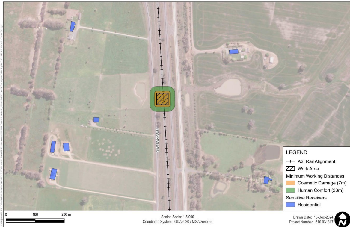
Figure 3 Construction Vibration Minimum Working Distances
