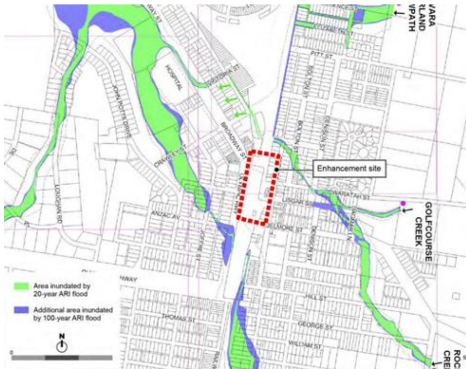
Figure 1-4: 1% AEP and 5% AEP Flood Extents at Junee Yard Clearances (Source: Albury to Illabo Environmental Impact Statement (EIS) Technical Paper 11 – Hydrology, flooding and water quality (July 2022), Figure 4.49)
