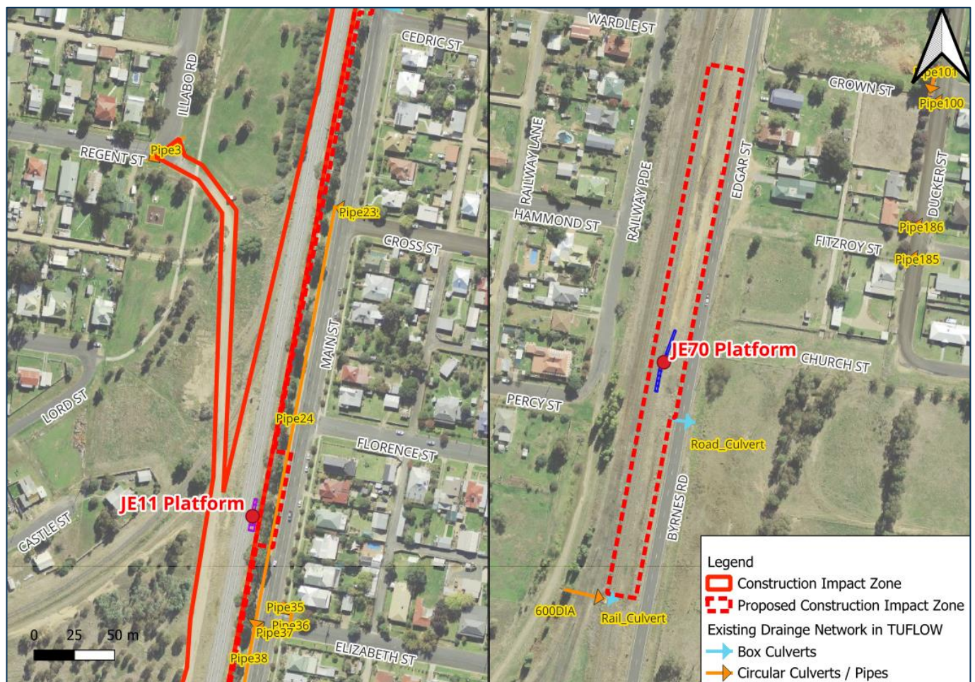
Figure 4-5: Existing Drainage Network in TUFLOW
