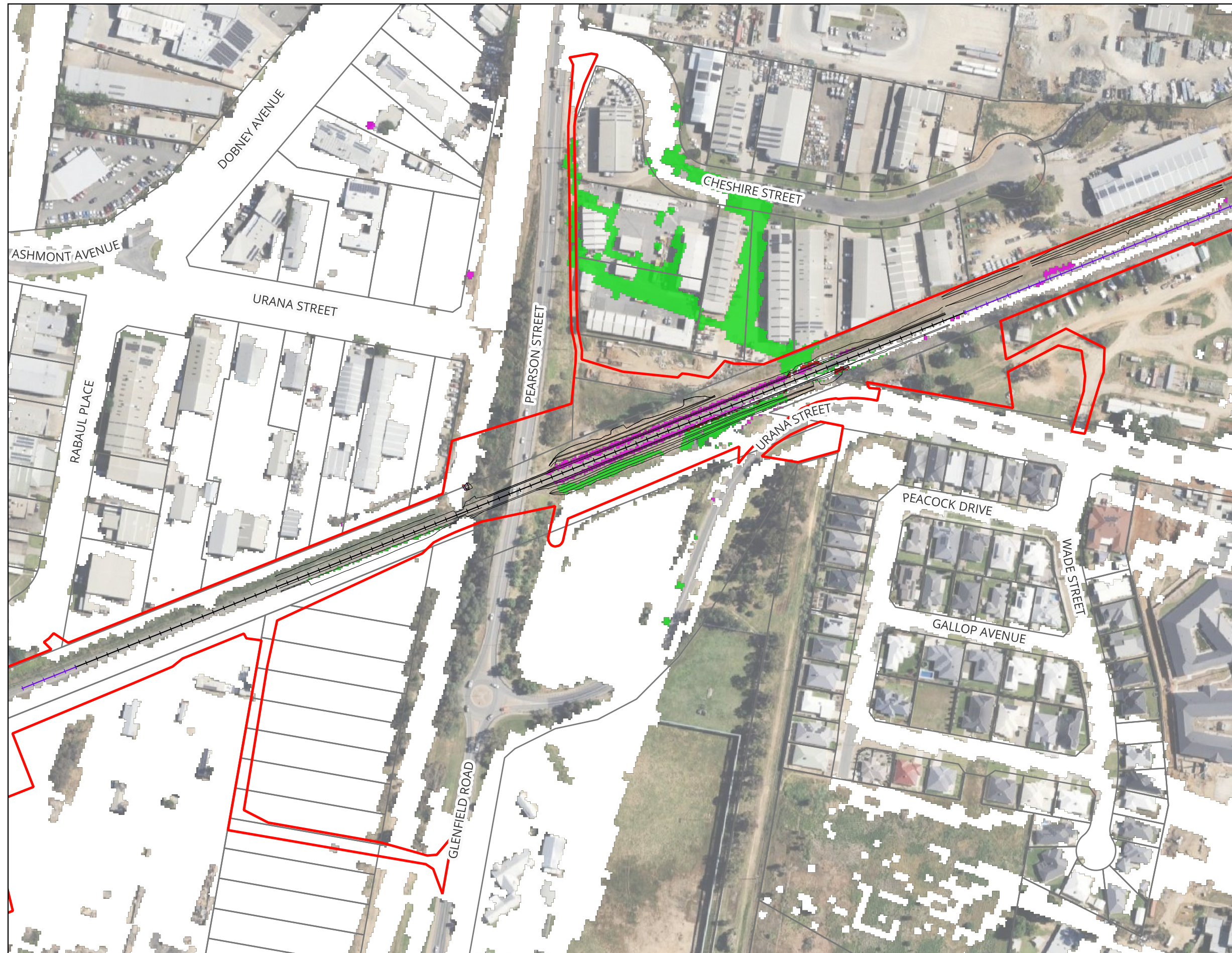
Figure A44 : Changes in Peak Flood Velocity for 2% AEP - Master Design Condition vs Existing Condition
