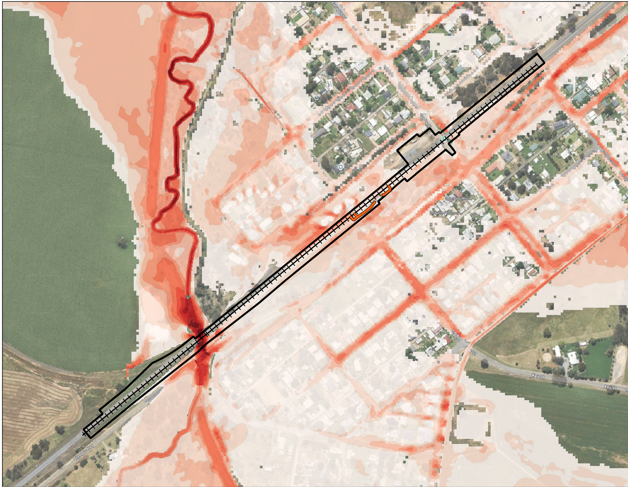
Figure A53 : 1% AEP Peak Flood Velocity - Blockage Assessment
