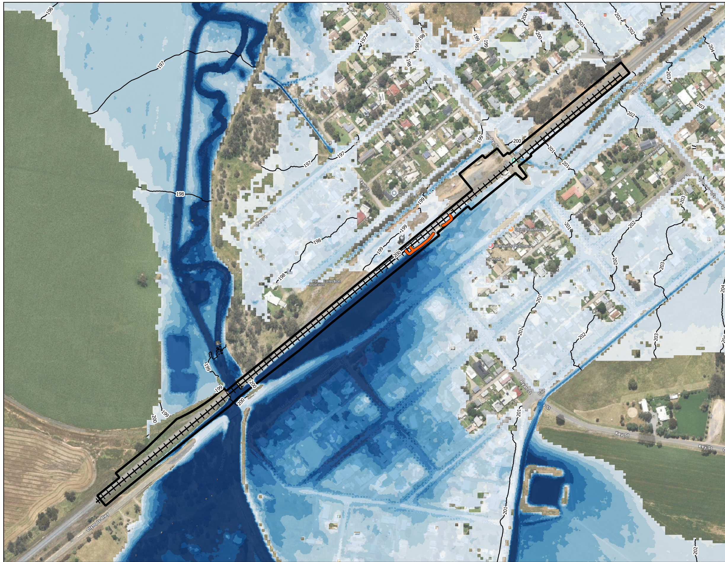
Figure A20 : 2% AEP Peak Flood Depth and Levels - Design Condition
