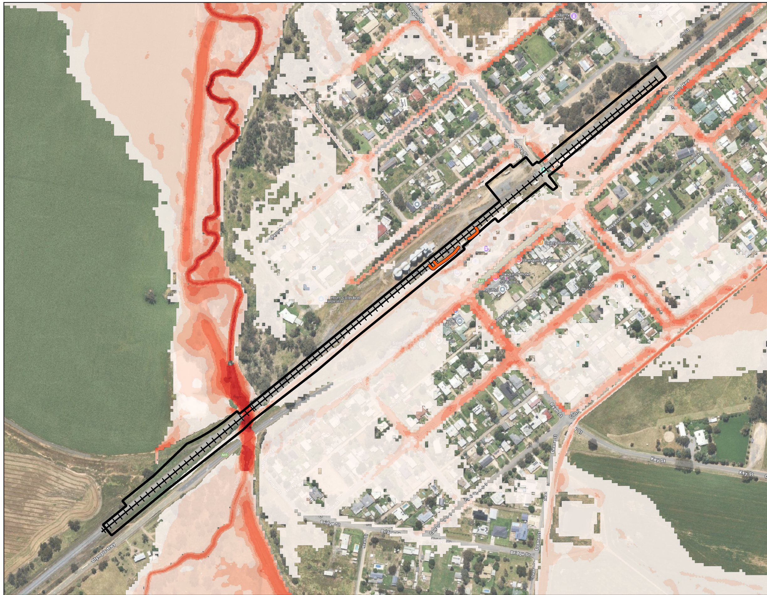
Uranquinty Yard - Inland Rail (A2P) - IFC Stage Figure A25 : 5% AEP Peak Flood Velocity - Design Condition
