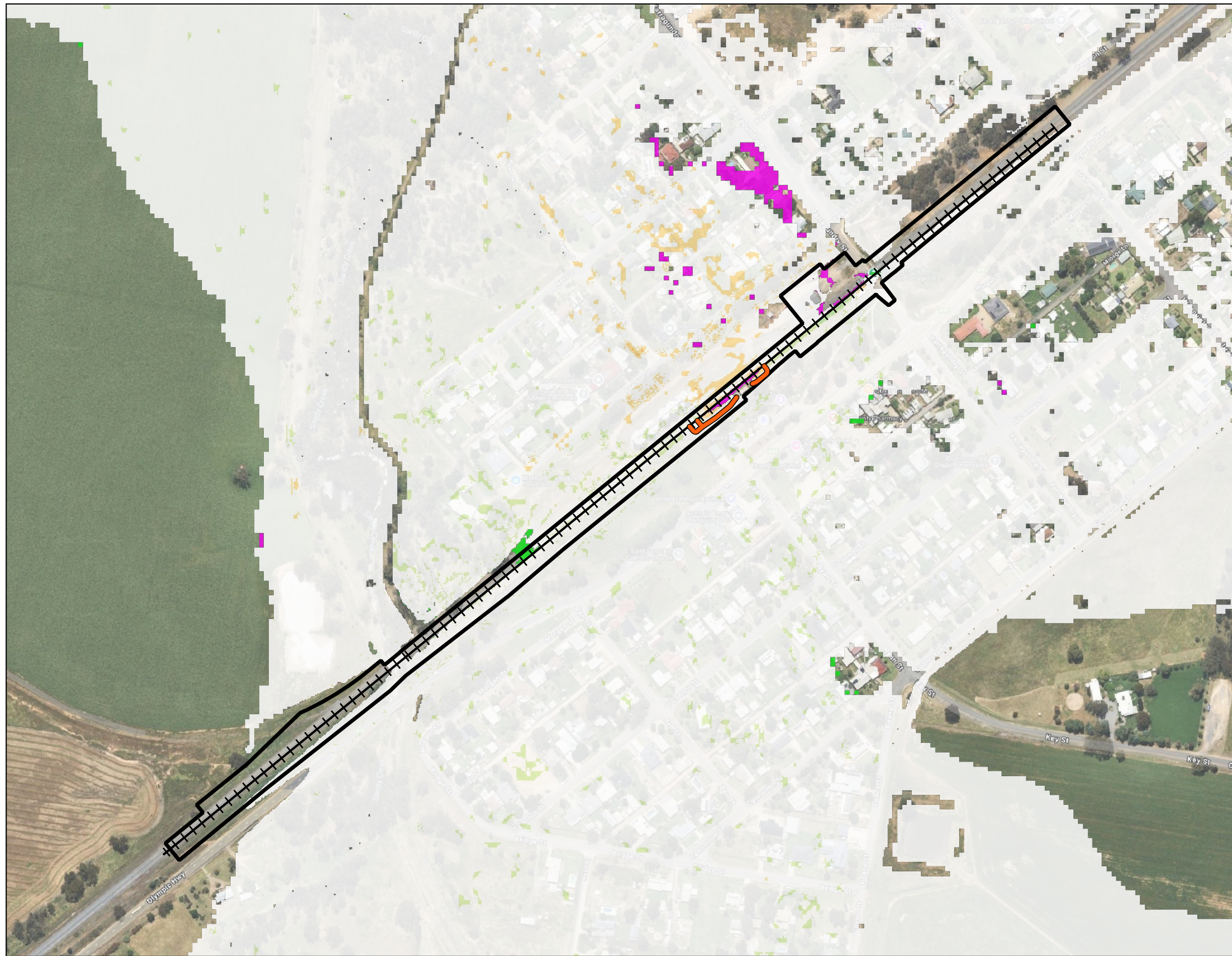
Figure A51 : 0.2% AEP (Climate Change Scenario 2) Changes in Peak Flood Hazard - Design Condition vs Existing Condition
