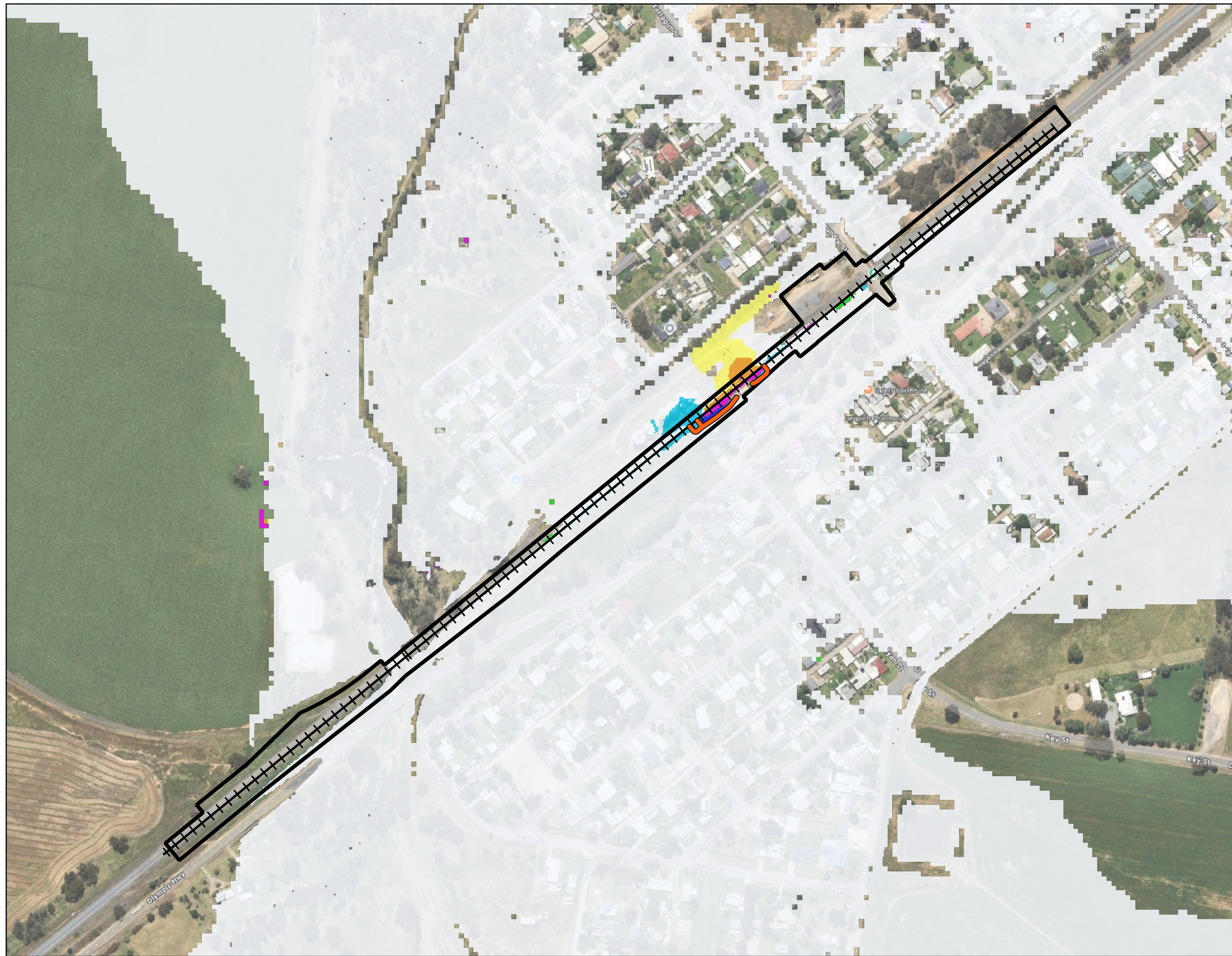
Figure A39 : 1% AEP Changes in Peak Flood Levels - Design Condition vs Existing Condition
