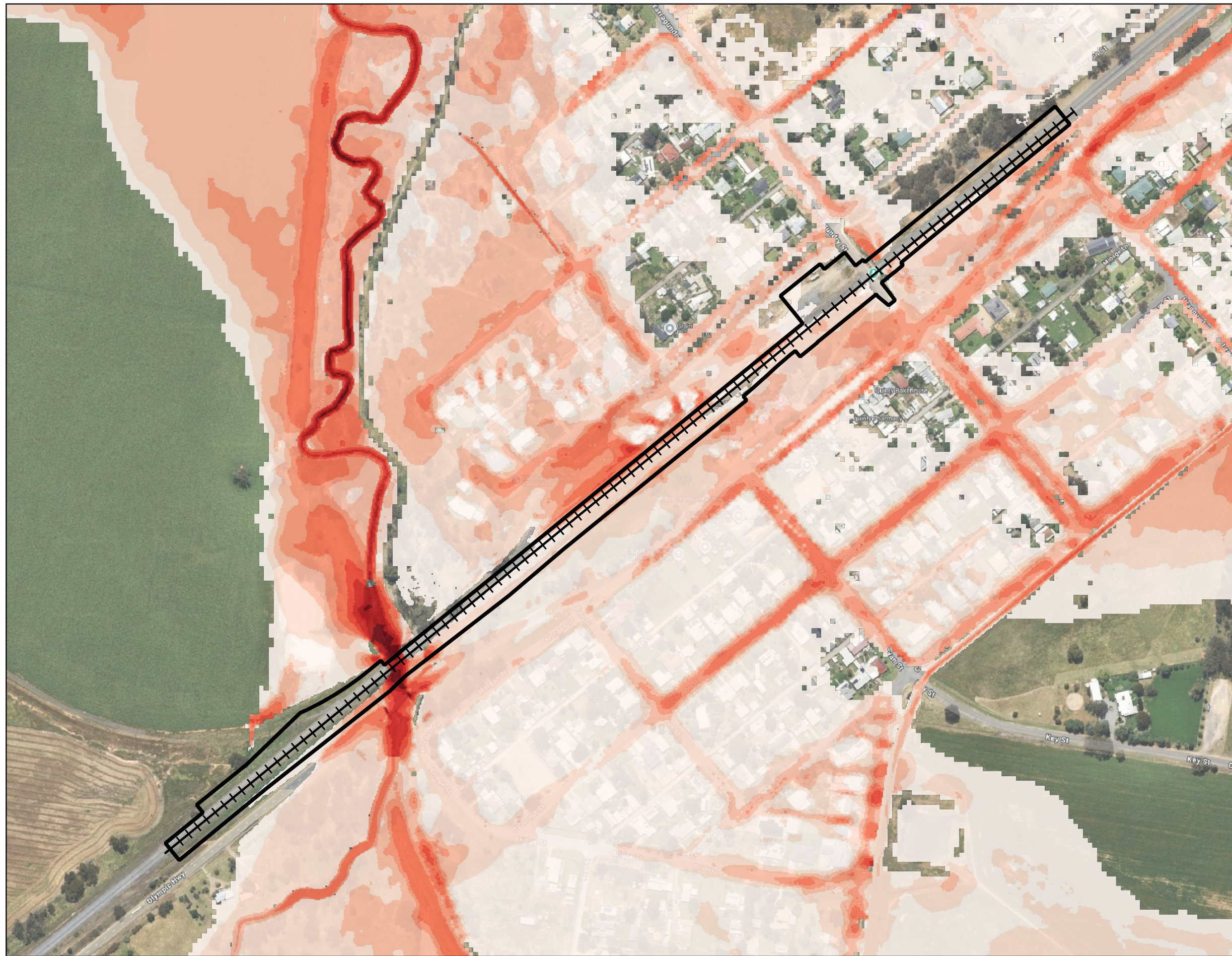
Figure A10 : 0.5% AEP (Climate Change Scenario 1) Peak Flood Velocity - Existing Condition
