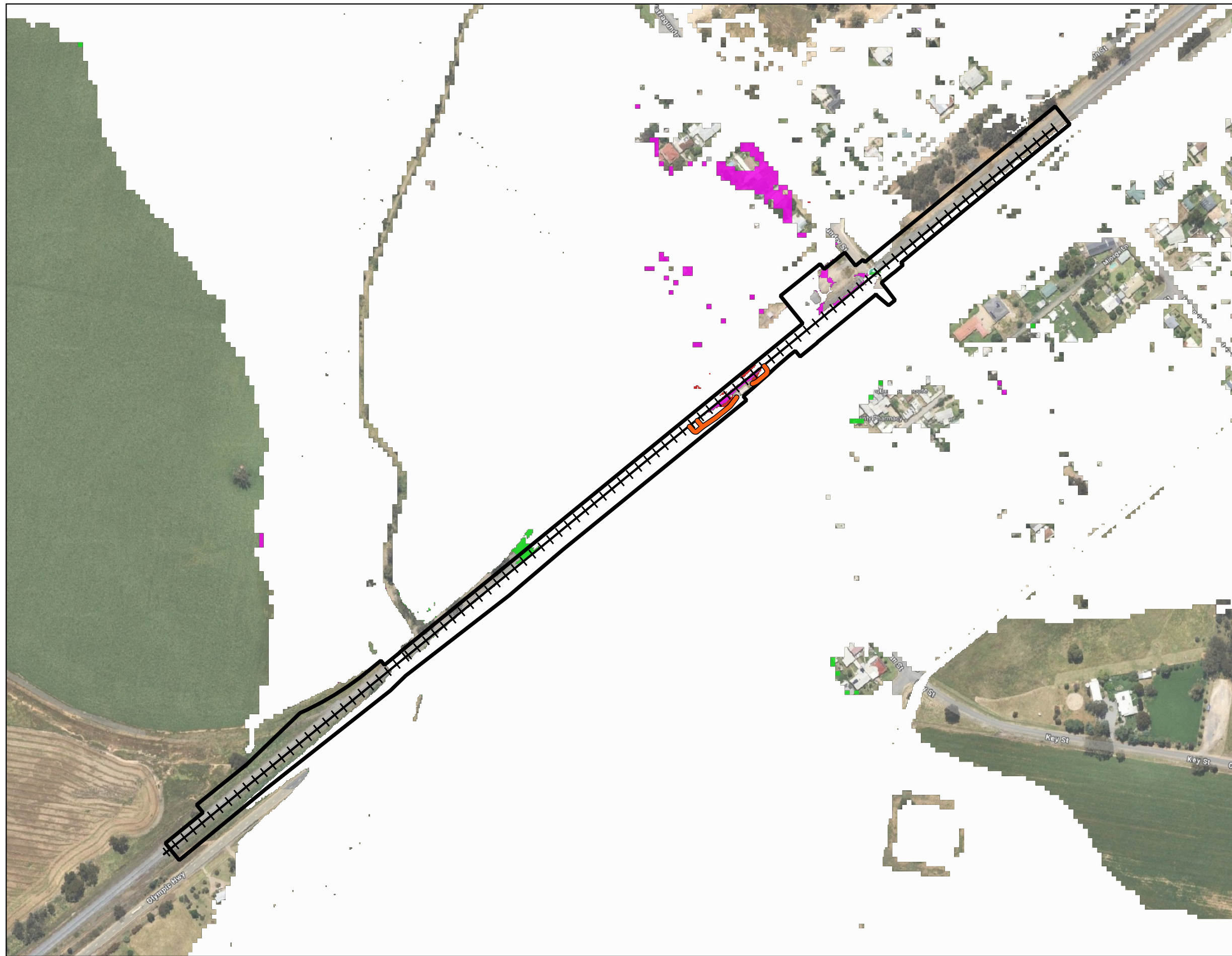
Figure A46 : 0.2% AEP (Climate Change Scenario 2) Changes in Peak Flood Velocity - Design Condition vs Existing Condition
