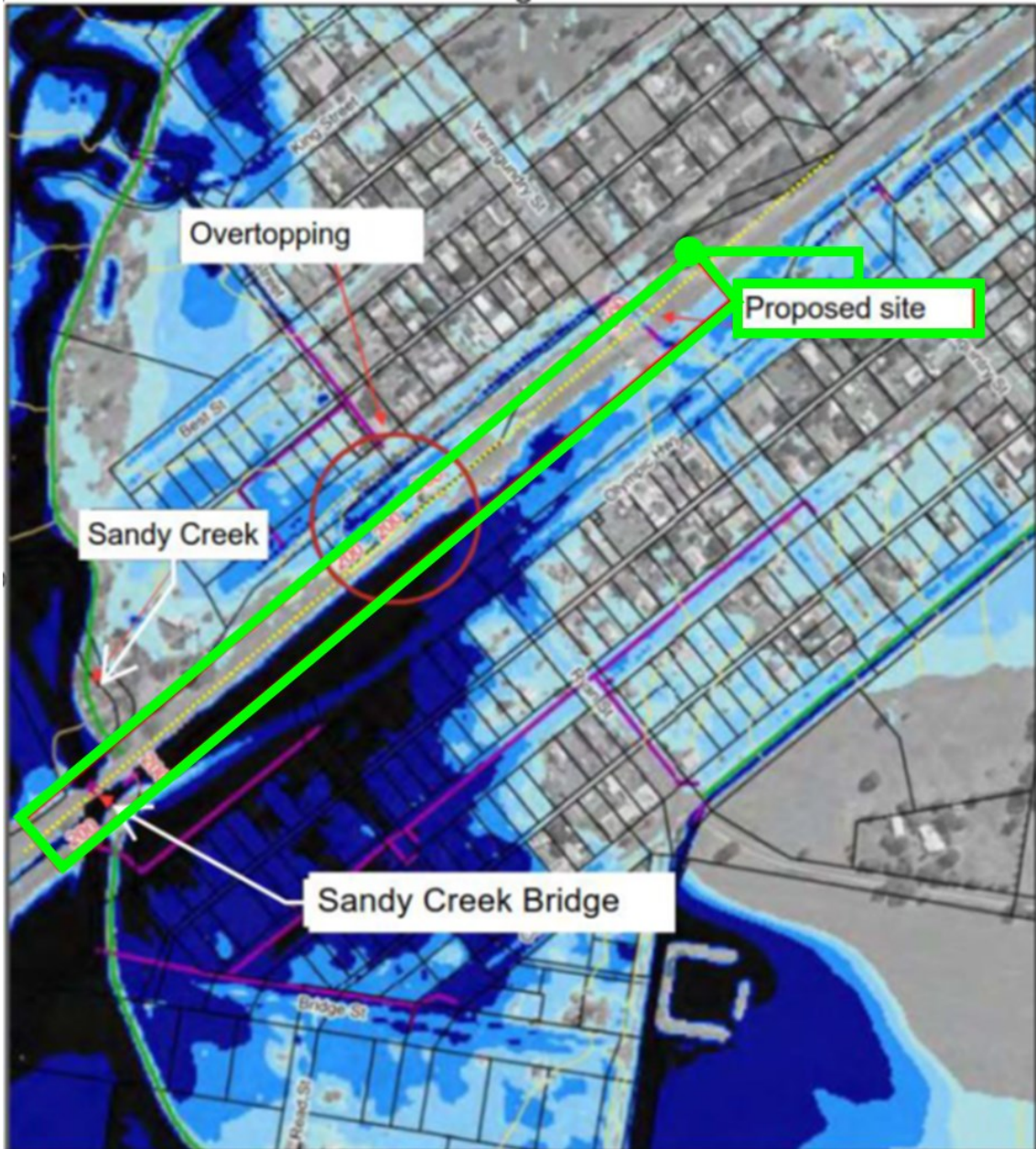
Figure 1-2: 1% AEP Regional Flooding (Image source: A2I and S2P Projects Reference Design Report - Wagga Wagga (June 2022))
