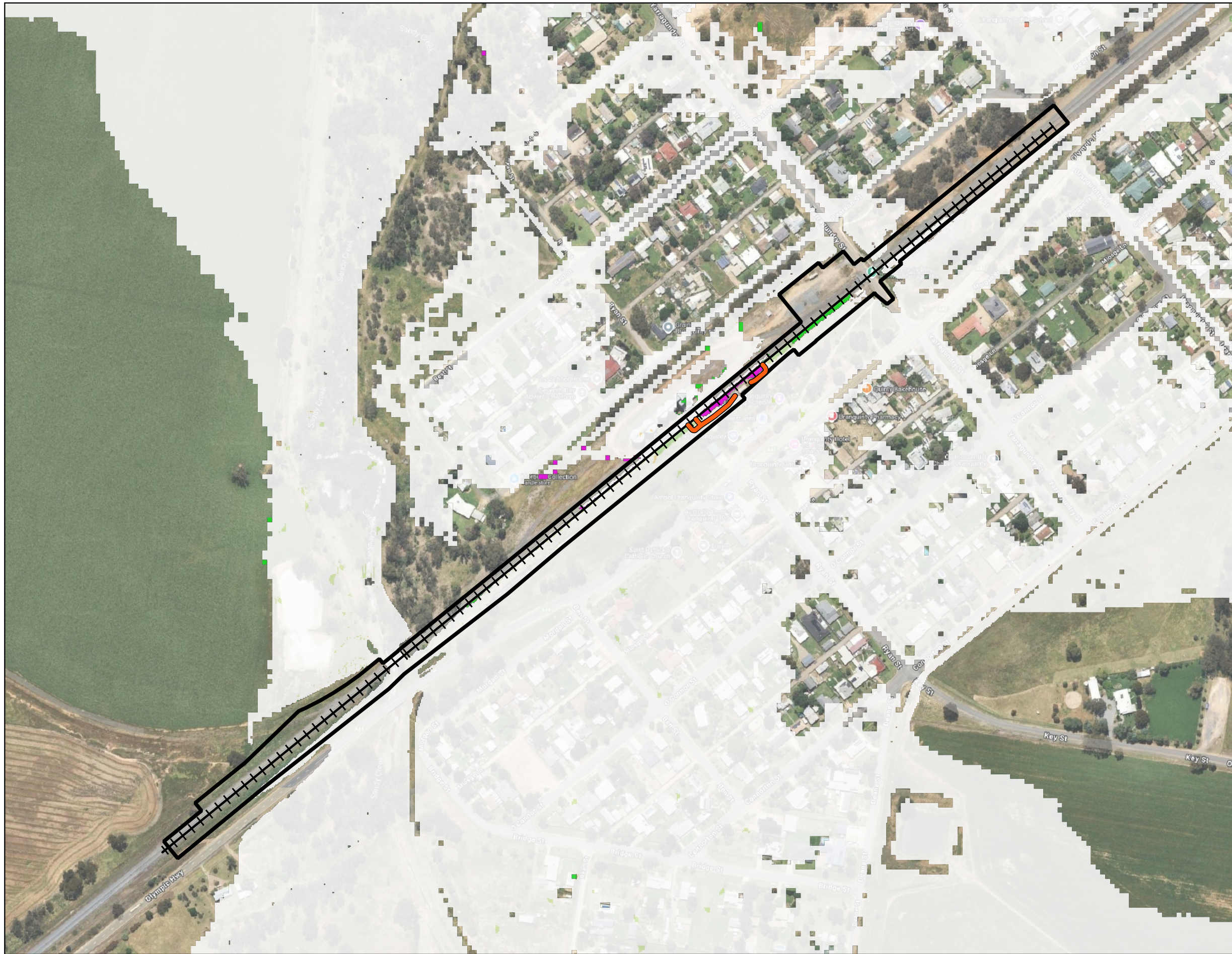
Figure A48 : 2% AEP Changes in Peak Flood Hazard - Design Condition vs Existing Condition
