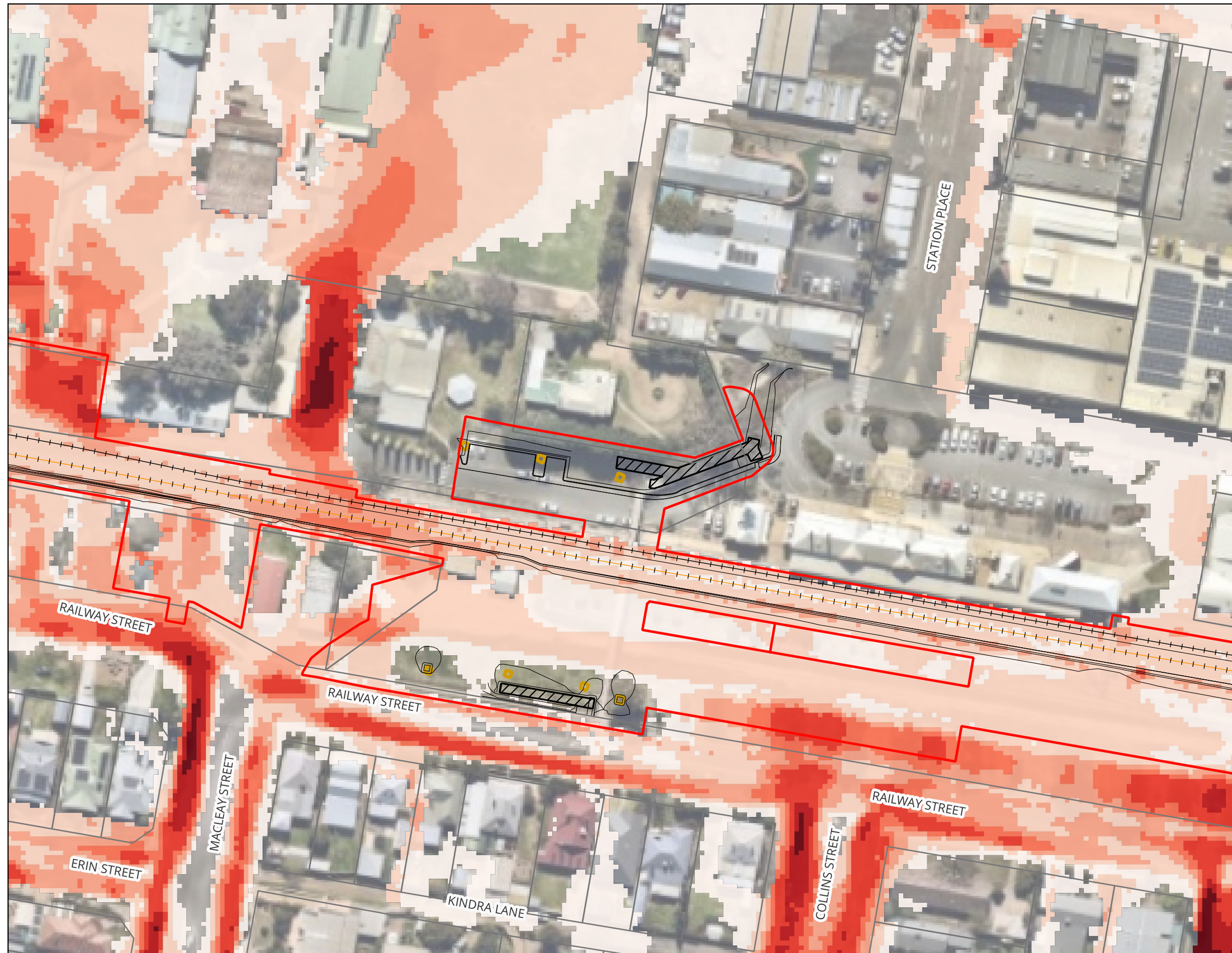
Wagga Mothers Footbridge - Inland Rail (A2P) - IFC Stage Figure A34 : 0.05% AEP Peak Flood Velocity - Master Design Condition
