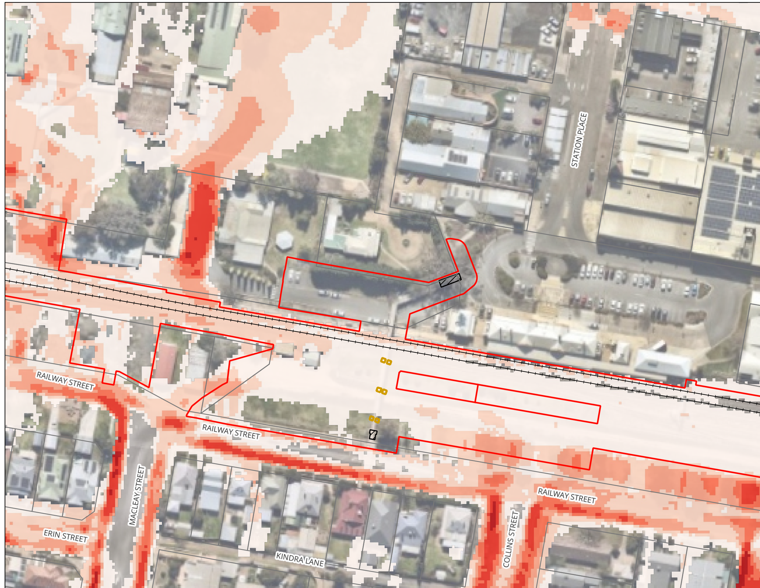
Wagga Mothers Footbridge - Inland Rail (A2P) - IFC Stage Figure A10 : 2% AEP Peak Flood Velocity - Existing Condition
