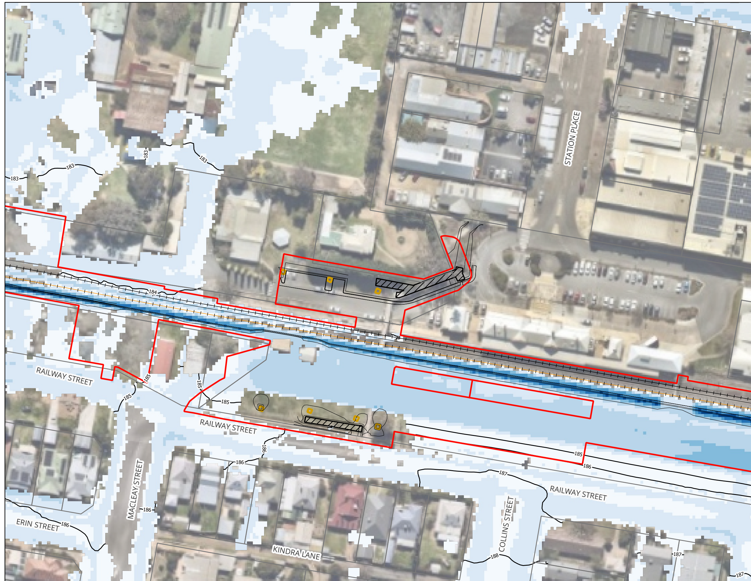
Figure A23 : 5% AEP Peak Flood Depth and Levels - Master Design Condition
