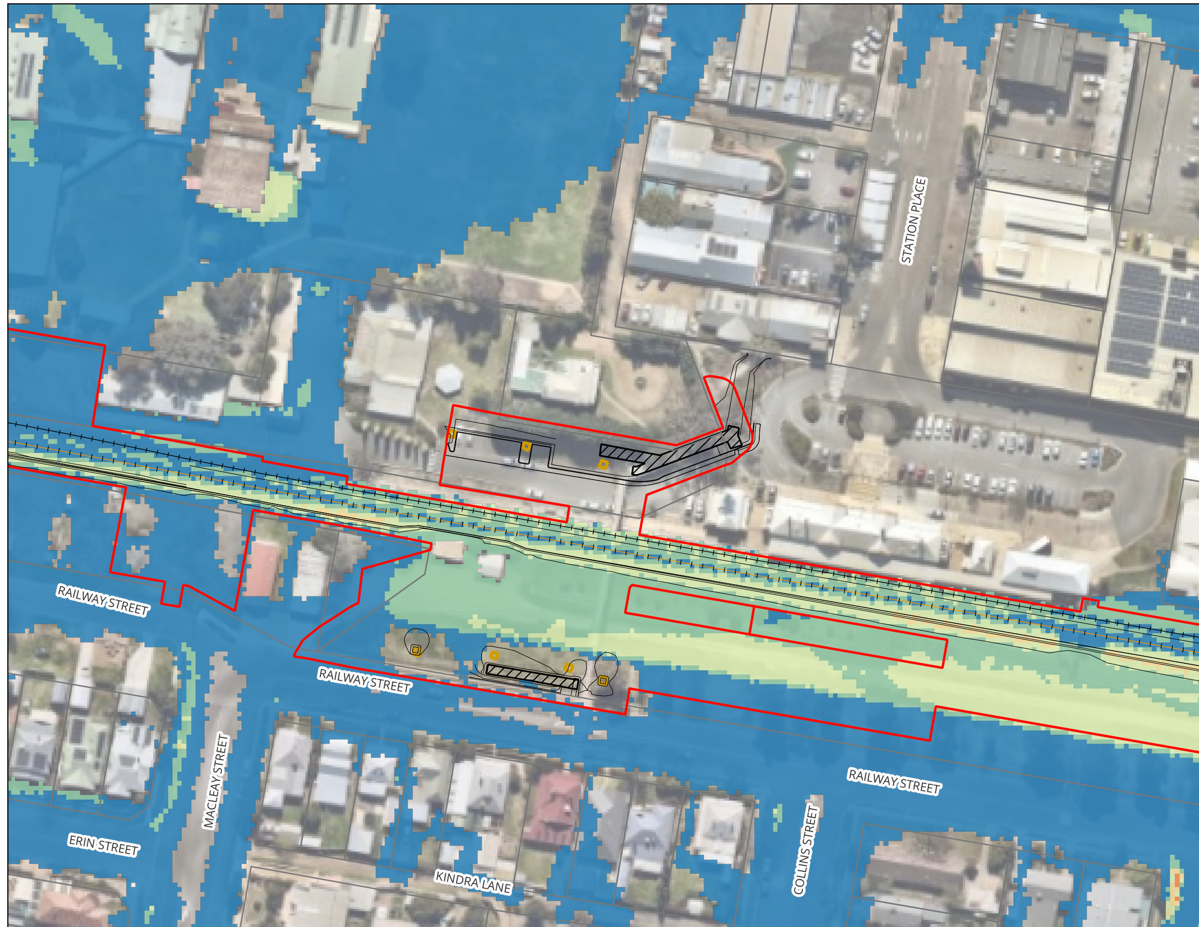
Figure A40 : 1% AEP Climate Changes Peak Flood Hazard - Master Design Condition
