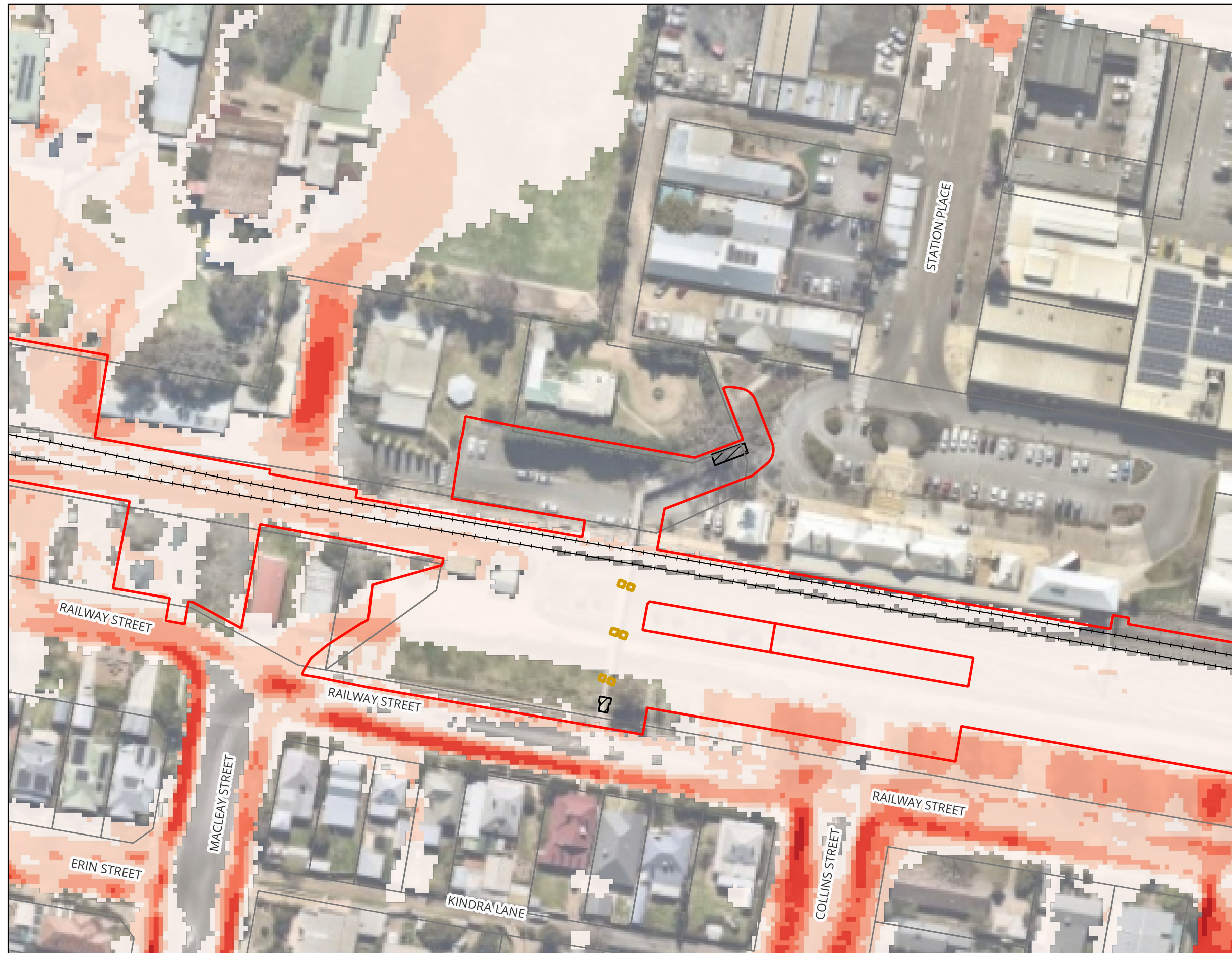
Wagga Mothers Footbridge - Inland Rail (A2P) - IFC Stage Figure A09 : 5% AEP Peak Flood Velocity - Existing Condition
