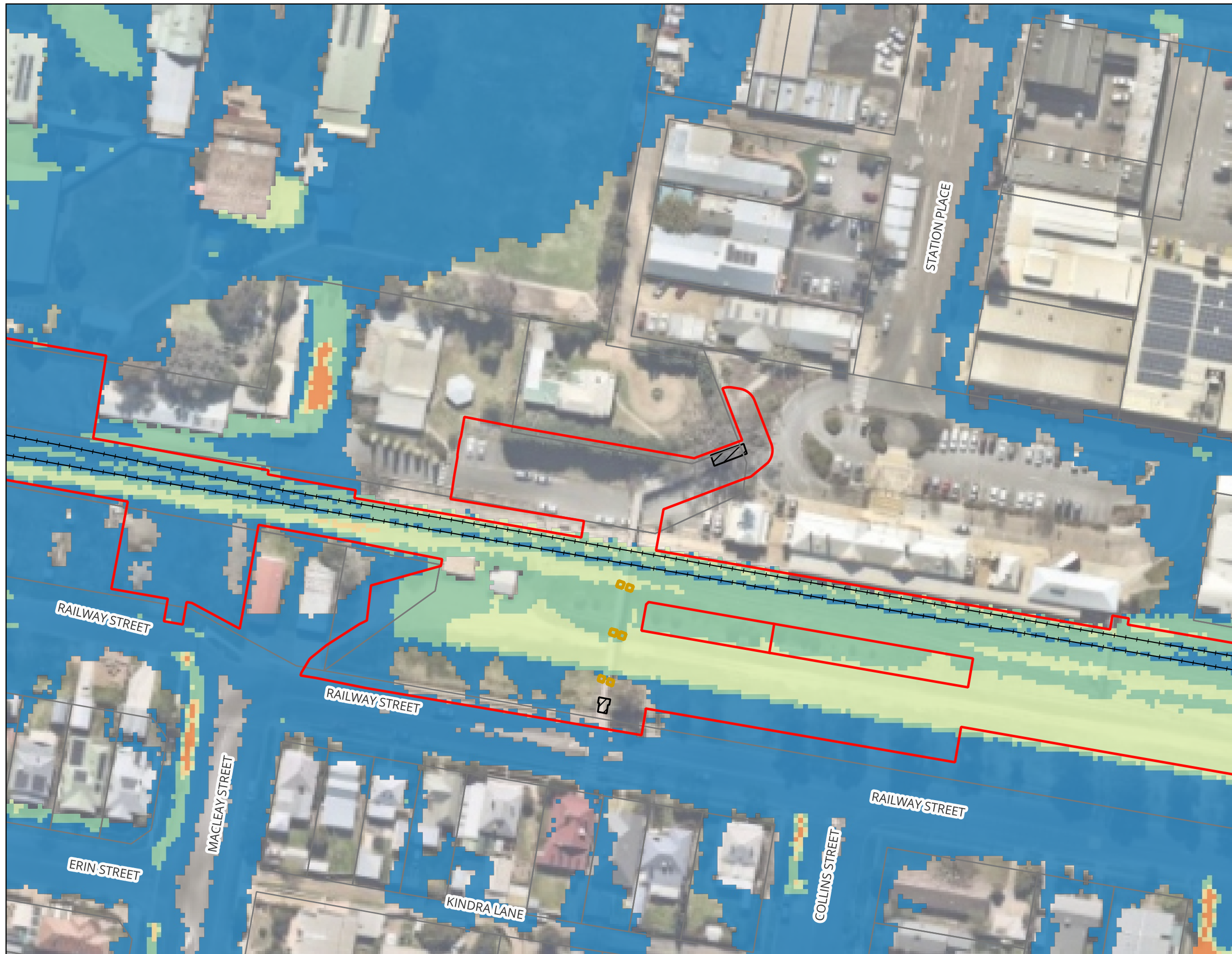
Wagga Mothers Footbridge - Inland Rail (A2P) - IFC Stage Figure A20 : 0.05% AEP Peak Flood Hazard - Existing Condition
