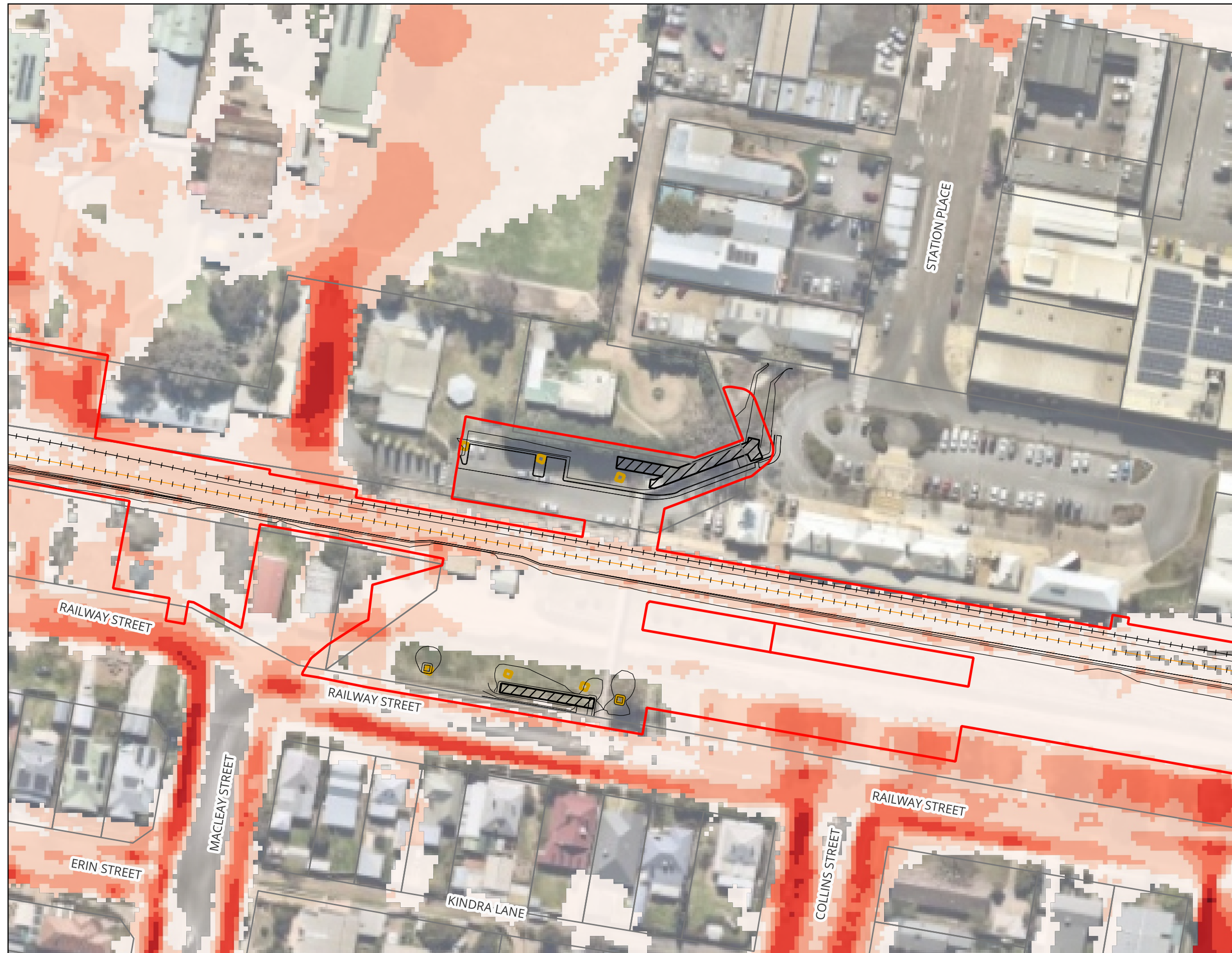
Wagga Mothers Footbridge - Inland Rail (A2P) - IFC Stage Figure A32 : 1% AEP Peak Flood Velocity - Master Design Condition
