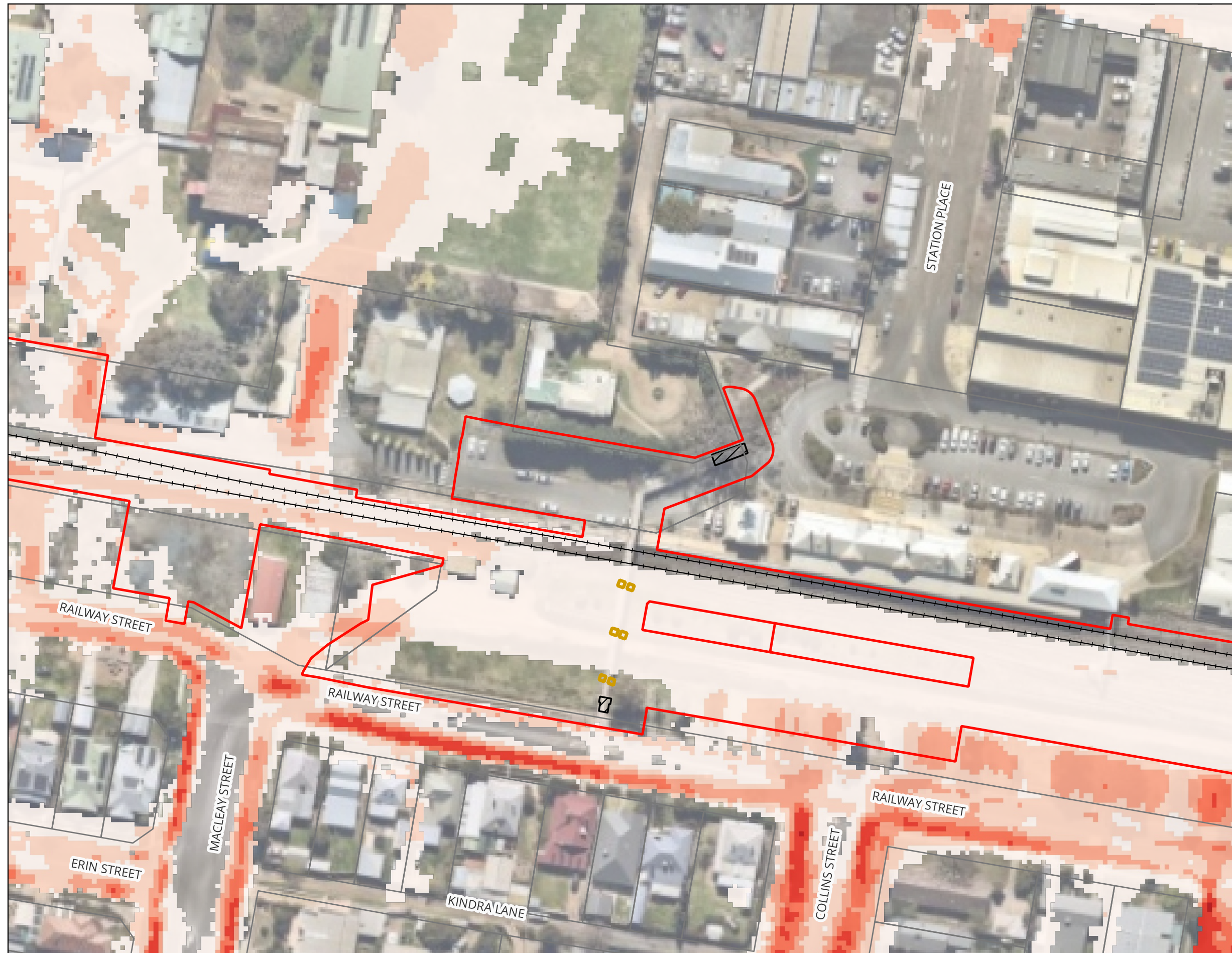
Wagga Mothers Footbridge - Inland Rail (A2P) - IFC Stage Figure A08 : 10% AEP Peak Flood Velocity - Existing Condition
