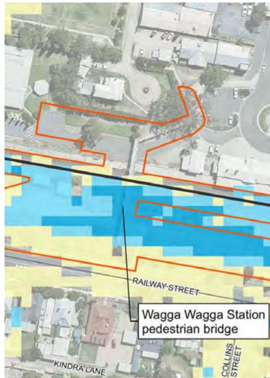
Figure 1-3: 1% AEP Local Flooding for Wagga Wagga Station Pedestrian bridge (Wagga Mothers Footbridge) (Image source: Albury to Illabo EIS Technical Paper 11 (July 2022))
