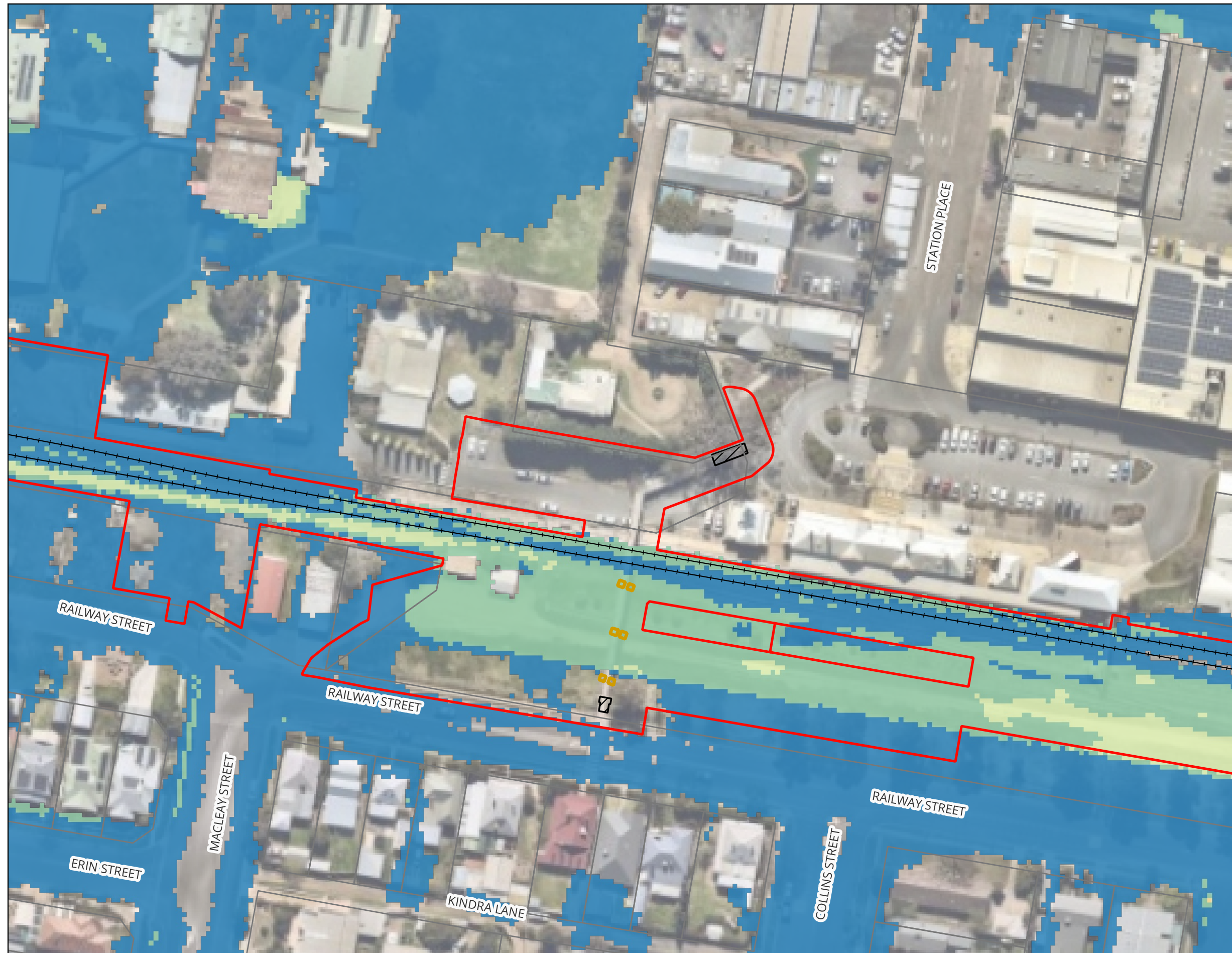
Wagga Mothers Footbridge - Inland Rail (A2P) - IFC Stage Figure A18 : 1% AEP Peak Flood Hazard - Existing Condition
