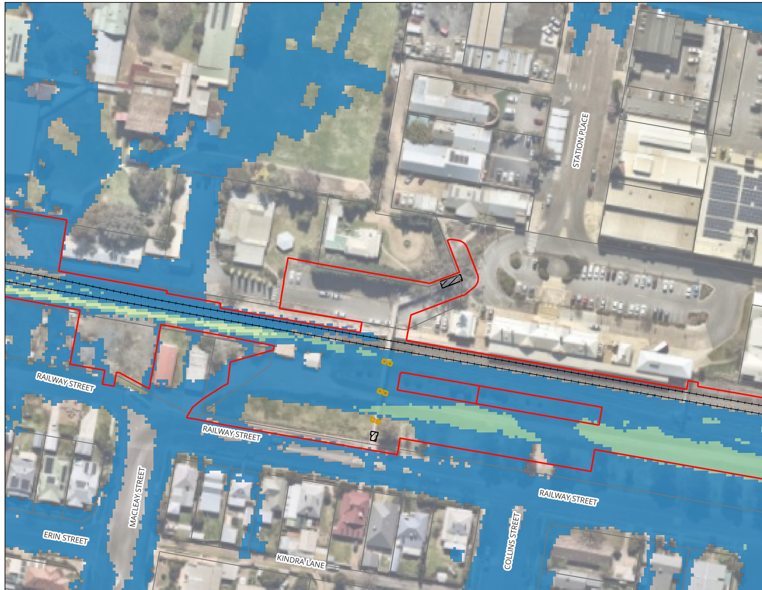
Wagga Mothers Footbridge - Inland Rail (A2P) - IFC Stage Figure A15 : 10% AEP Peak Flood Hazard - Existing Condition
