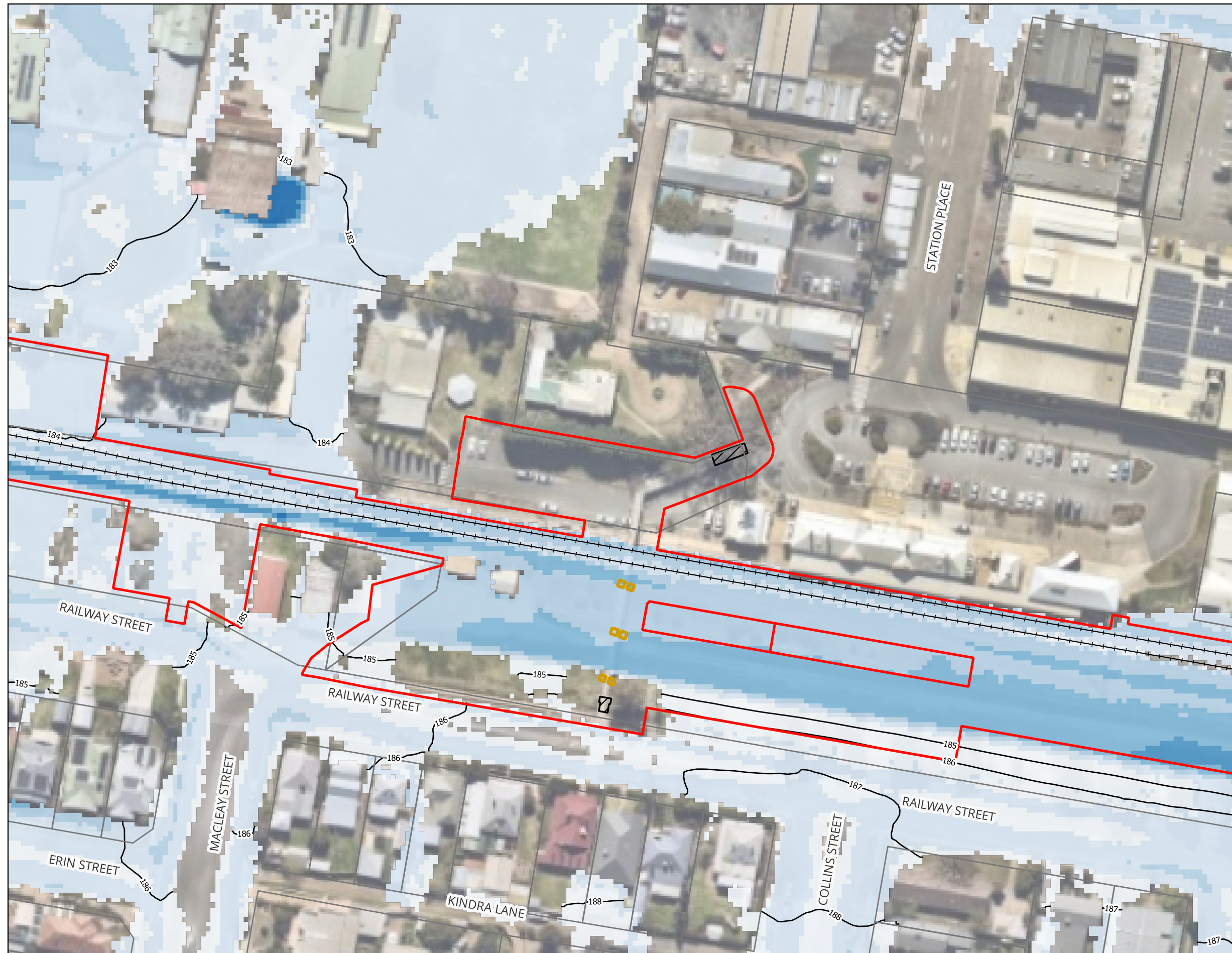
Figure A04 : 1% AEP Peak Flood Depth and Levels - Existing Condition
