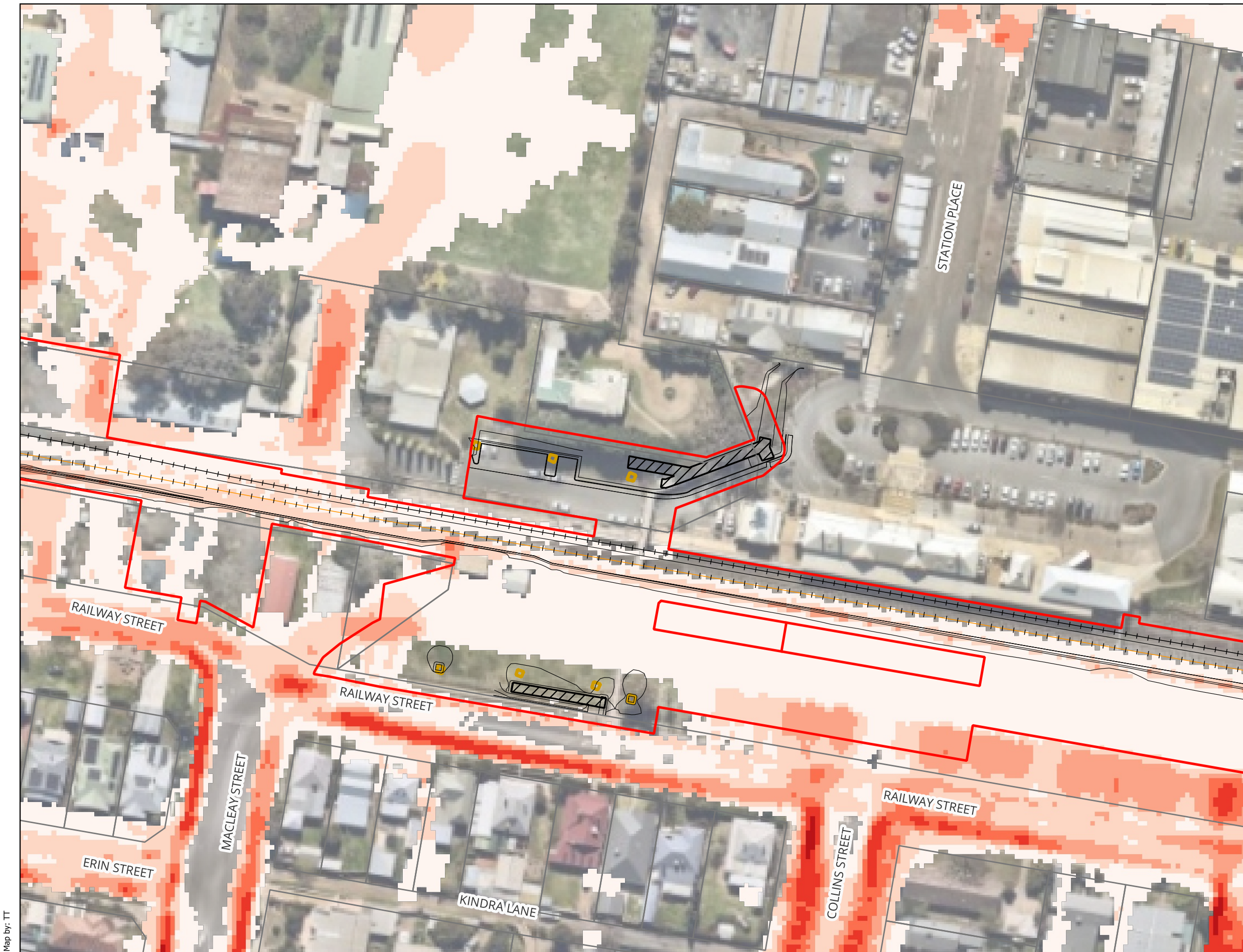
Wagga Mothers Footbridge - Inland Rail (A2P) - IFC Stage Figure A30 : 5% AEP Peak Flood Velocity - Master Design Condition
