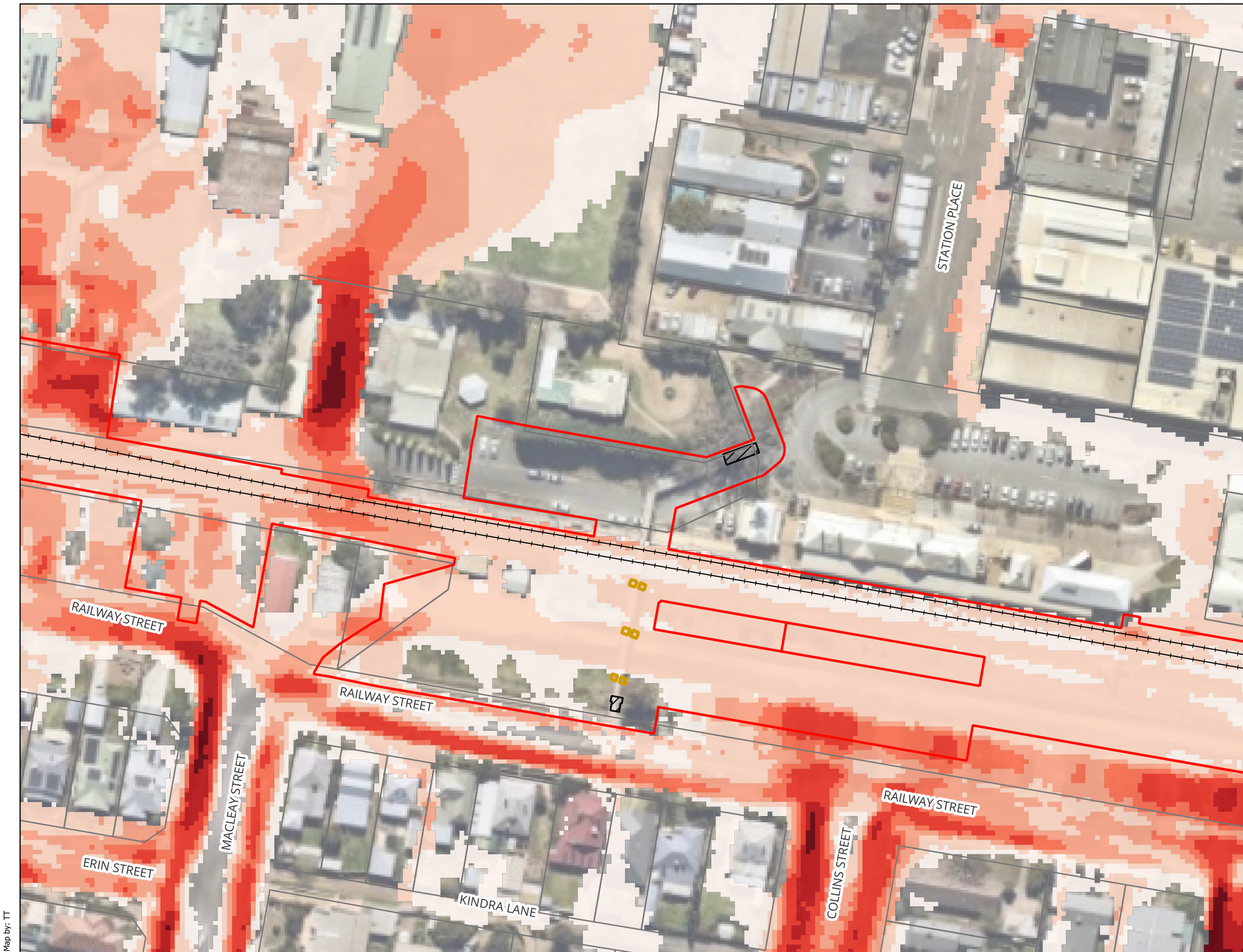
Wagga Mothers Footbridge - Inland Rail (A2P) - IFC Stage Figure A13 : 0.05% AEP Peak Flood Velocity - Existing Condition
