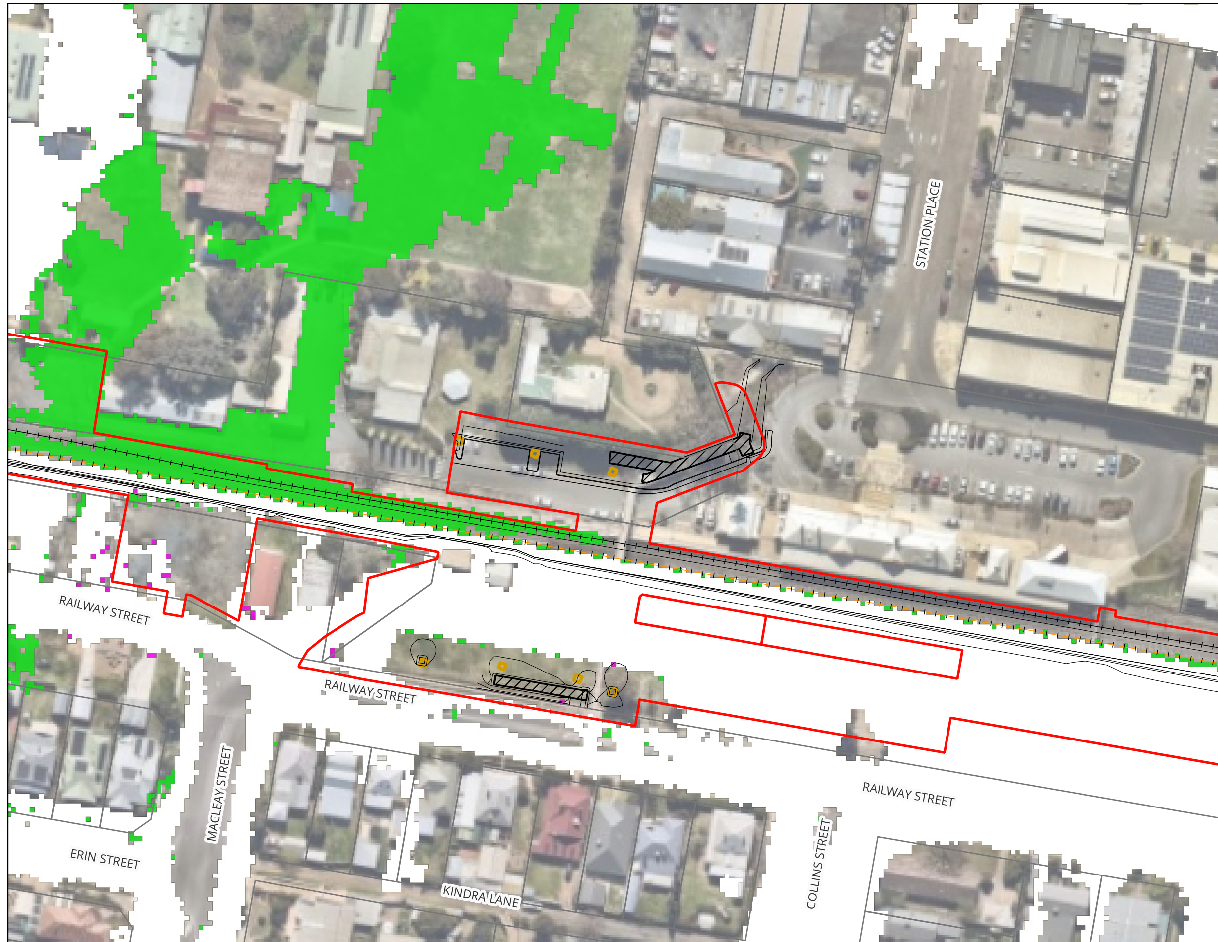
Figure A48 : Changes in Peak Flood Velocity for 10% AEP - Master Design Condition vs Existing Condition
