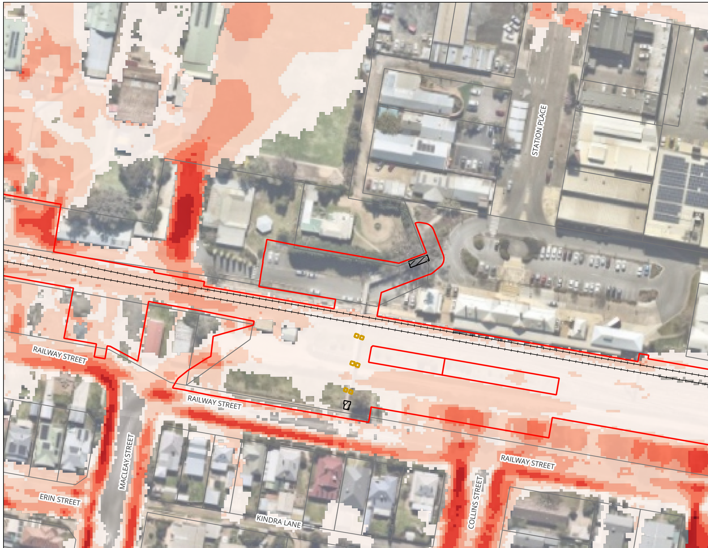
Wagga Mothers Footbridge - Inland Rail (A2P) - IFC Stage Figure A11 : 1% AEP Peak Flood Velocity - Existing Condition
