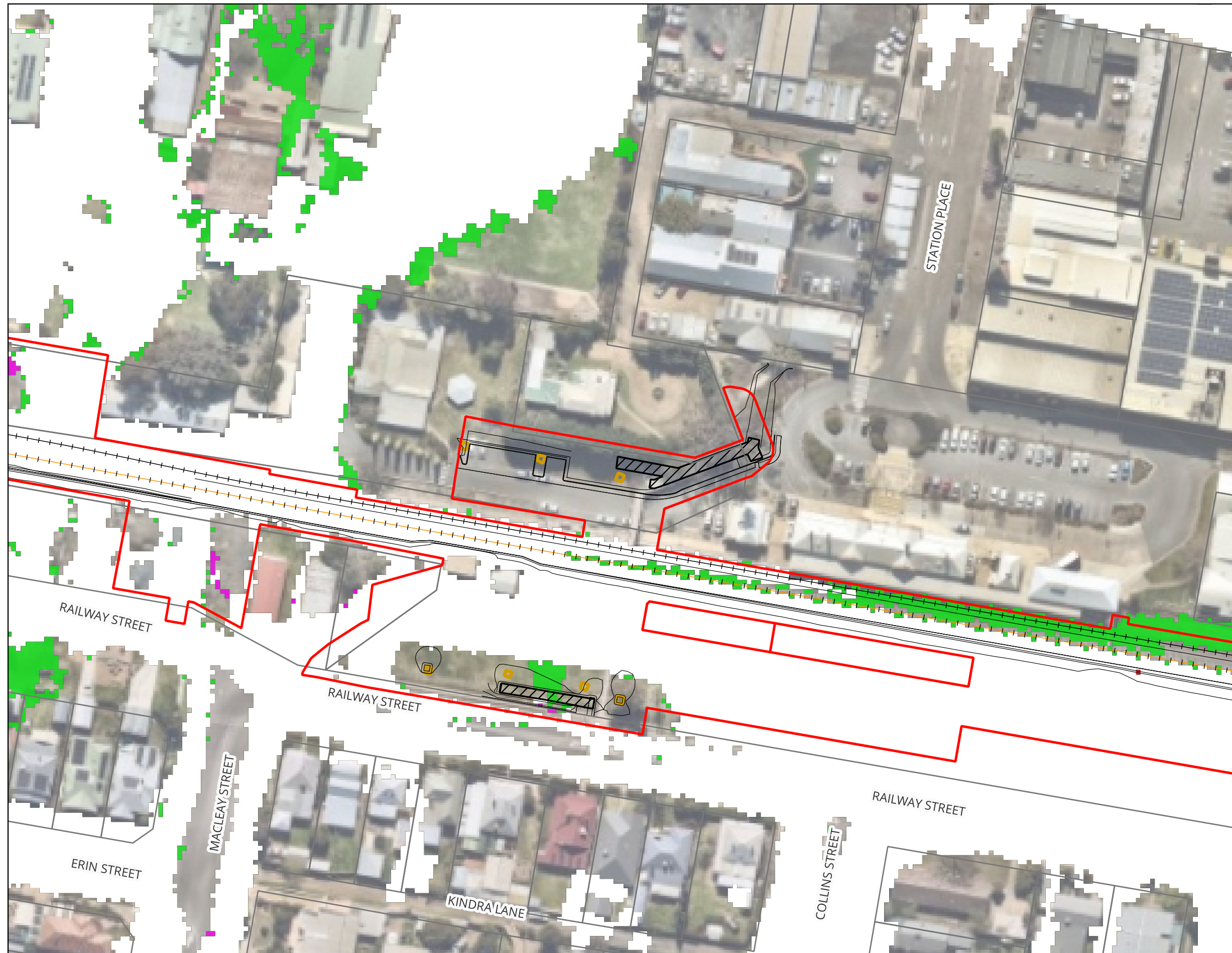
Figure A50 : Changes in Peak Flood Velocity for 2% AEP - Master Design Condition vs Existing Condition
