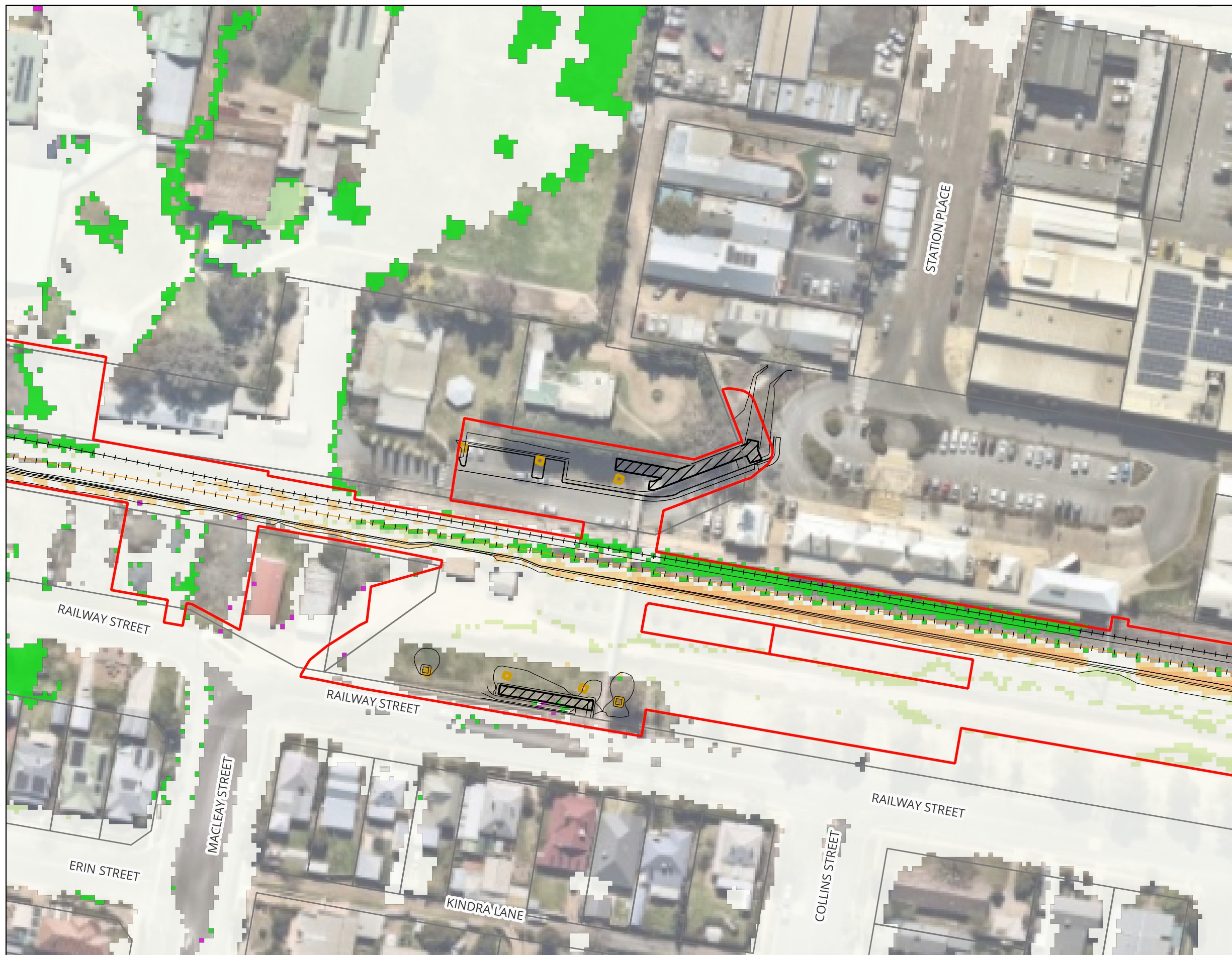
Figure A54 : Changes in Peak Flood Hazard for 5% AEP - Master Design Condition vs Existing Condition
