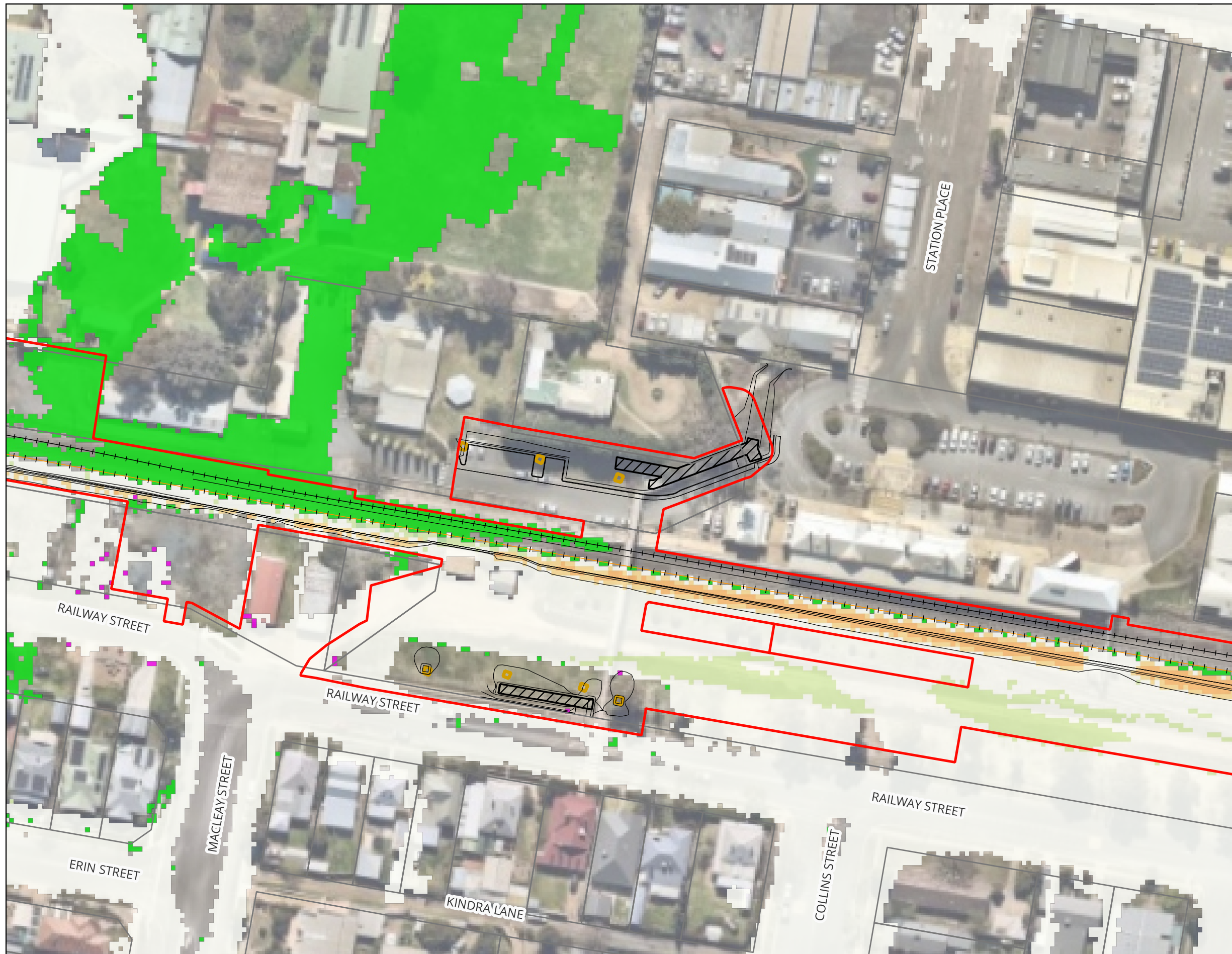
Figure A53 : Changes in Peak Flood Hazard for 10% AEP - Master Design Condition vs Existing Condition
