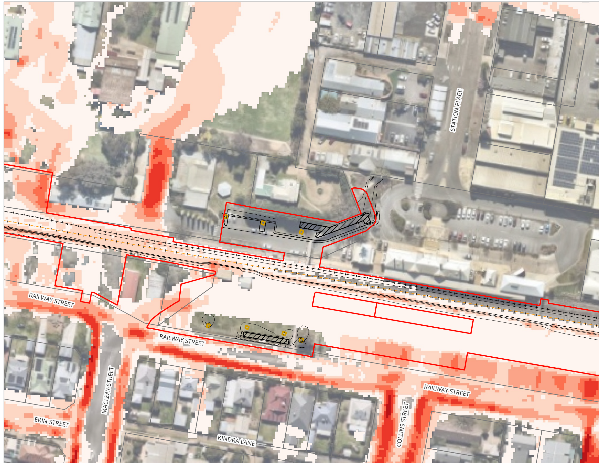
Wagga Mothers Footbridge - Inland Rail (A2P) - IFC Stage Figure A31 : 2% AEP Peak Flood Velocity - Master Design Condition
