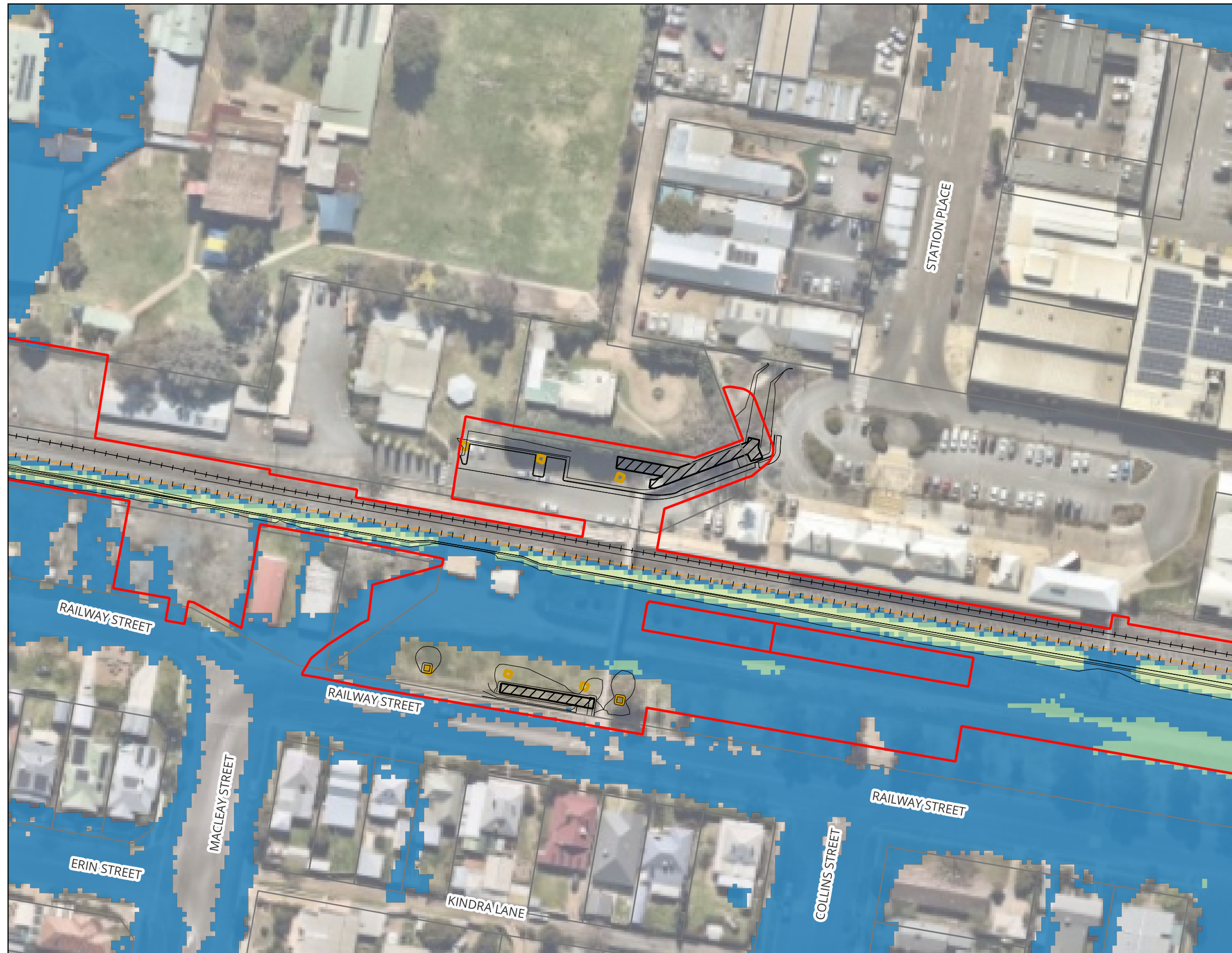
Wagga Mothers Footbridge - Inland Rail (A2P) - IFC Stage Figure A36 : 10% AEP Peak Flood Hazard - Master Design Condition
