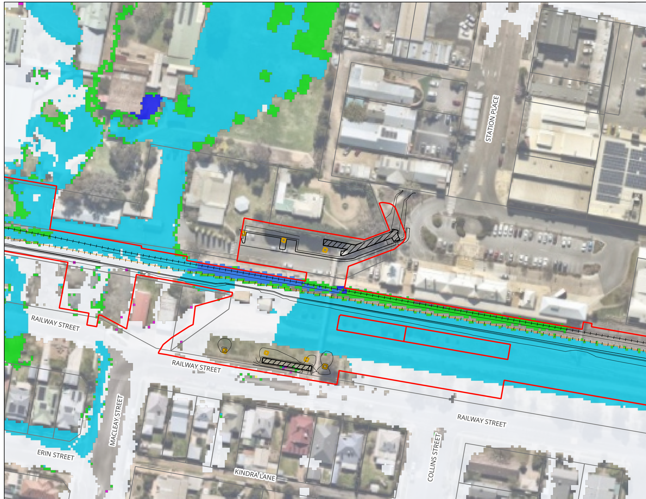
Figure A44 : Changes in Peak Flood Levels for 5% AEP - Master Design Condition vs Existing Condition
