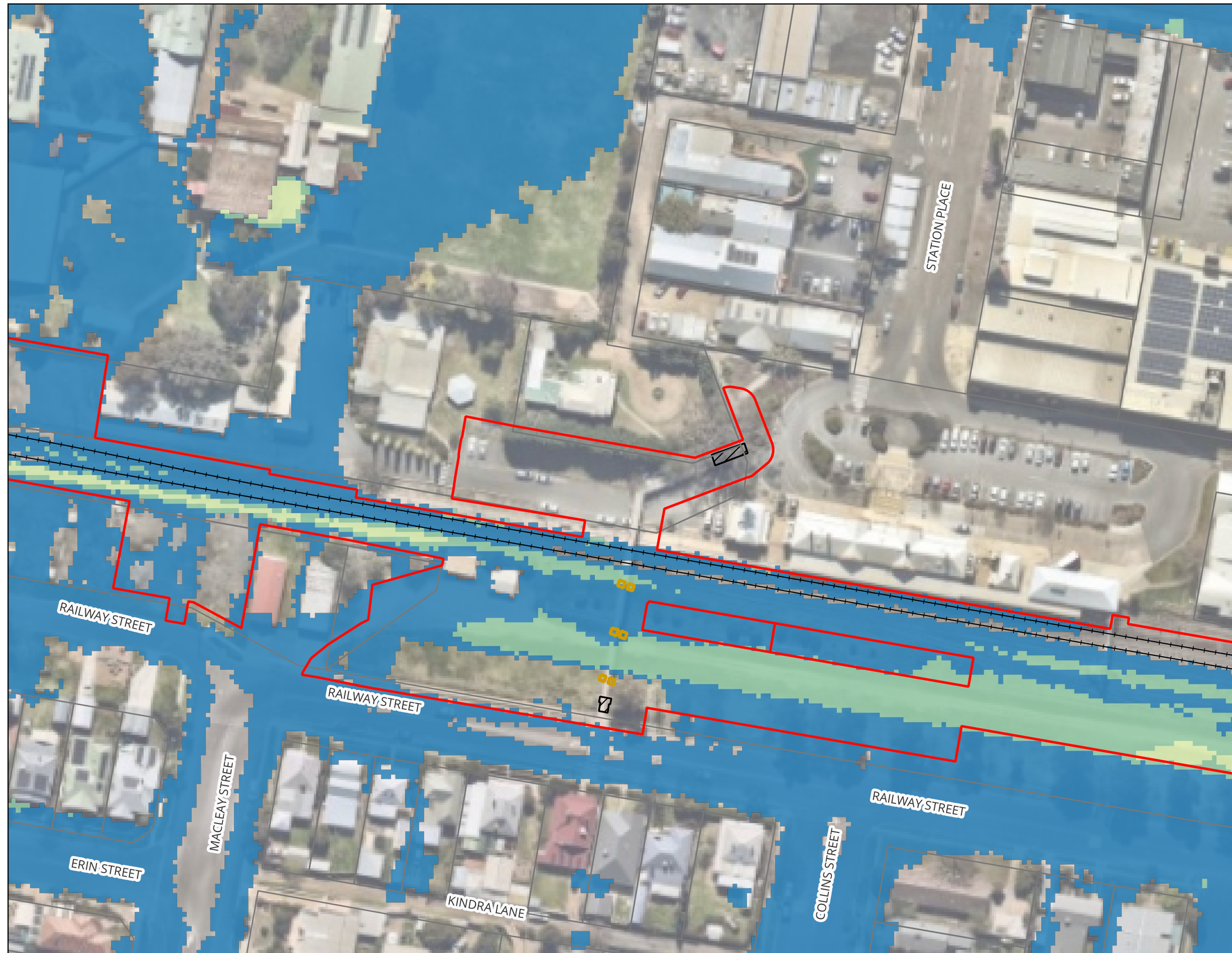
Wagga Mothers Footbridge - Inland Rail (A2P) - IFC Stage Figure A16 : 5% AEP Peak Flood Hazard - Existing Condition
