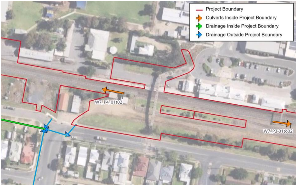
Figure 6-7: Culverts at Wagga Mothers Footbridge Site
