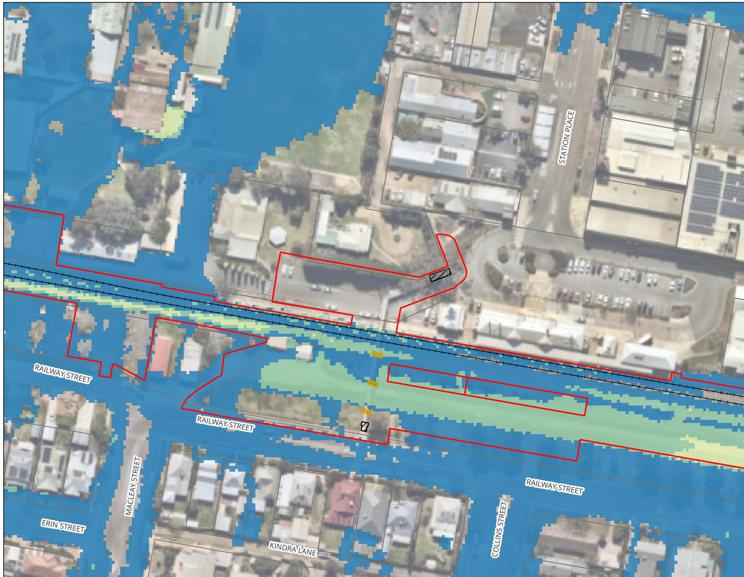
Wagga Mothers Footbridge - Inland Rail (A2P) - IFC Stage Figure A17 : 2% AEP Peak Flood Hazard - Existing Condition
