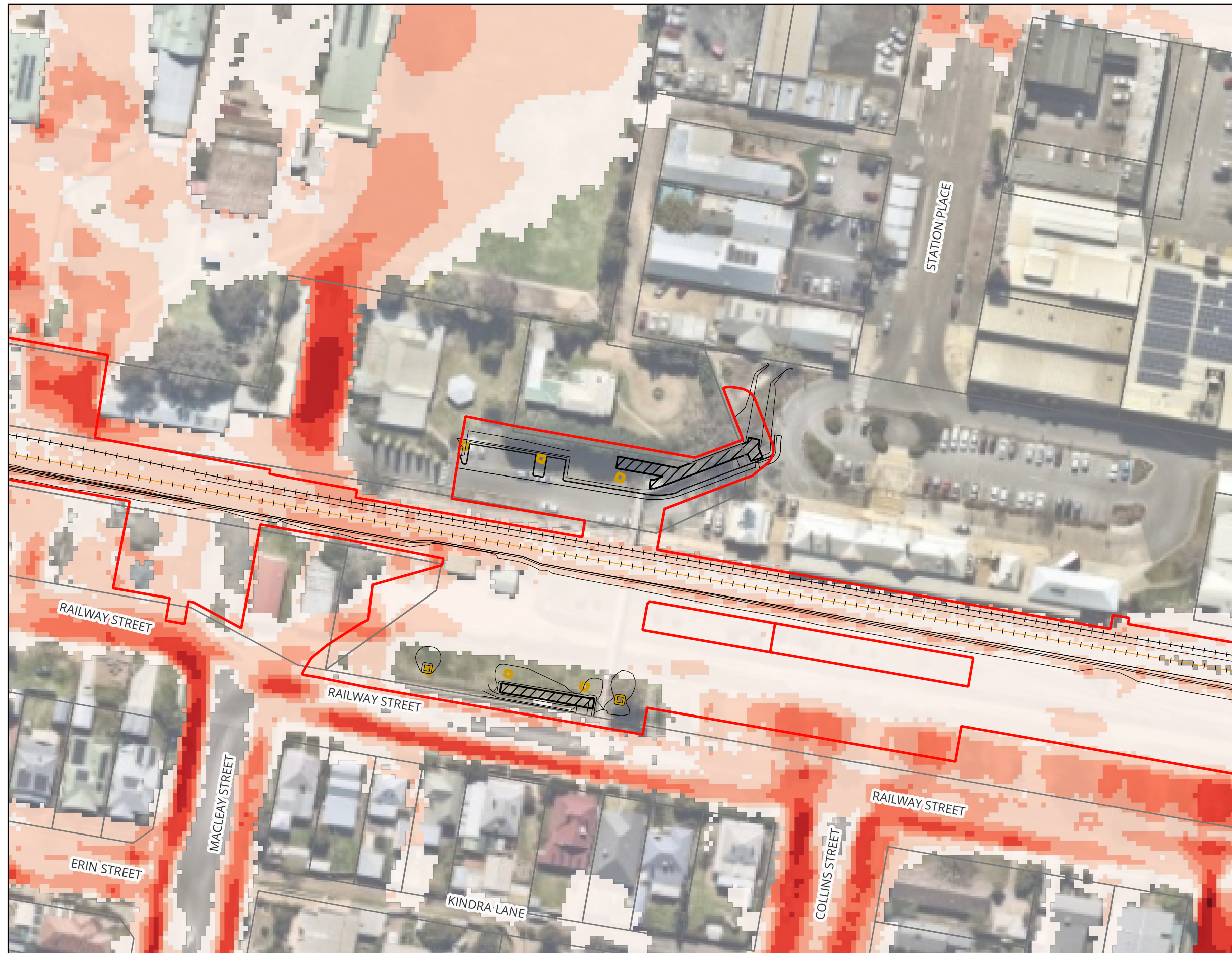
Figure A59 : 1% AEP Peak Flood Velocity - Master Design Blockage Condition
