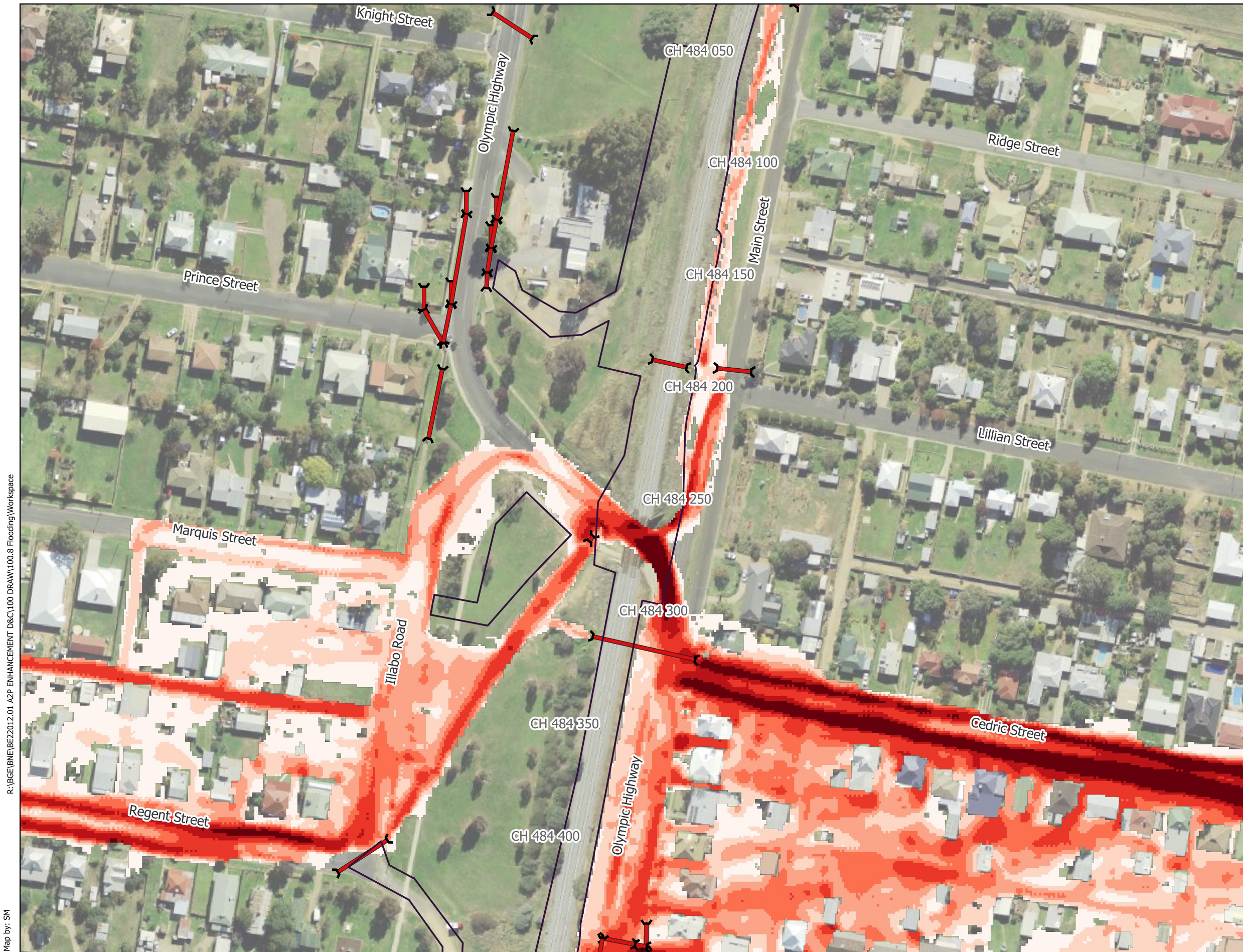
Figure 7c - Olympic Highway Underbridge - IFC Stage 5% AEP Flood Velocity (m/s) - Existing Conditions
