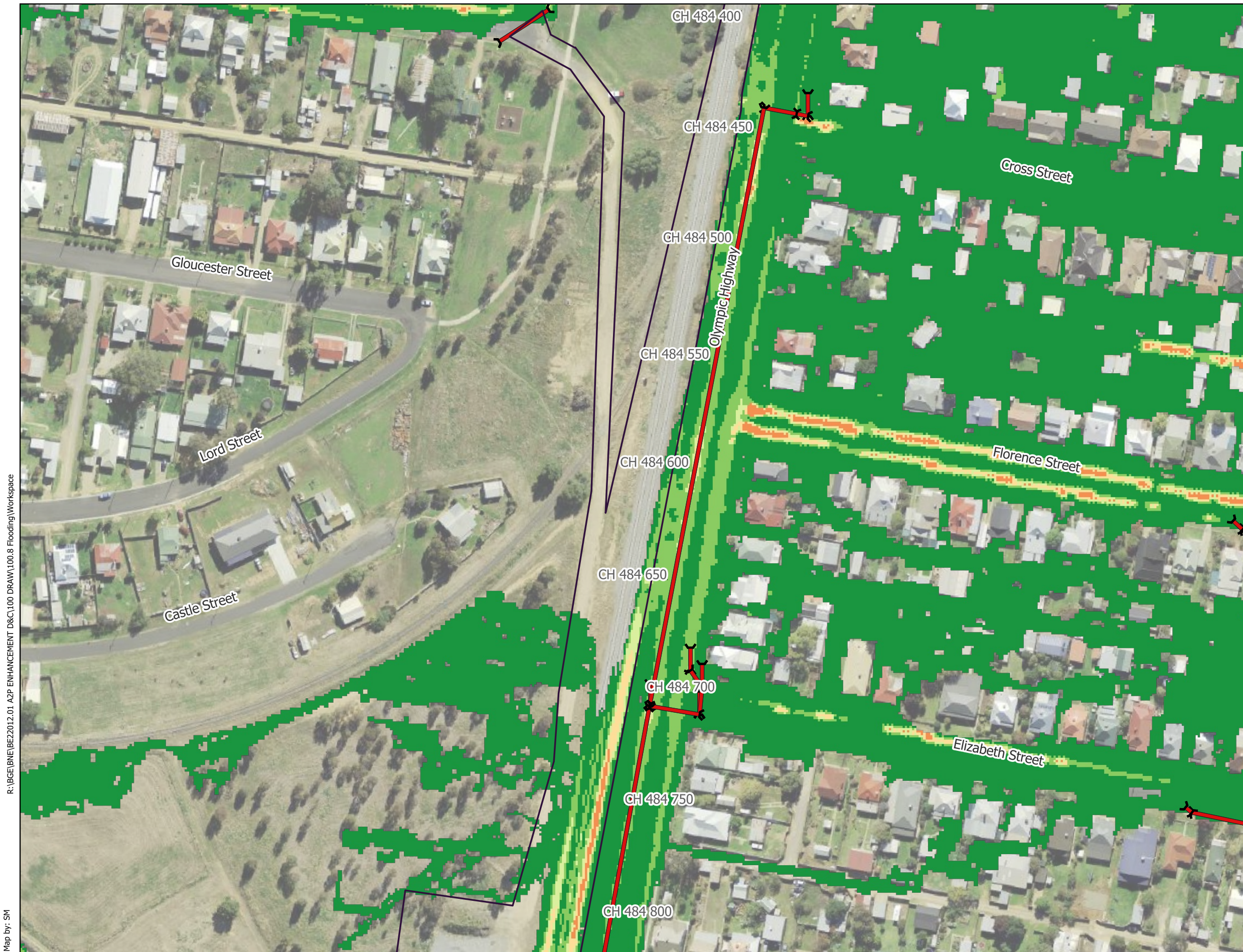
Figure 12b - Olympic Highway Underbridge - IFC Stage 5% AEP Flood Hazard (ARR2019) - Existing Conditions
