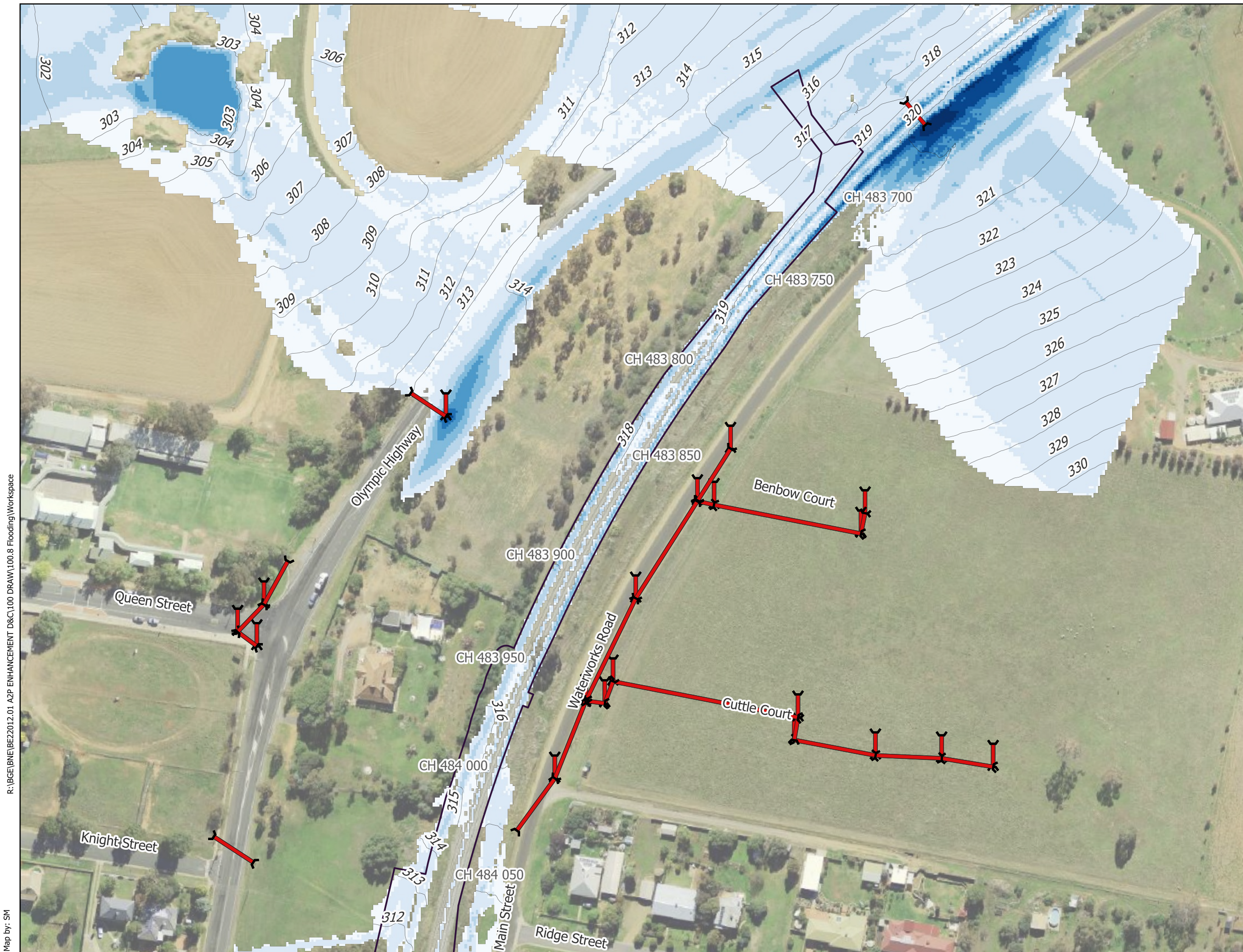
Figure 6d - Olympic Highway Underbridge - IFC Stage PMF Flood Depth (m) and Levels (m AHD) - Existing Conditions
