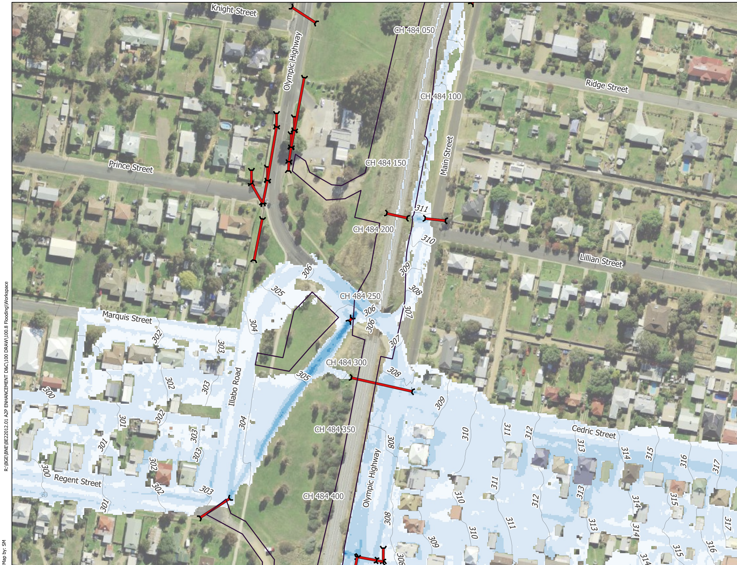
Figure 3c - Olympic Highway Underbridge - IFC Stage 2% AEP Flood Depth (m) and Levels (m AHD) - Existing Conditions
