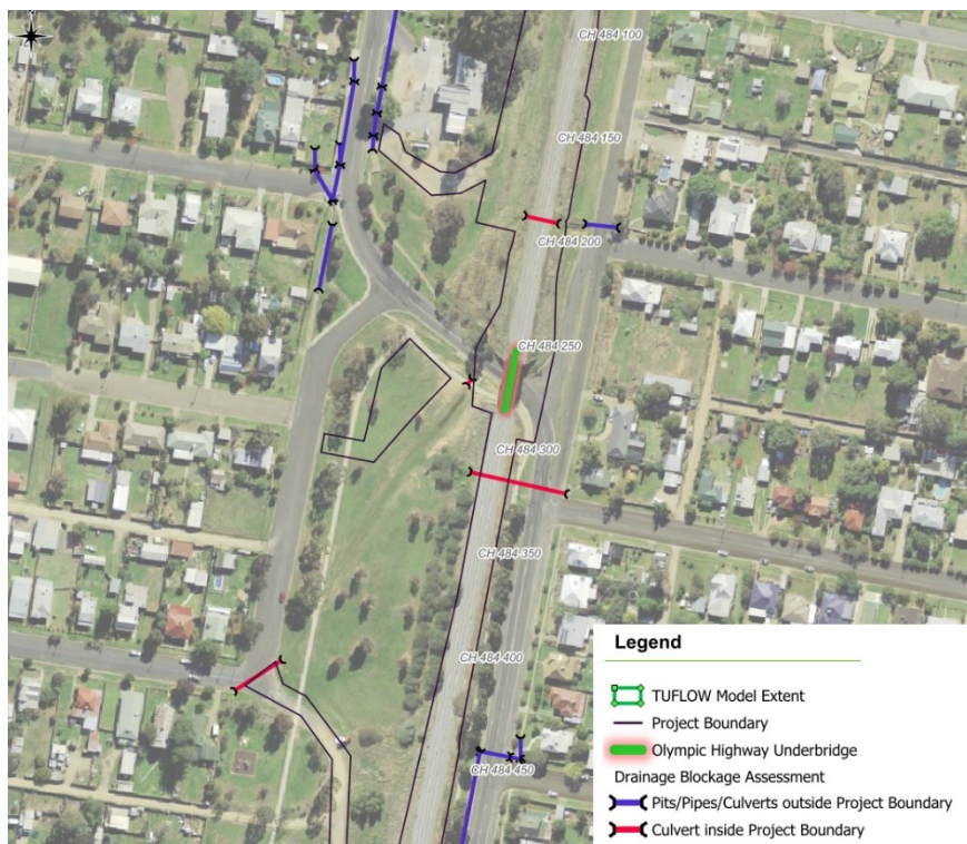
Figure 5-11: Culvert Blockage Setup
