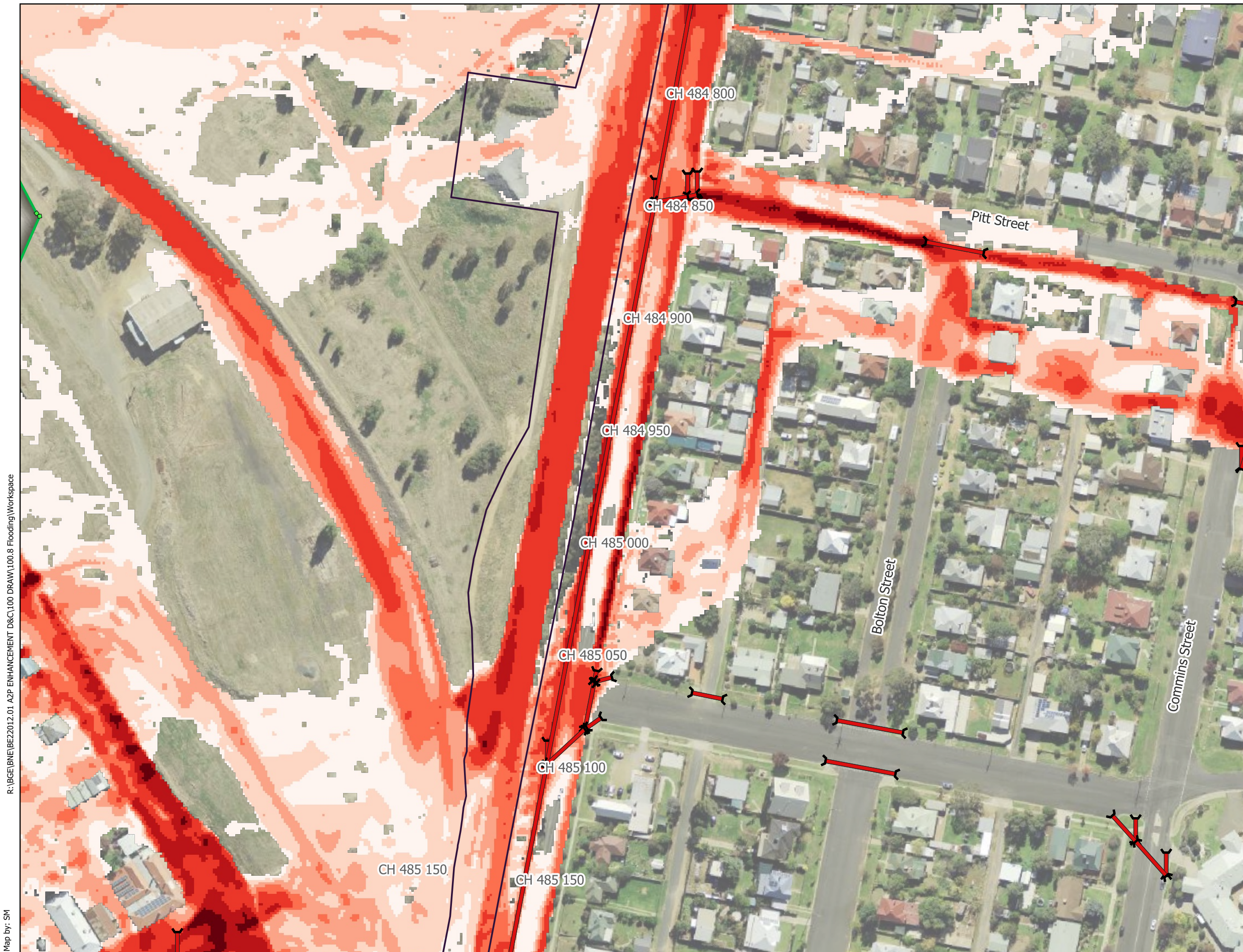
Figure 9a - Olympic Highway Underbridge - IFC Stage 1% AEP Flood Velocity (m/s) - Existing Conditions
