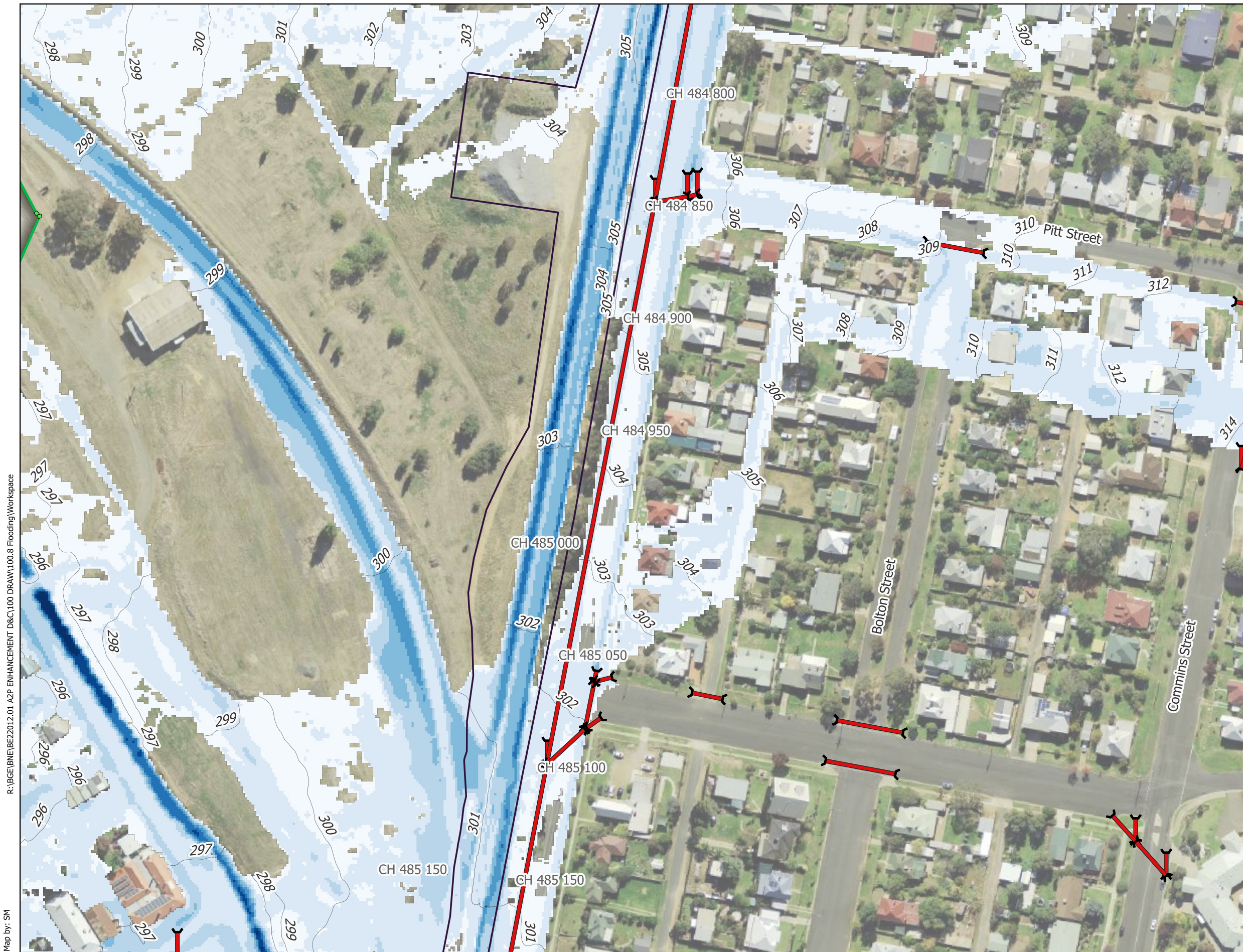
Figure 3a - Olympic Highway Underbridge - IFC Stage 2% AEP Flood Depth (m) and Levels (m AHD) - Existing Conditions
