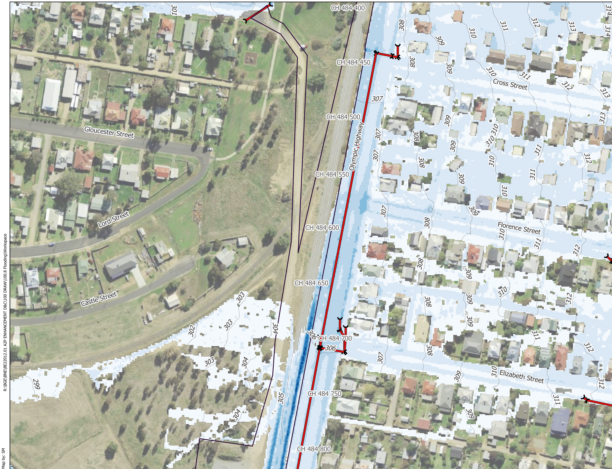
Figure 2b - Olympic Highway Underbridge - IFC Stage 5% AEP Flood Depth (m) and Levels (m AHD) - Existing Conditions
