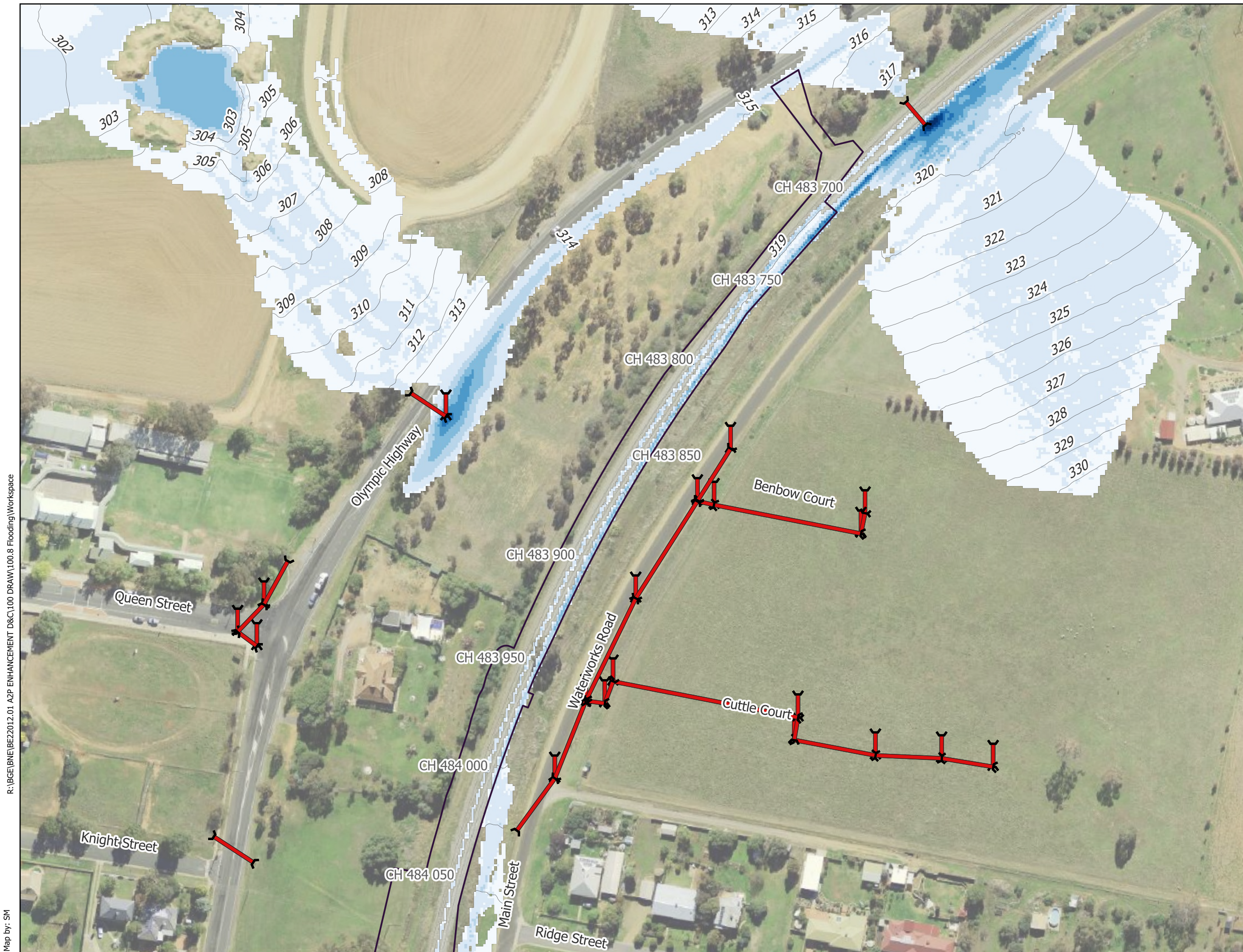
Figure 3d - Olympic Highway Underbridge - IFC Stage 2% AEP Flood Depth (m) and Levels (m AHD) - Existing Conditions
