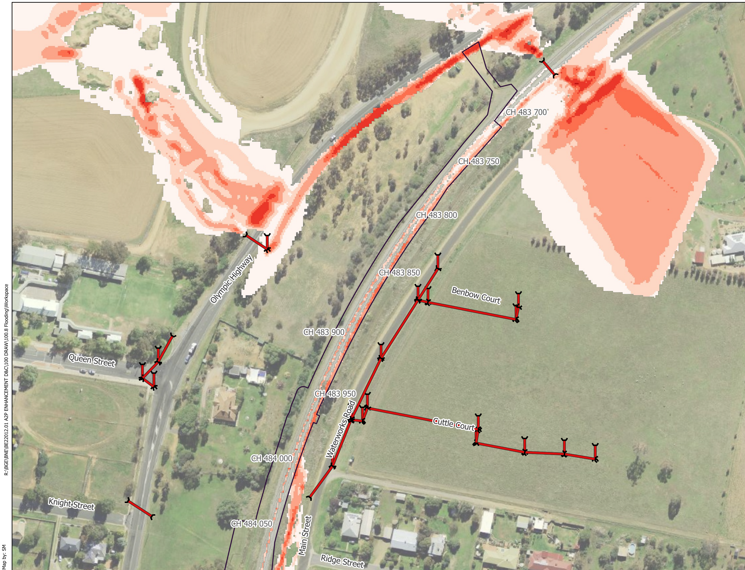
Figure 8d - Olympic Highway Underbridge - IFC Stage 2% AEP Flood Velocity (m/s) - Existing Conditions
