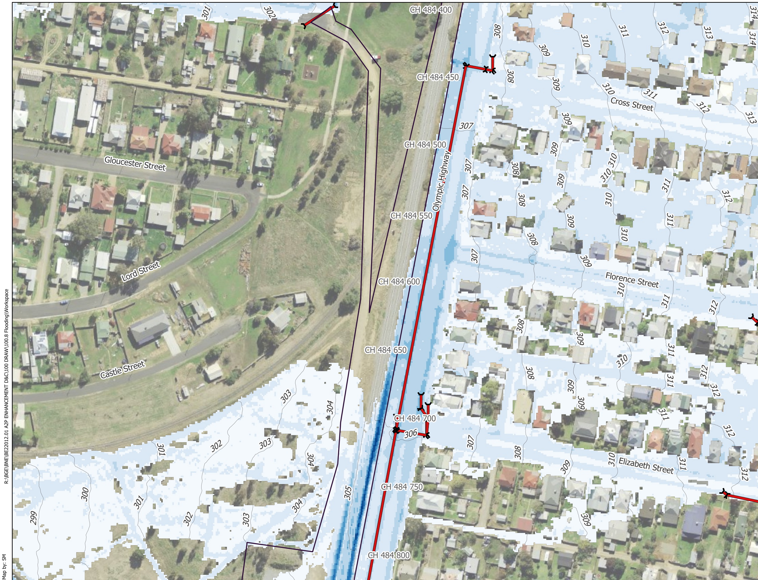
Figure 3b - Olympic Highway Underbridge - IFC Stage 2% AEP Flood Depth (m) and Levels (m AHD) - Existing Conditions
