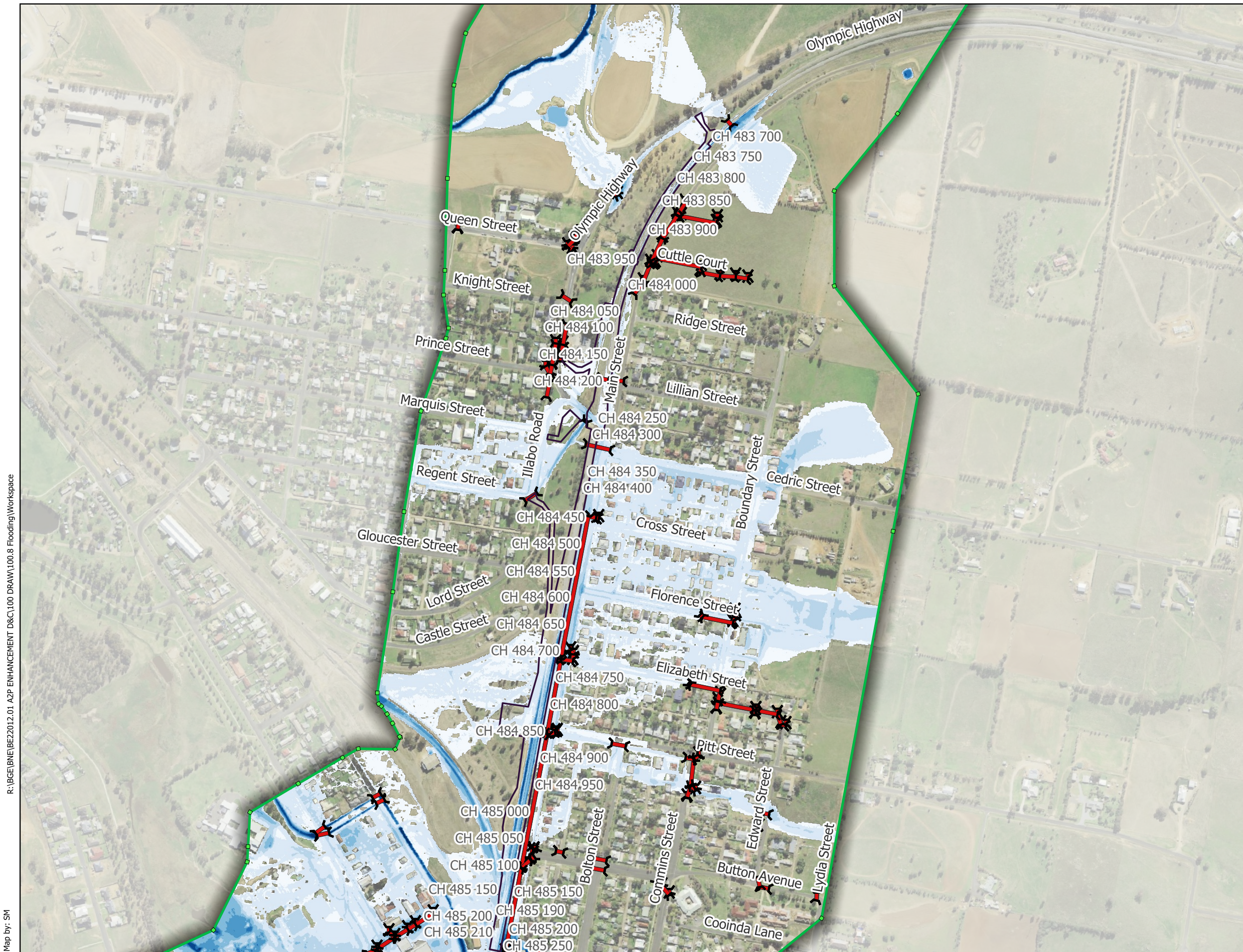
Figure 4 - Olympic Highway Underbridge - IFC Stage 1% AEP Flood Depth (m) and Levels (m AHD) - Existing Conditions
