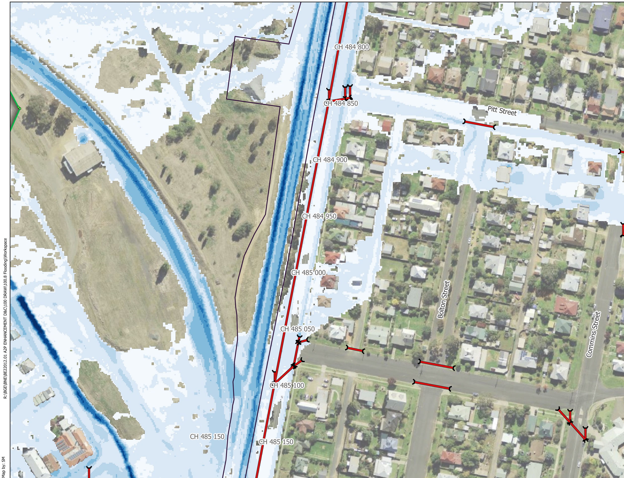
Figure 4a - Olympic Highway Underbridge - IFC Stage 1% AEP Flood Depth (m) and Levels (m AHD) - Existing Conditions
