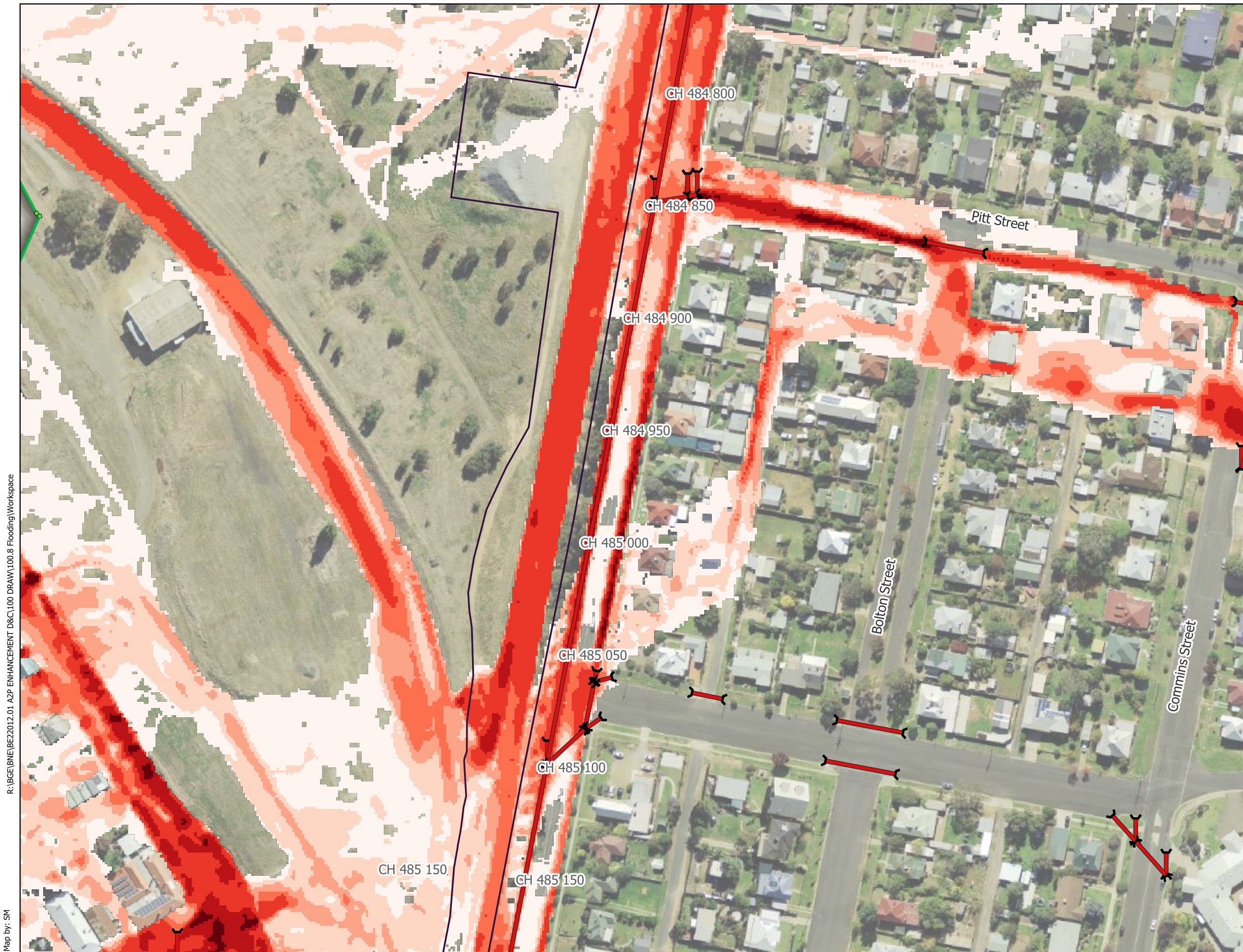
Figure 8a - Olympic Highway Underbridge - IFC Stage 2% AEP Flood Velocity (m/s) - Existing Conditions
