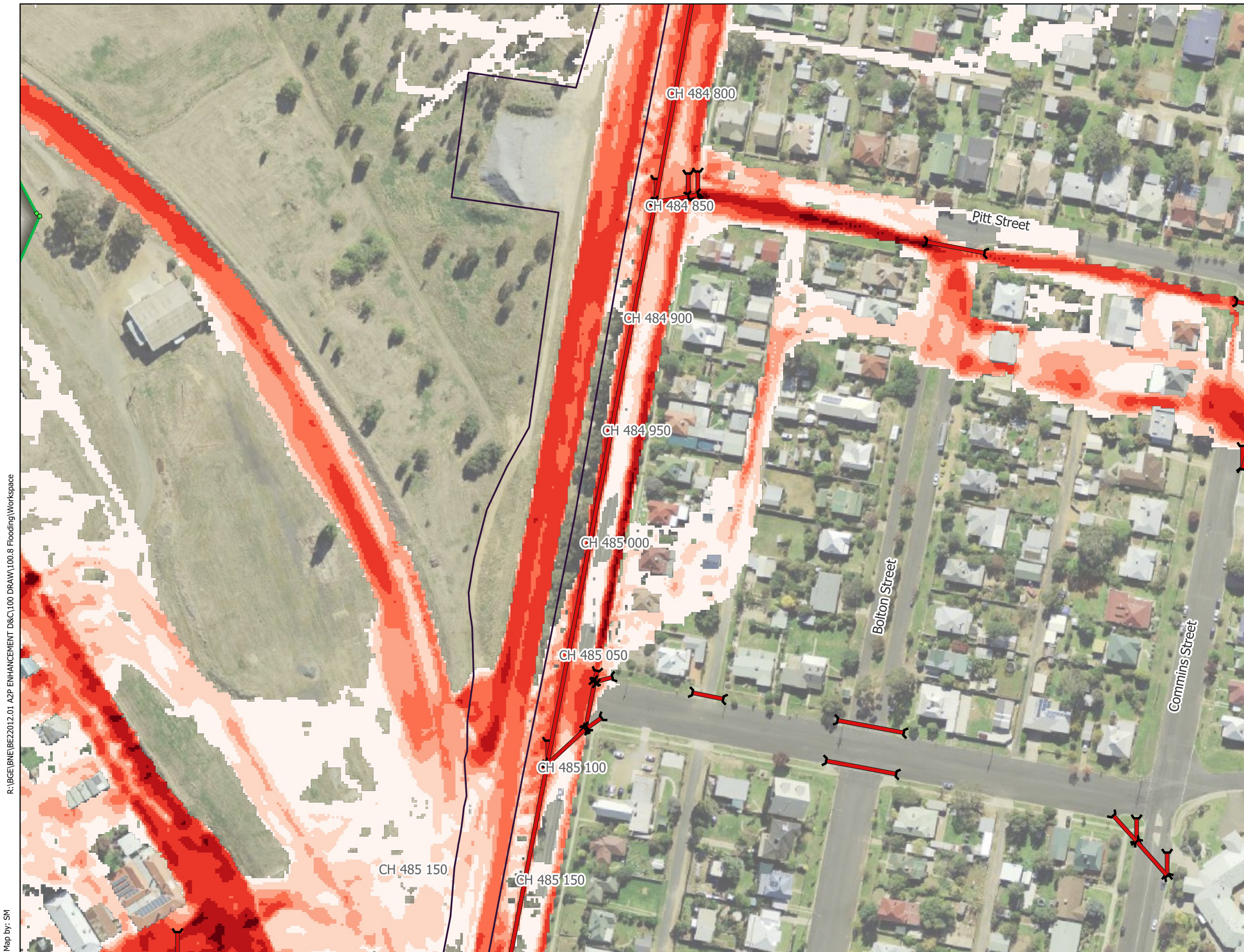
Figure 7a - Olympic Highway Underbridge - IFC Stage 5% AEP Flood Velocity (m/s) - Existing Conditions
