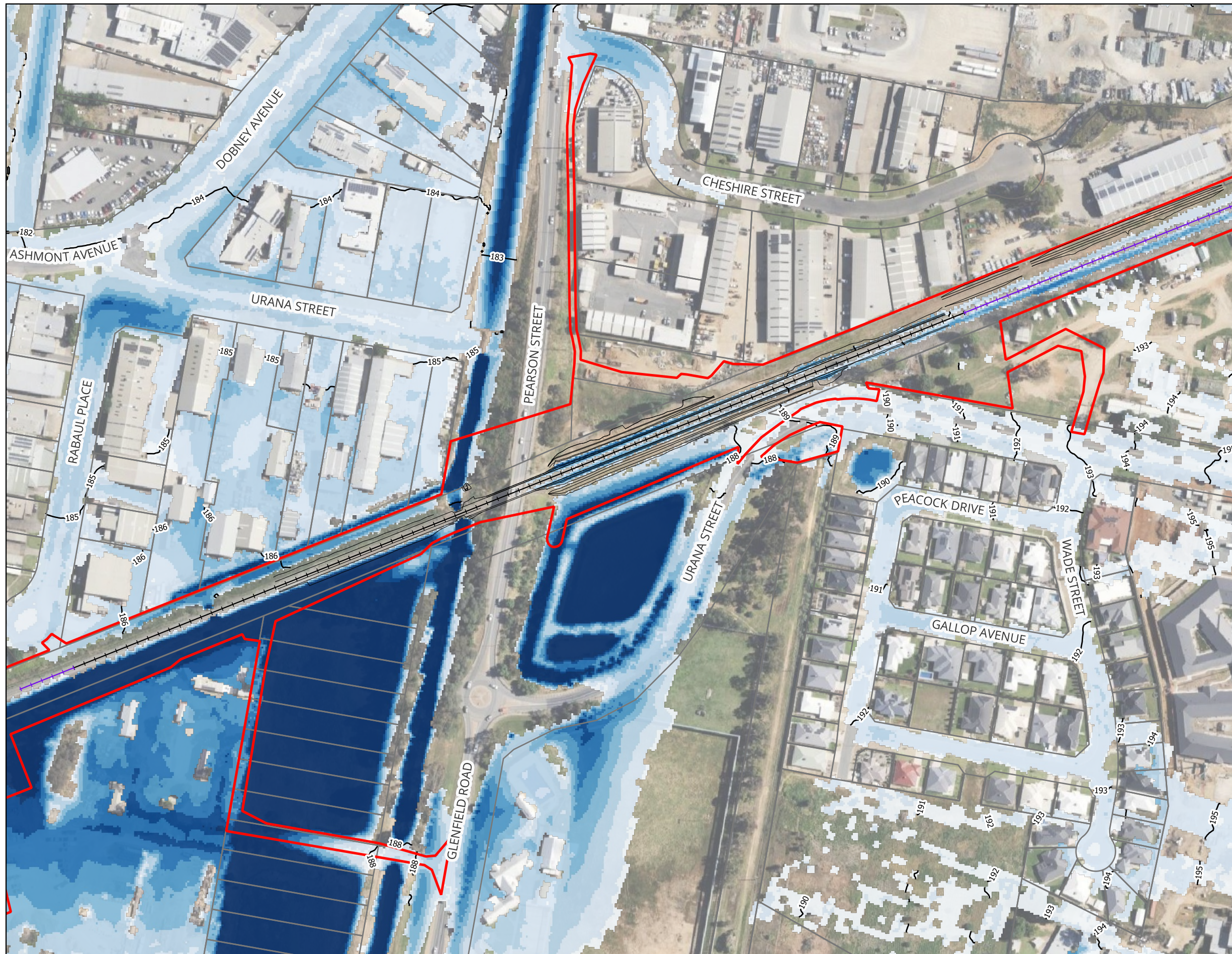
Figure A22 : 1% AEP Peak Flood Depth and Levels - Master Design Condition
