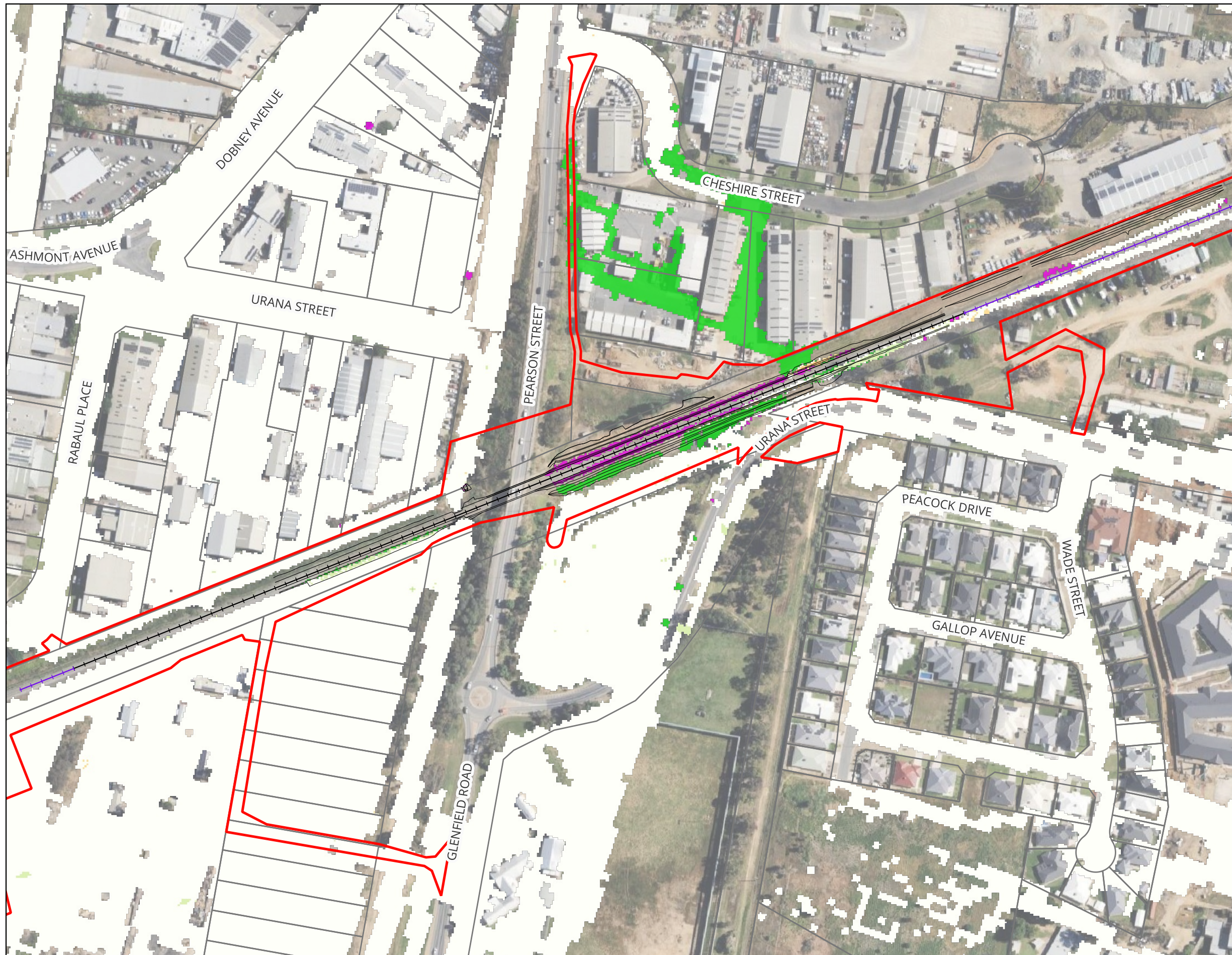
Figure A49 : Changes in Peak Flood Hazard for 2% AEP - Master Design Condition vs Existing Condition
