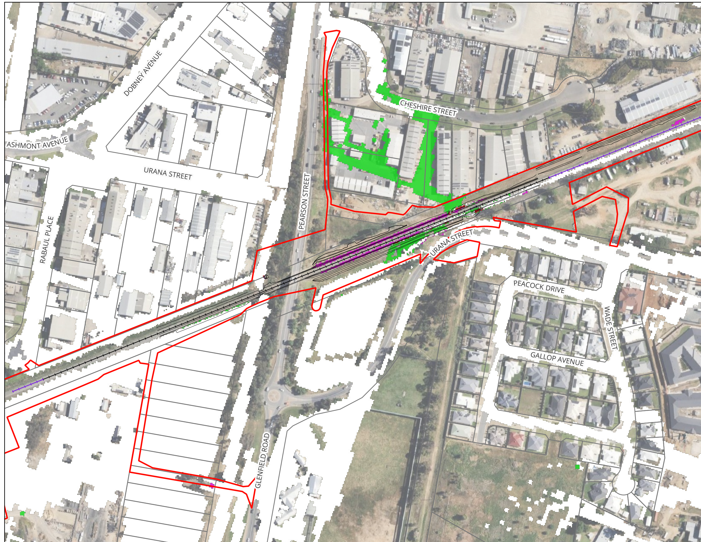
Figure A43 : Changes in Peak Flood Velocity for 5% AEP - Master Design Condition vs Existing Condition
