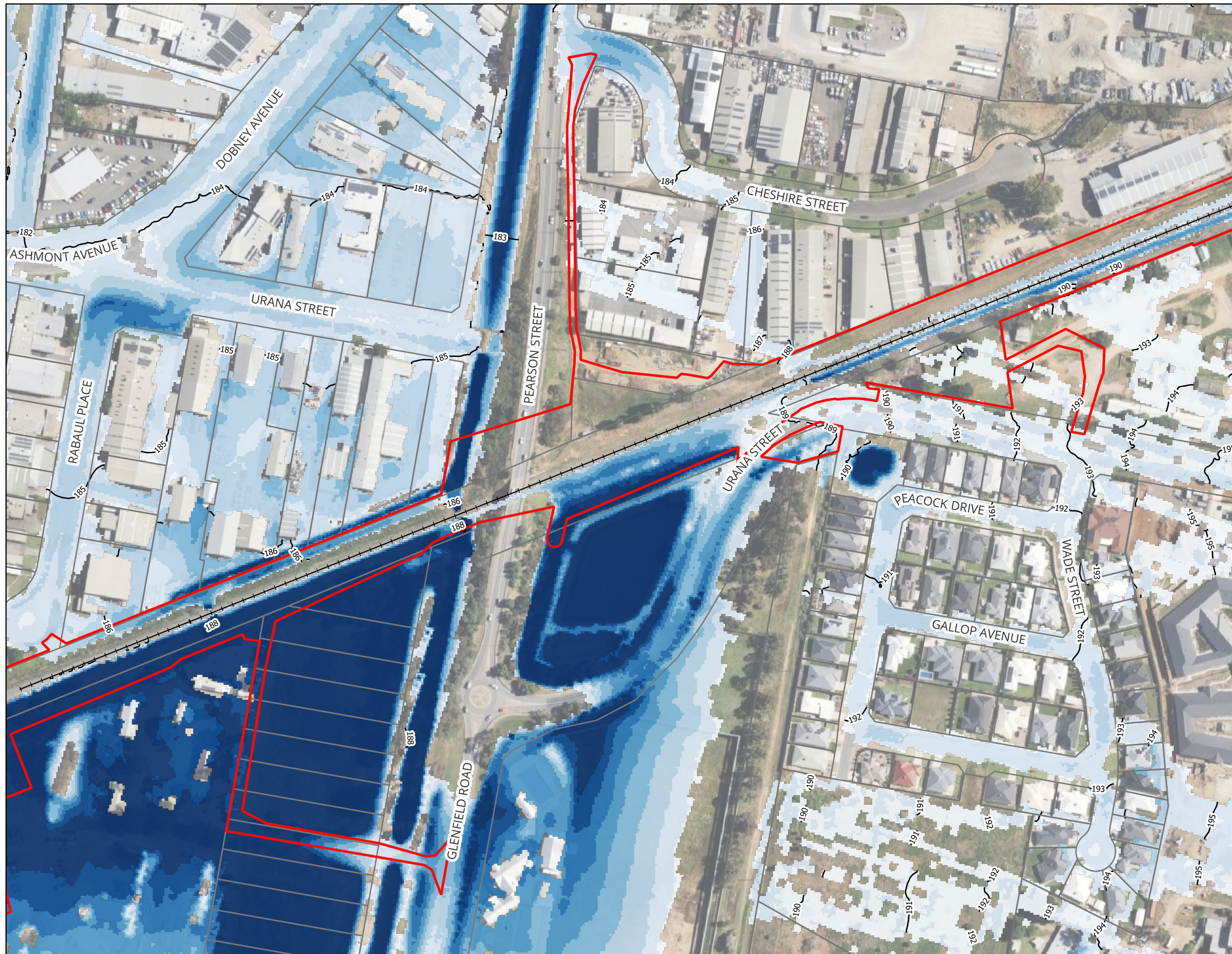
Figure A05 : 1% AEP Climate Changes Peak Flood Depth and Levels - Existing Condition
