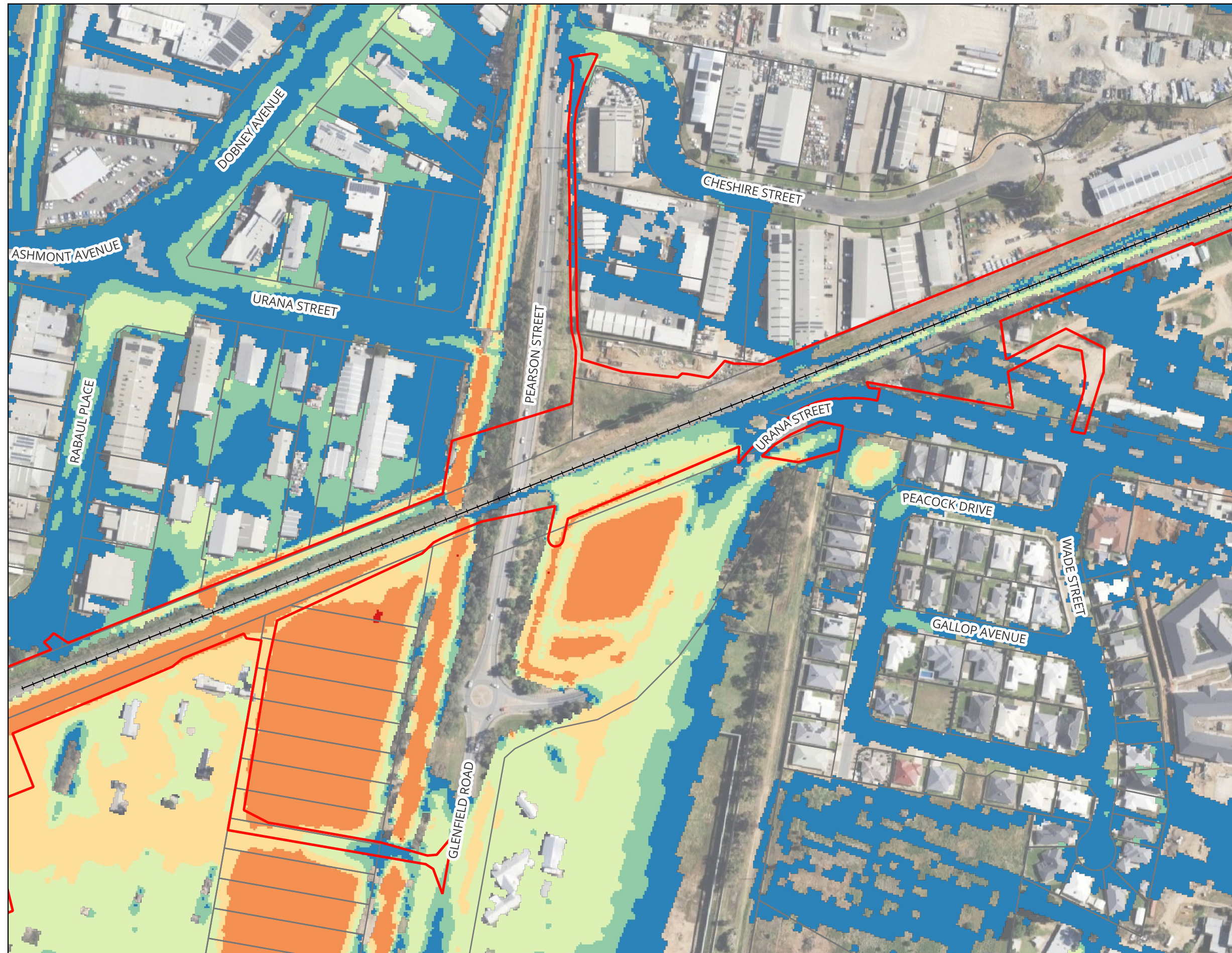
Figure A17 : 1% AEP Climate Changes Peak Flood Hazard - Existing Condition
