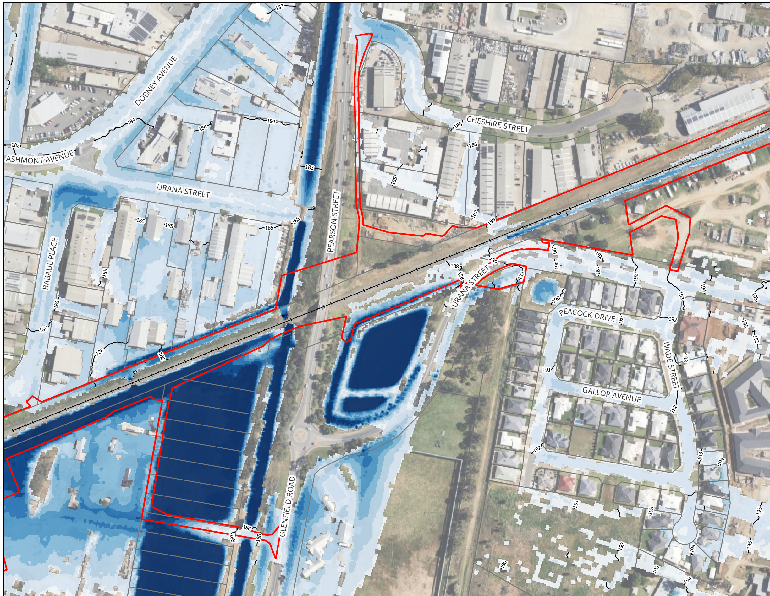
Pearson Street Bridge - Inland Rail (A2P) IFC Design - IFC Stage Figure A03 : 2% AEP Peak Flood Depth and Levels - Existing Condition
