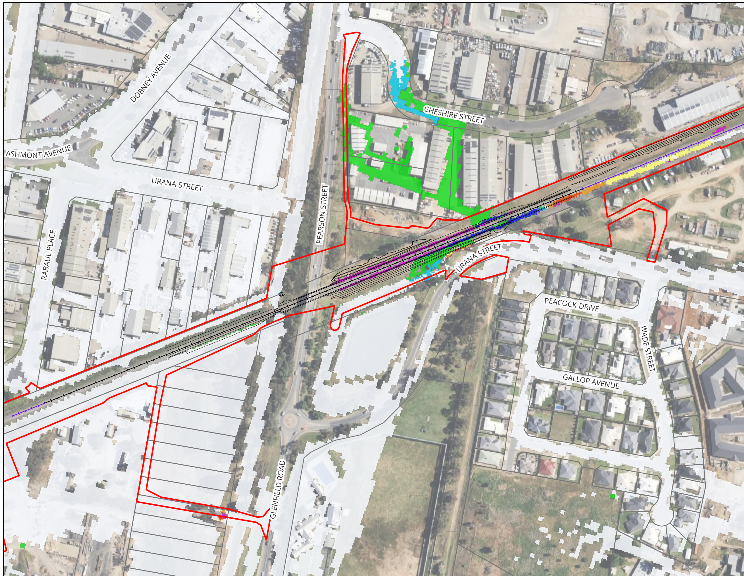
Figure A38 : Changes in Peak Flood Levels for 5% AEP - Master Design Condition vs Existing Condition
