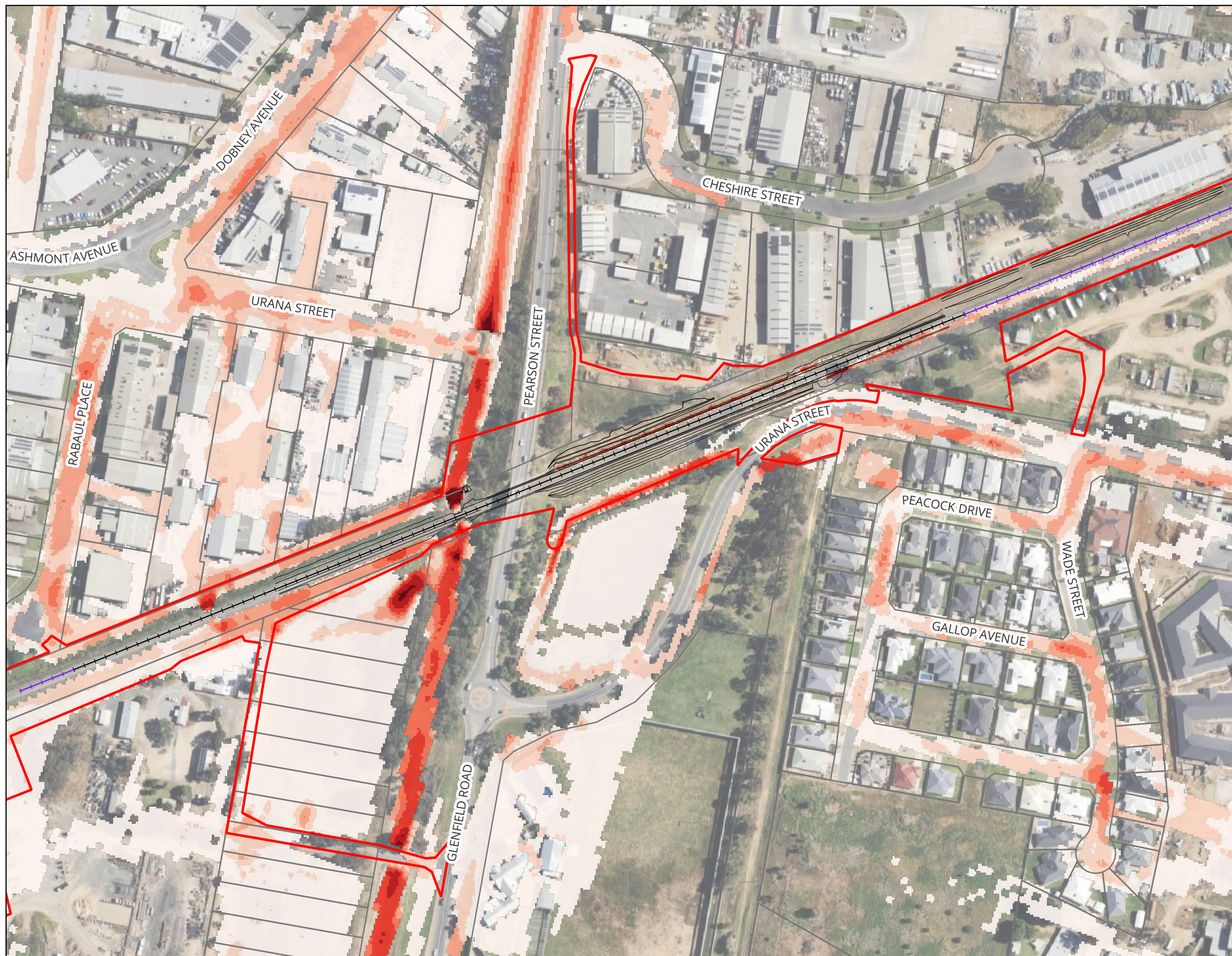
Pearson Street Bridge - Inland Rail (A2P) IFC Design - IFC Stage Figure A25 : 10% AEP Peak Flood Velocity - Master Design Condition
