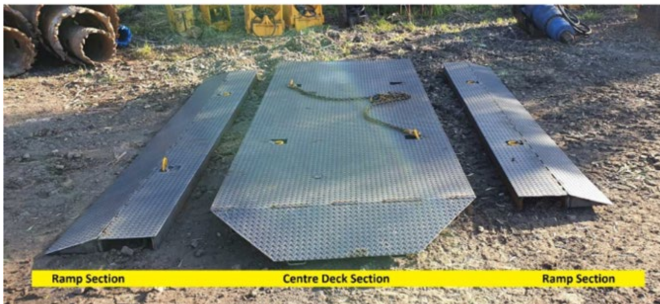
FIGURE 25: RAPIDLY DEPLOYABLE TEMPORARY RAILWAY RAMP
